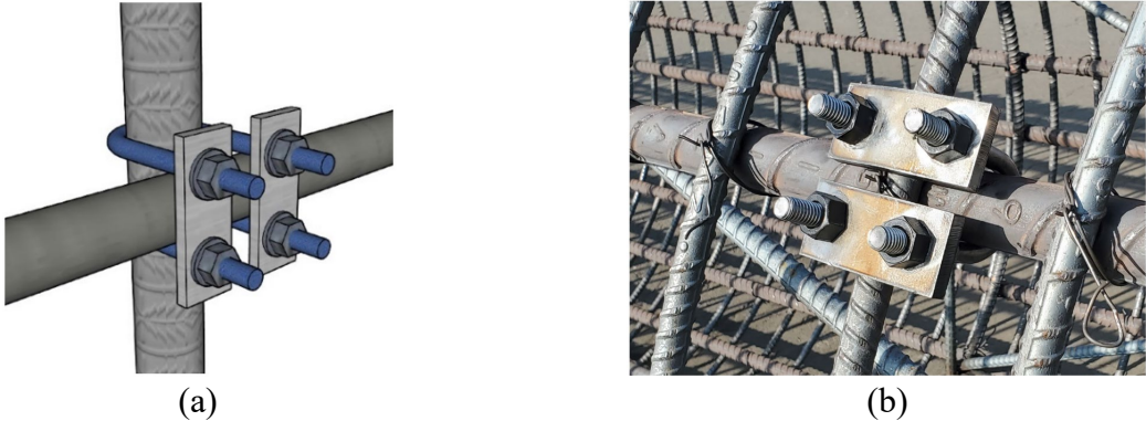
Fig. 3. (a) Schematic view of U-bolt connector, (b) an assembled U-bolt connection on a cross-bar connection in a rebar cage.
