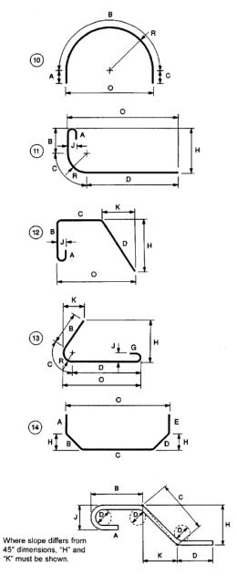
**ENLARGED VIEW SHOWING BAR BENDING DETAILS**
