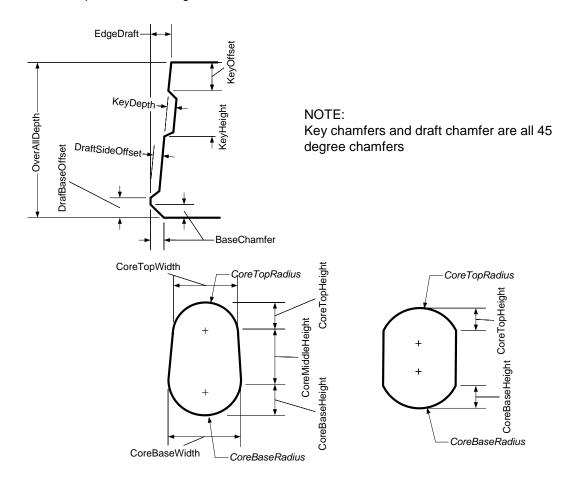
NOTE: The CoreTopRadius and CoreBaseRadius parameters can be derived and are therefore not listed in the IfcHollowCoreShapeProfileDef definition. They are shown to define that the curves are arcs. The parameters for the center core are the same as above, but with the prefix "Center".
