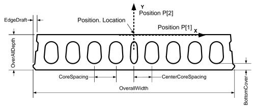
NOTE: In all cases, the cores are symmetrically distributed on either side of the plank center line, irrespective of whether the number of cores is odd or even. For planks with a center core with different geometry to that of the other cores, set CenterCoreSpacing > 0. When the number of cores is even, all Center Core parameters are ignored.
