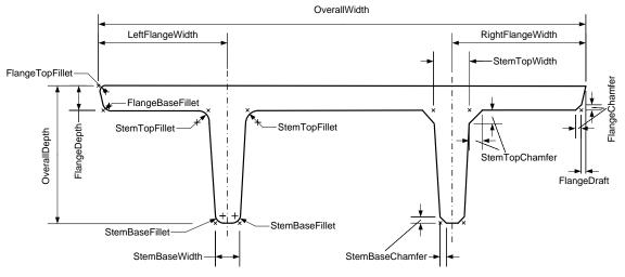
NOTE: The left and right stems show alternate configurations; either can have chamfers or fillets at top or base. Where the values of Fillet parameters are grater than zero, Chamfer values will be ignored.
