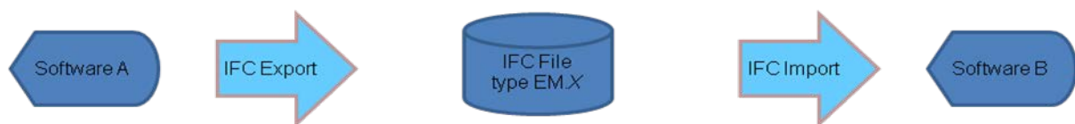
Fig. 4: Exchanging a model from one BIM software application to another.
