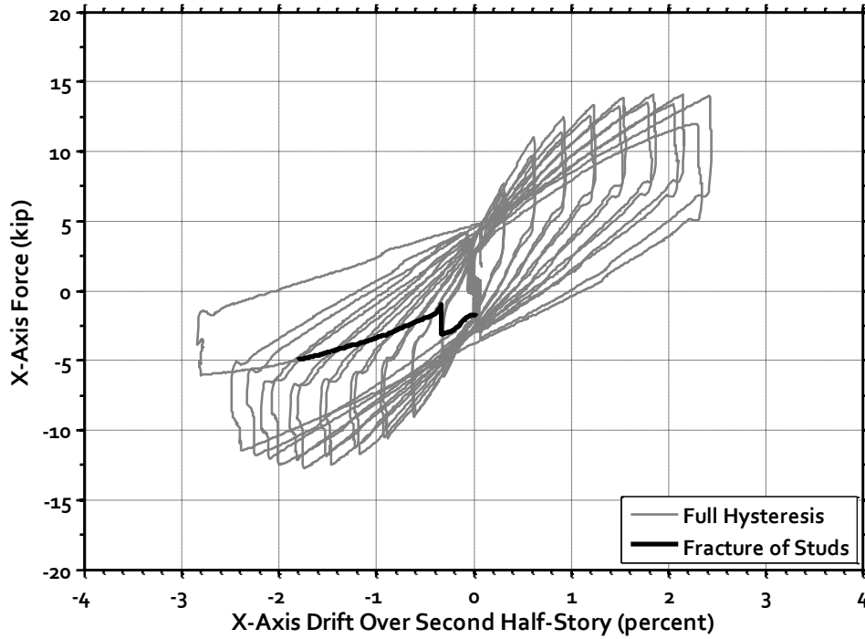
Figure C-6: Specimen B2 – Load versus Second Half-Story Drift in X-Direction
