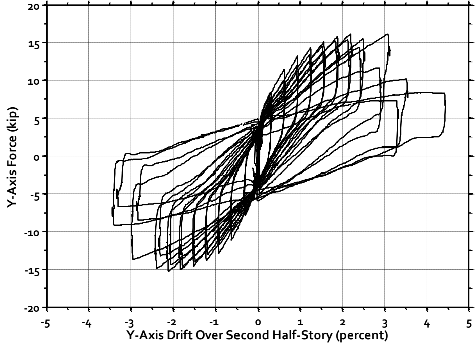
Figure C-16: Specimen B4 – Load versus Second Half-Story Drift in Y-Direction
