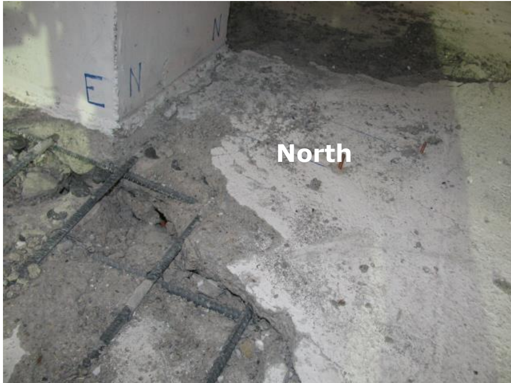
Figure 3-14: Specimen B1 – Sound Concrete on North Face of Connection After Test
