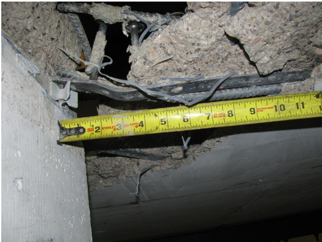
Figure 3-19: Specimen B3 – Bending of Base Rail between First and Second Shear Stud
