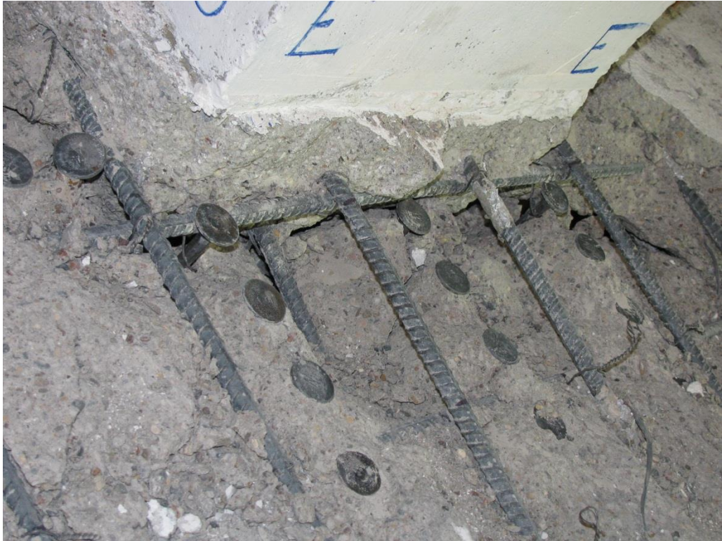
Figure 3-13: Specimen B1 – Void in Connection Region on East and South Faces of Connection After Test
