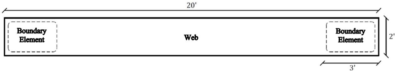
**Figure 6 - Wall Cross-Section**
