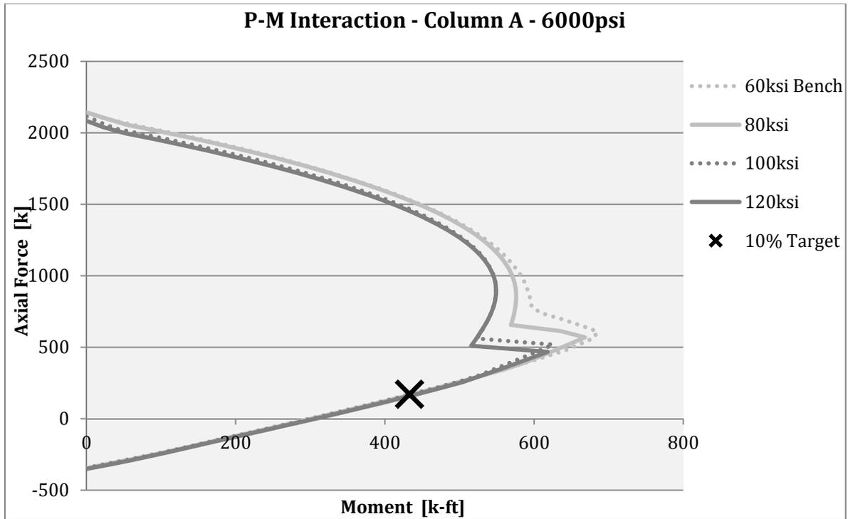
Figure 12- P-M Interaction Curves for Column A (Fig. 5) with  $f'_c = 6,000$  psi and Varying  $f_y$ . All designs have the same flexural strength at axial load ratio of 10%.
