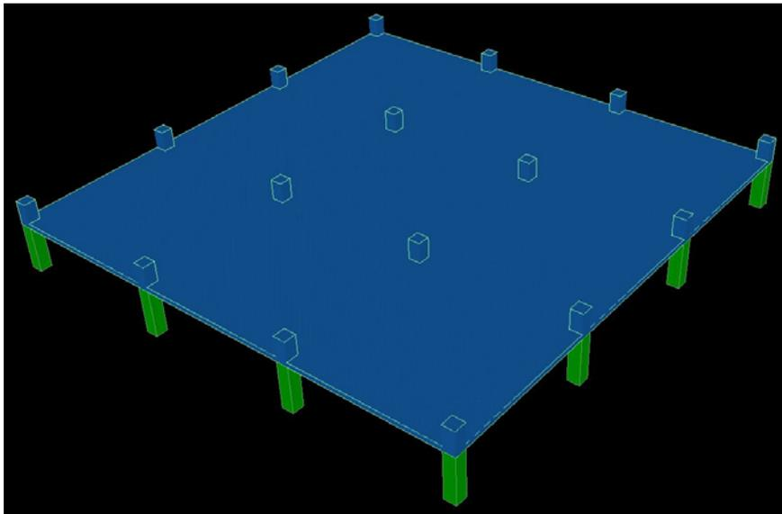
**Figure 2 – Two-Way System Configuration**
