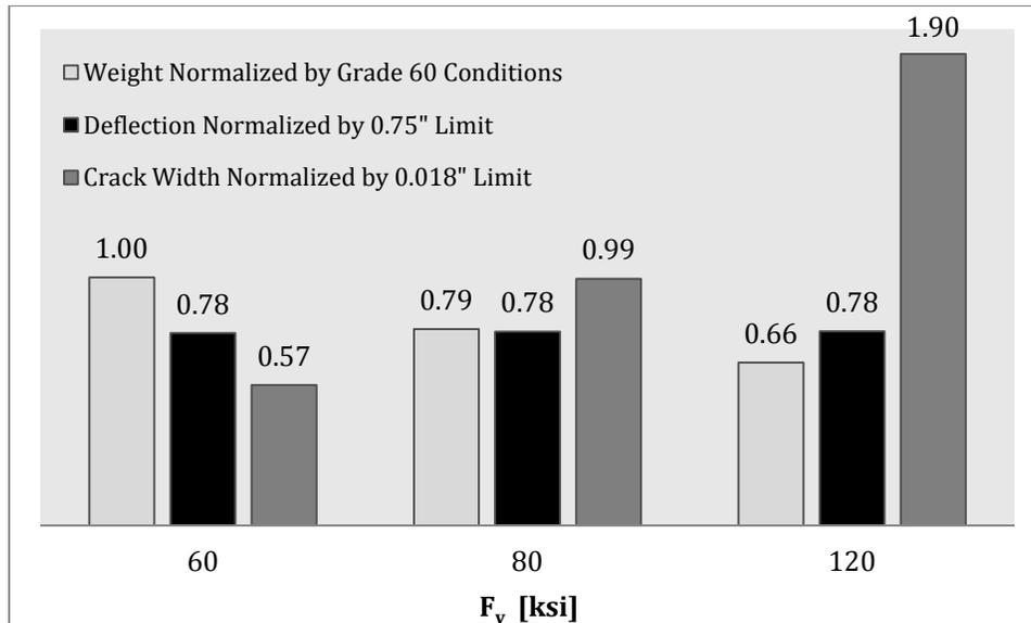
**Figure 9 – One-Way Slab Example – 27 ft. Span Length, 10 in. Slab Thickness**
