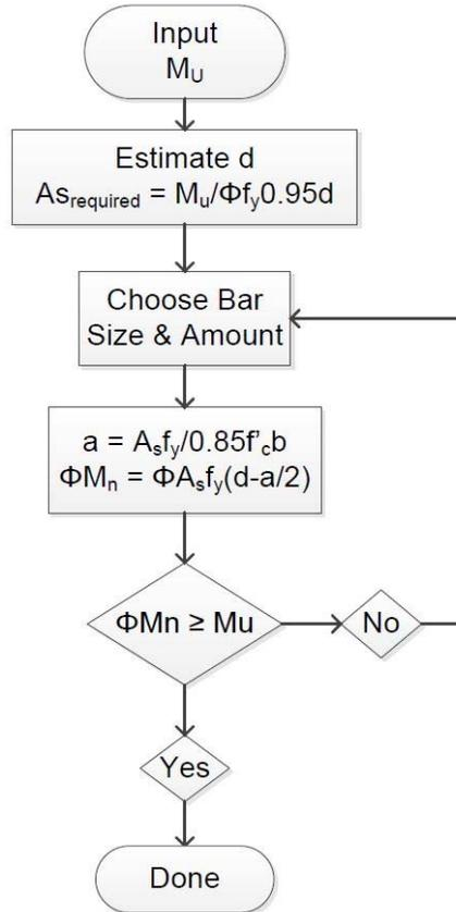
**Figure 7 - Flexural Design Flow**
