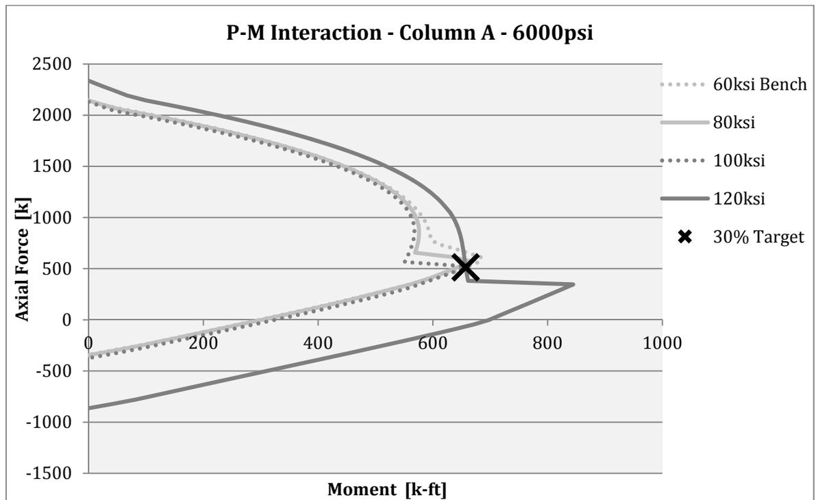
Figure 13 - P-M Interaction Curves for Column A (Fig. 5) with  $f'_c = 6,000$  psi and Varying  $f_y$ . All designs have the same flexural strength at axial load ratio of 30%.
