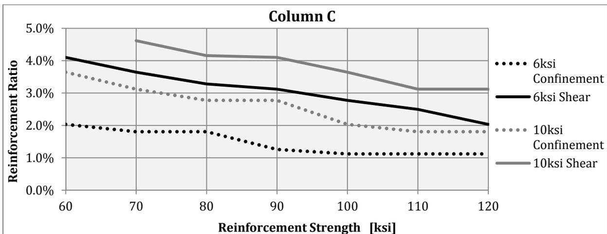
**Figure 16 – Transverse Reinforcement Ratios versus Steel Strength for Different Column Geometries**
