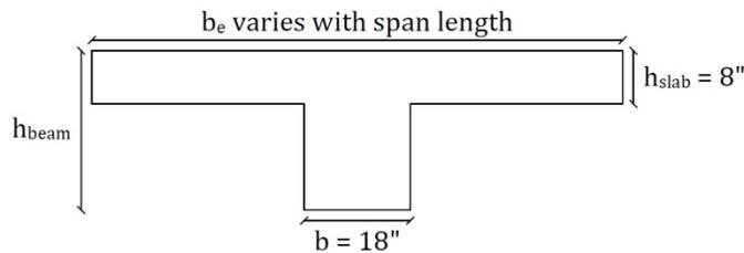
**Figure 4 – Beam Cross-Section**
