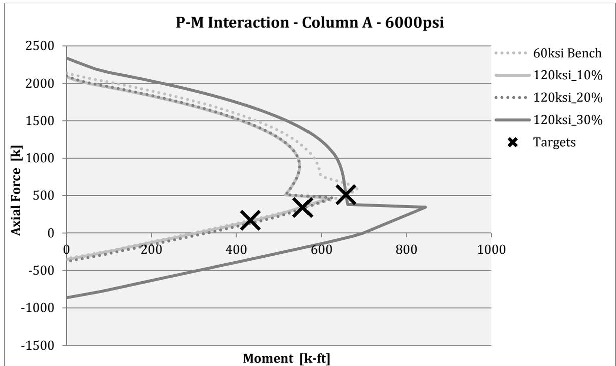
**Figure 14 - P-M Interaction Curves for Column A (Fig. 5) with  $f'_c = 6,000$  psi and  $f_y = 120$  ksi. Designs have the same flexural strength as the 60 ksi reference design for axial load ratios of 10%, 20% and 30%.**
