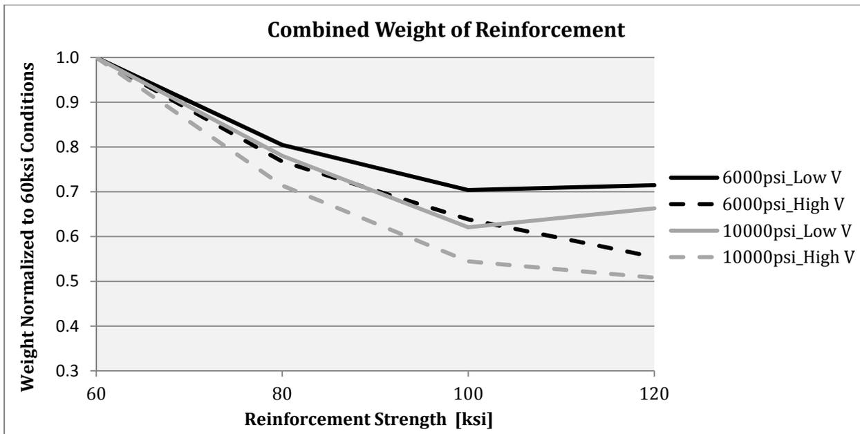
**Figure 17 – Normalized Weight of Longitudinal, Confining, and Shear Reinforcement for Structural Walls with the Same Flexural Strength and Different Concrete Strengths and Shear Demands**
