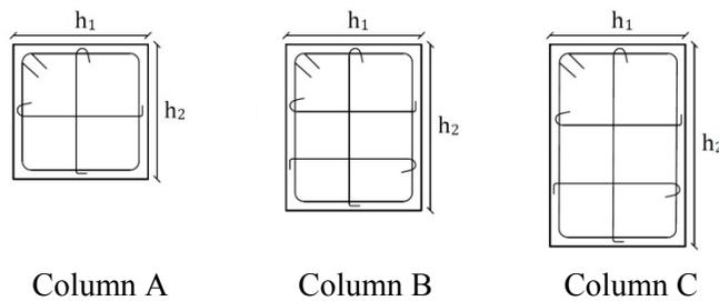
**Figure 5 - Column Cross Sections**
