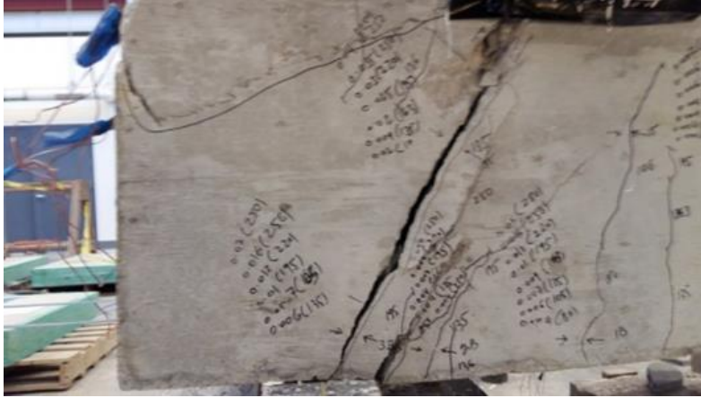
Figure 4.4 Specimen NH-3-8-5-13-F4.1-II after failure
