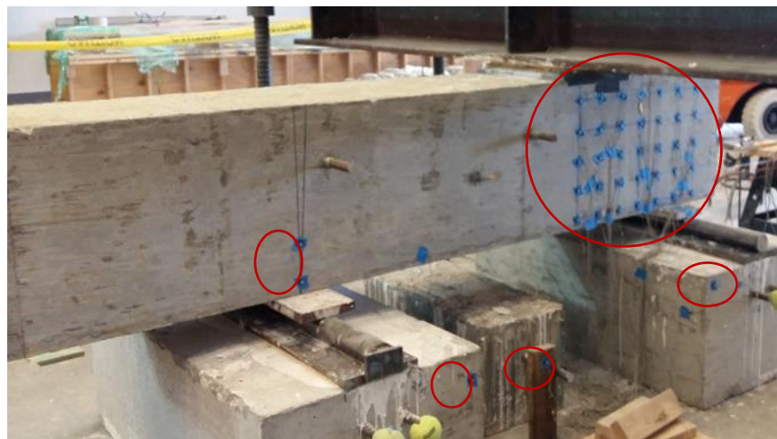
Figure 2.25 Placement of markers for a typical specimen
