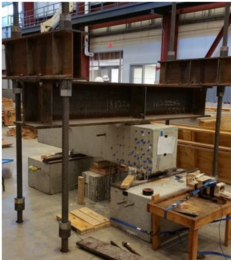
Figure 2.18 A typical CCT node test
