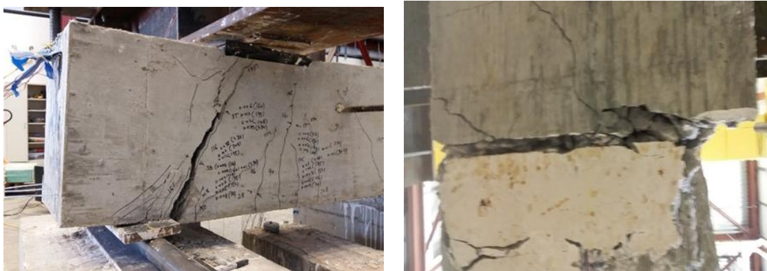
a. Side view b. Bottom of the specimen Figure 4.7 Pullout failure – Specimen H-3-8-5-11-F4.1-II
