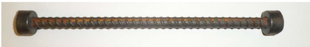
Figure 1.7: Headed deformed bar for use as shear reinforcement
