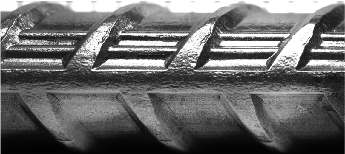
Figure 2-4: Front view of longitudinal geometry for M1-B2-100-#8
