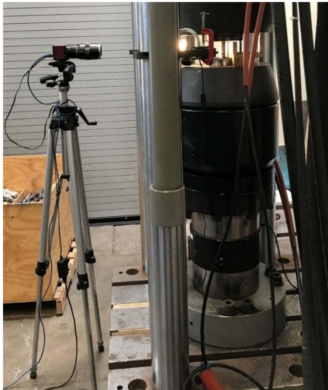
FIGURE 2-7: SIDE VIEW OF EXPERIMENTAL SETUP SHOWING TEST FRAME AND DIC CAMERA
