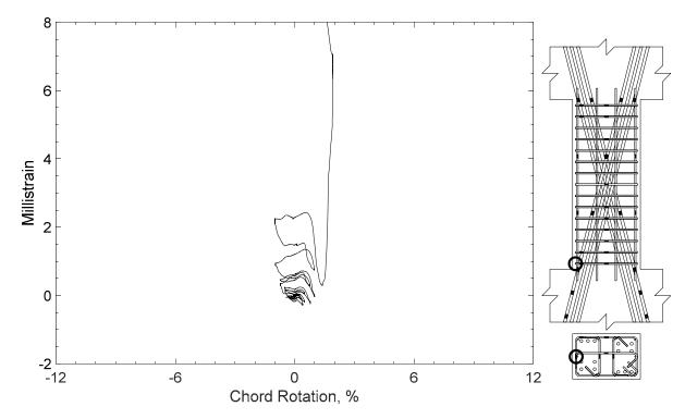
Figure 217 – Measured strain in closed stirrup of D80-2.5, strain gauge S3
