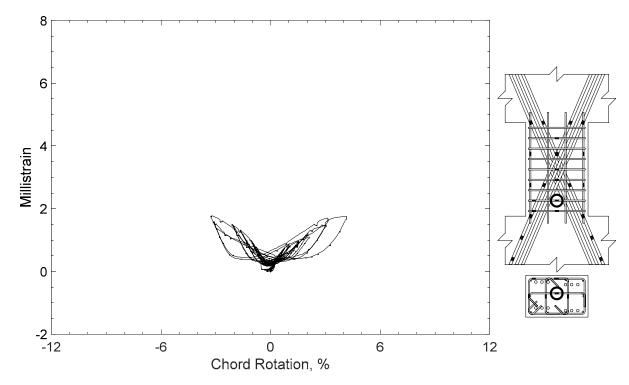
Figure 197 – Measured strain in crosstie of D120-1.5, strain gauge T3
