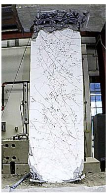
Figure C.92 – D120-3.5 at +8% chord rotation, second cycle
