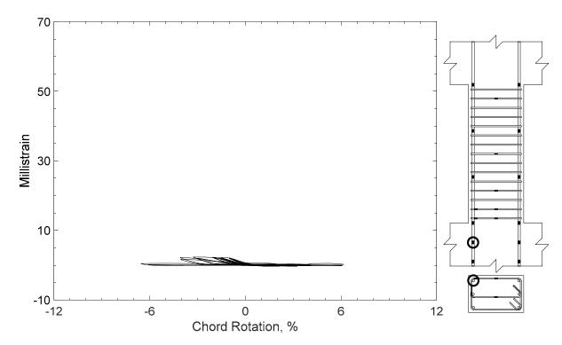
Figure 427 – Measured strain in parallel bar of P100-2.5, strain gauge P3
