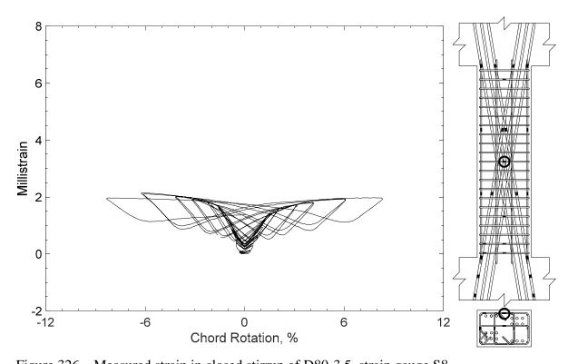
Figure 326 – Measured strain in closed stirrup of D80-3.5, strain gauge S8
