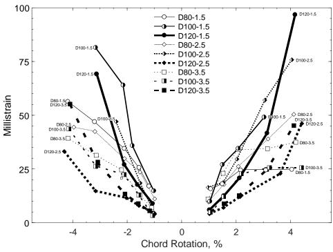
Figure 504 – Maximum strains in D-type beams during loading steps 5 through 9 (1% through 4% chord rotation), D strain gauges
