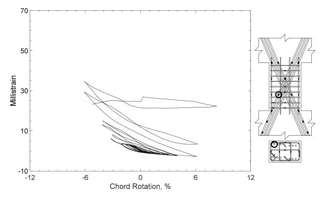
Figure 89 – Measured strain in diagonal bar of D80-1.5, strain gauge D7
