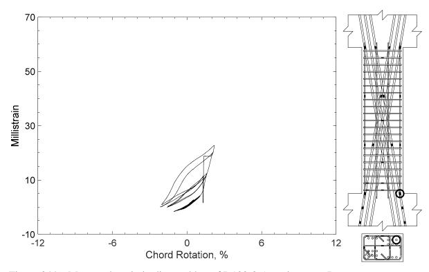
Figure 344 – Measured strain in diagonal bar of D100-3.5, strain gauge D6
