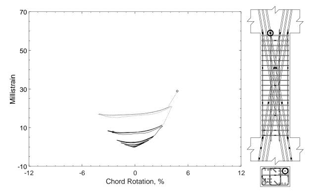
Figure 382 – Measured strain in diagonal bar of D120-3.5, strain gauge D11
