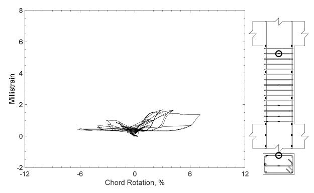
Figure 423 – Measured strain in closed stirrup of P80-2.5, strain gauge S9
