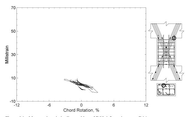
Figure 96 – Measured strain in diagonal bar of D80-1.5, strain gauge D14
