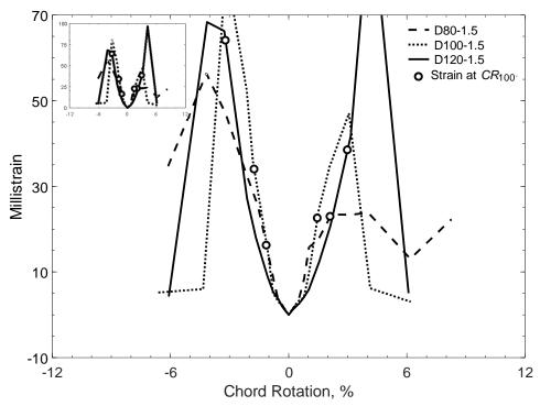
Figure 489 – Envelopes of measured strains in diagonal bars of D-type beams with an aspect ratio of 1.5, D strain gauges
