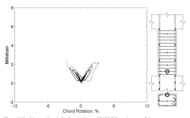
Figure 440 – Measured strain in closed stirrup of P100-2.5, strain gauge S4
