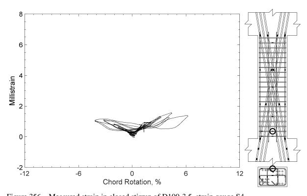
Figure 356 – Measured strain in closed stirrup of D100-3.5, strain gauge S4
