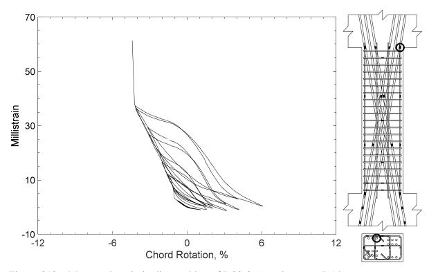
Figure 318 – Measured strain in diagonal bar of D80-3.5, strain gauge D14
