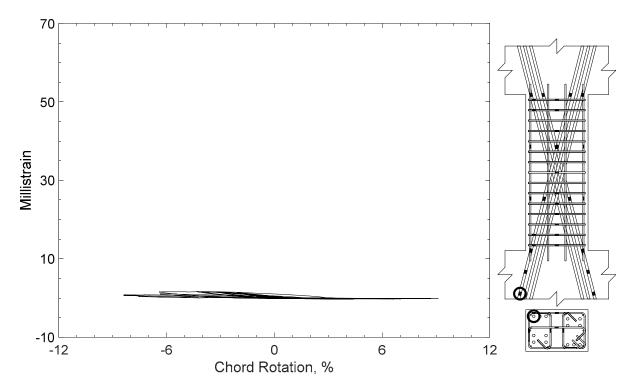
Figure 264 – Measured strain in diagonal bar of D120-2.5, strain gauge D1
