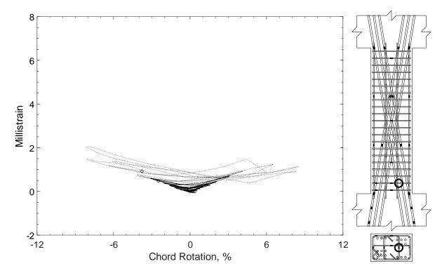
Figure 400 - Measured strain in crosstie of D120-3.5, strain gauge T1
