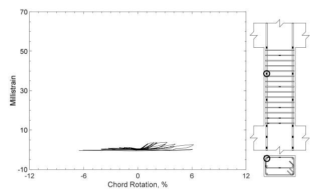
Figure 433 – Measured strain in parallel bar of P100-2.5, strain gauge P9
