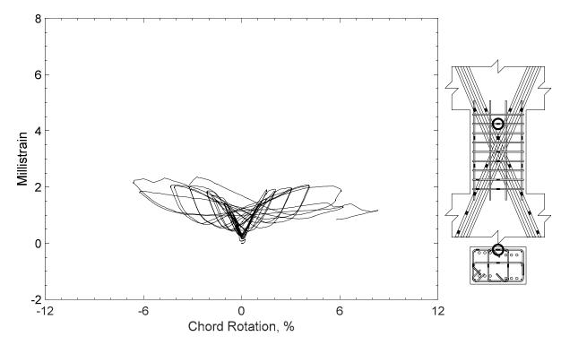
Figure 143 – Measured strain in closed stirrup of D100-1.5, strain gauge S9
