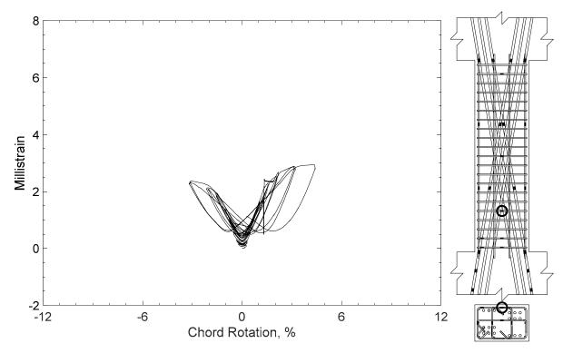
Figure 359 – Measured strain in closed stirrup of D100-3.5, strain gauge S7
