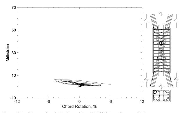
Figure 241 – Measured strain in diagonal bar of D100-2.5, strain gauge D10
