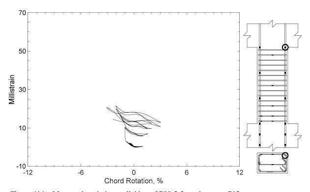
Figure 414 – Measured strain in parallel bar of P80-2.5, strain gauge P12
