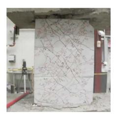
Figure C.15 – D100-1.5 at +4% chord rotation, second cycle
