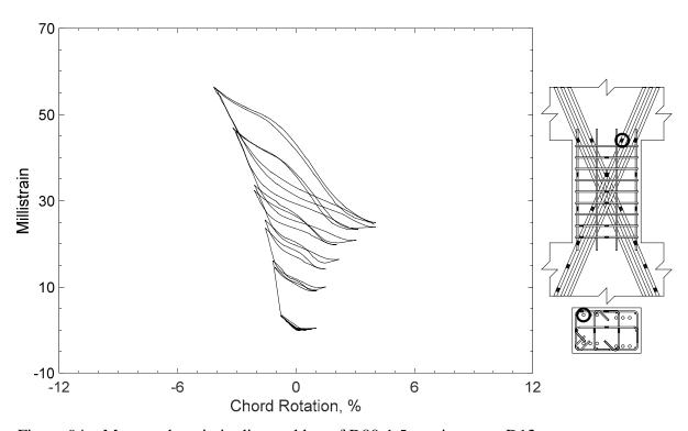
Figure 94 – Measured strain in diagonal bar of D80-1.5, strain gauge D12
