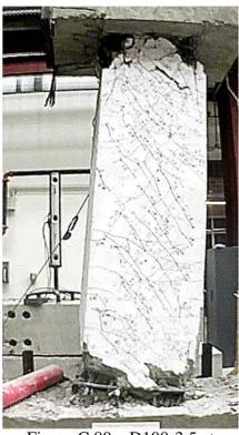
Figure C.80 – D100-3.5 at +8% chord rotation, second cycle
