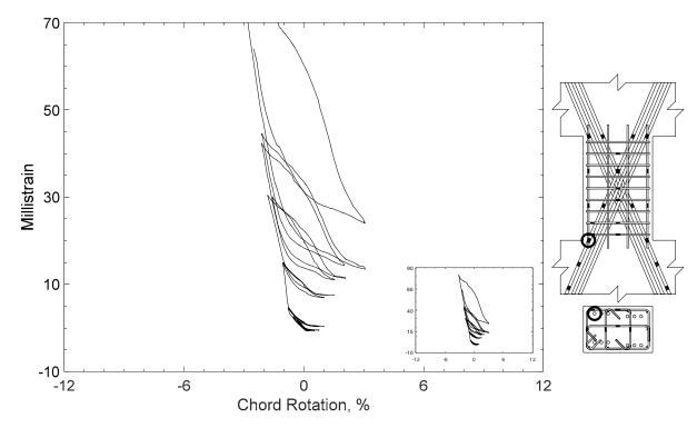
Figure 125 – Measured strain in diagonal bar of D100-1.5, strain gauge D5
