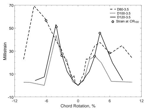
Figure 497 – Envelopes of measured strains in diagonal bars of D-type beams with an aspect ratio of 3.5, D strain gauges
