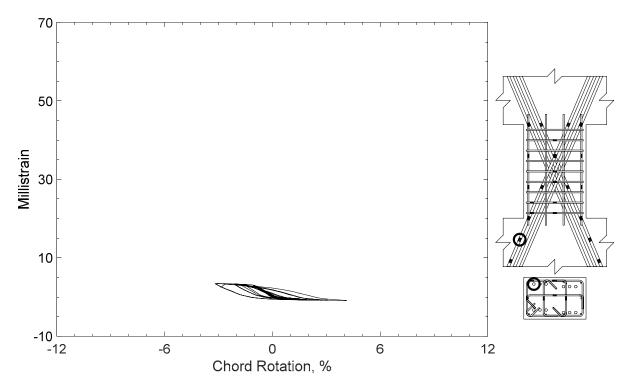
Figure 123 – Measured strain in diagonal bar of D100-1.5, strain gauge D3
