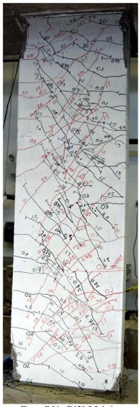
Figure C.84 – D120-3.5 during second cycle to 2% chord rotation
