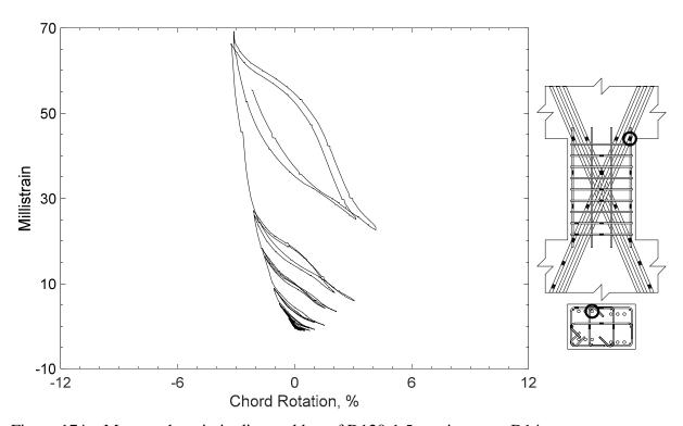
Figure 174 – Measured strain in diagonal bar of D120-1.5, strain gauge D14
