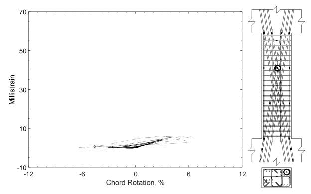
Figure 380 – Measured strain in diagonal bar of D120-3.5, strain gauge D9
