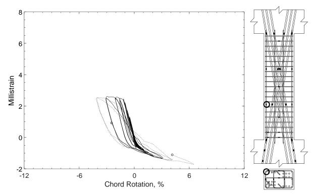
Figure 397 – Measured strain in parallel bar of D120-3.5, strain gauge H3
