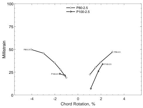
Figure 505 – Maximum strains in P-type beams during loading steps 5 through 9 (1% through 4% chord rotation), P strain gauges
