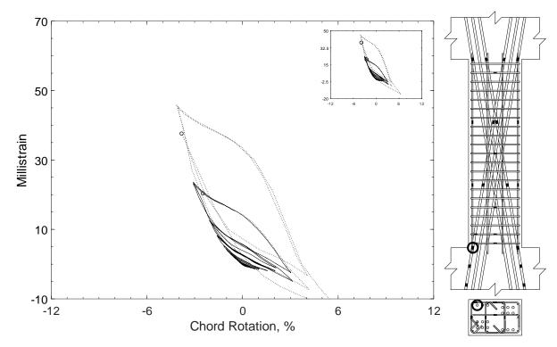
Figure 376 – Measured strain in diagonal bar of D120-3.5, strain gauge D5
