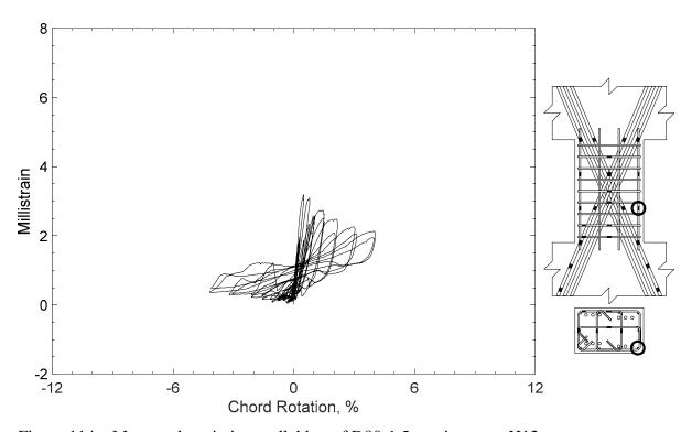
Figure 114 – Measured strain in parallel bar of D80-1.5, strain gauge H12
