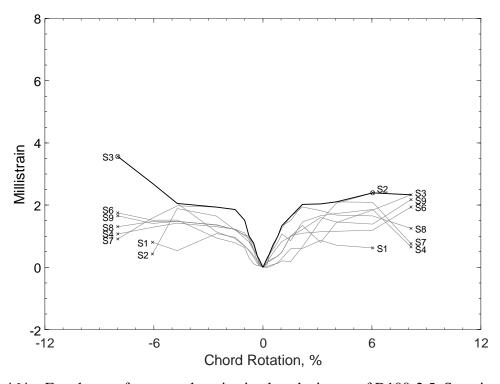
Figure 464 – Envelopes of measured strains in closed stirrups of D100-2.5, S strain gauges
