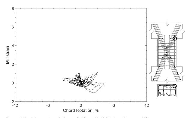
Figure 191 – Measured strain in parallel bar of D120-1.5, strain gauge H8
