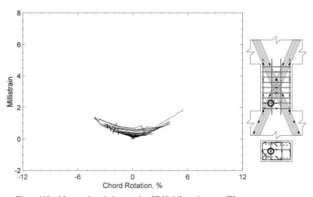
Figure 118 – Measured strain in crosstie of D80-1.5, strain gauge T2
