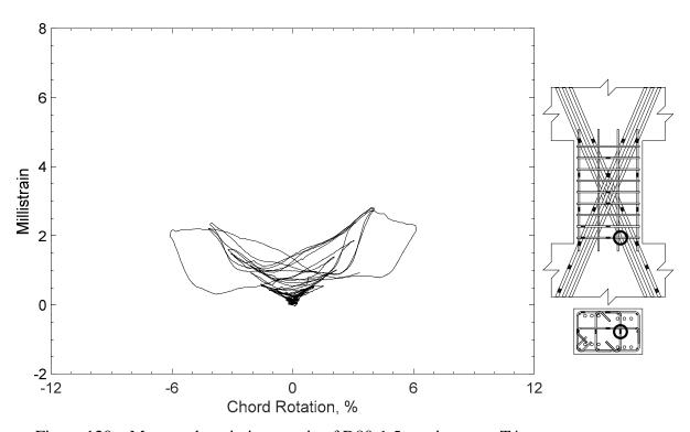
Figure 120 – Measured strain in crosstie of D80-1.5, strain gauge T4
