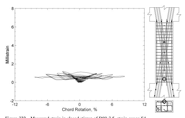
Figure 322 – Measured strain in closed stirrup of D80-3.5, strain gauge S4
