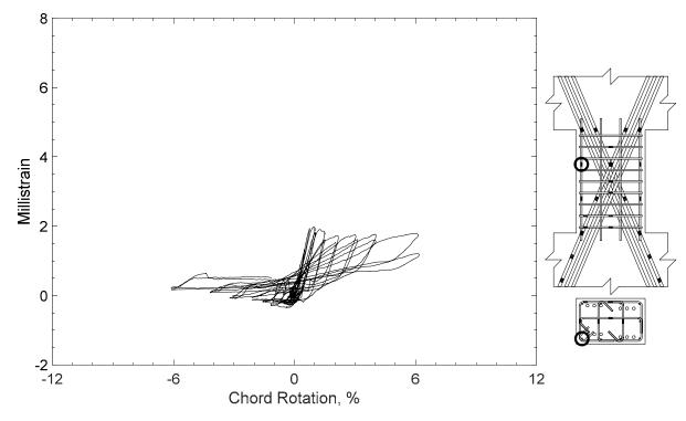
Figure 115 – Measured strain in parallel bar of D80-1.5, strain gauge H13
