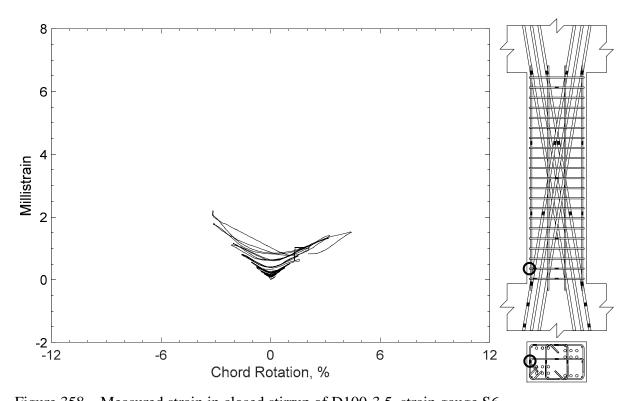
Figure 358 – Measured strain in closed stirrup of D100-3.5, strain gauge S6
