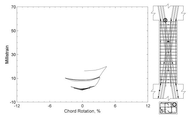
Figure 349 – Measured strain in diagonal bar of D100-3.5, strain gauge D11
