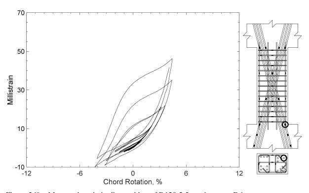
Figure 269 – Measured strain in diagonal bar of D120-2.5, strain gauge D6
