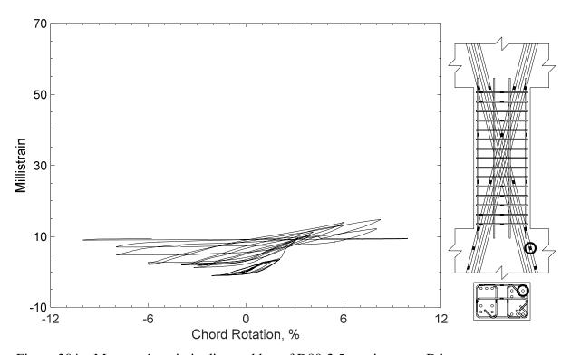
Figure 204 – Measured strain in diagonal bar of D80-2.5, strain gauge D4
