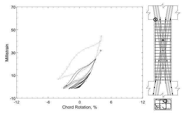
Figure 384 – Measured strain in diagonal bar of D120-3.5, strain gauge D13
