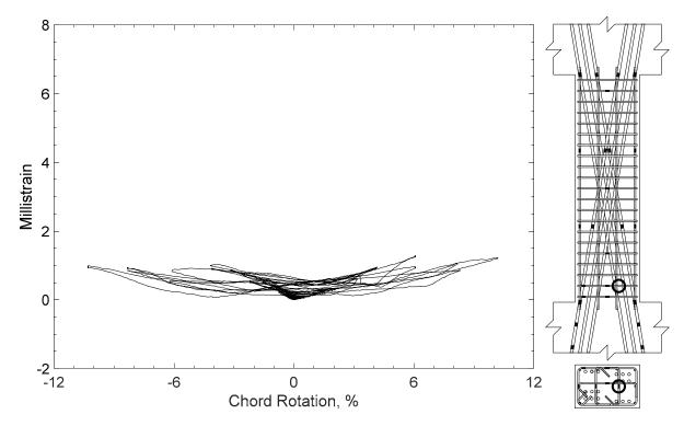
Figure 336 – Measured strain in crosstie of D80-3.5, strain gauge T1
