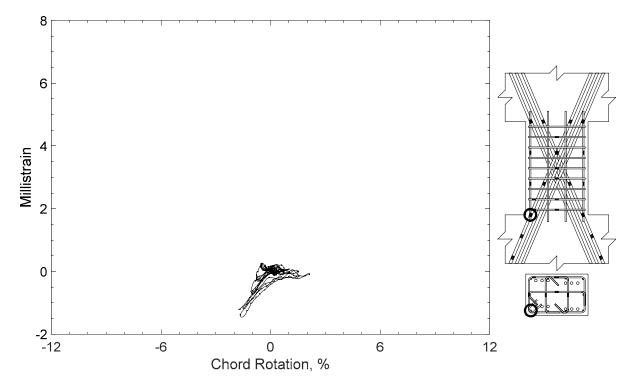
Figure 192 – Measured strain in parallel bar of D120-1.5, strain gauge H9
