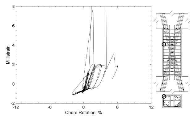
Figure 228 – Measured strain in parallel bar of D80-2.5, strain gauge H5
