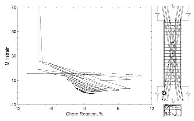
Figure 307 – Measured strain in diagonal bar of D80-3.5, strain gauge D3
