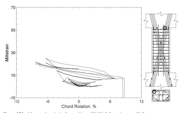
Figure 275 – Measured strain in diagonal bar of D120-2.5, strain gauge D12
