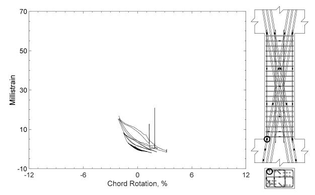
Figure 343 – Measured strain in diagonal bar of D100-3.5, strain gauge D5
