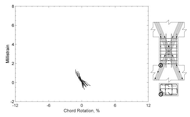
Figure 112 – Measured strain in parallel bar of D80-1.5, strain gauge H9
