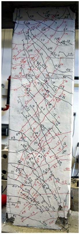
Figure C.60 – D80-3.5 during second cycle to 2% chord rotation
