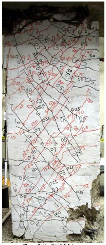
Figure C.41 – D100-2.5 during second cycle to 6% chord rotation
