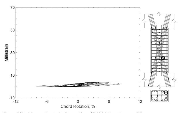
Figure 239 – Measured strain in diagonal bar of D100-2.5, strain gauge D8
