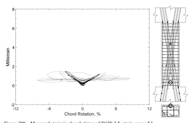
Figure 389 – Measured strain in closed stirrup of D120-3.5, strain gauge S4
