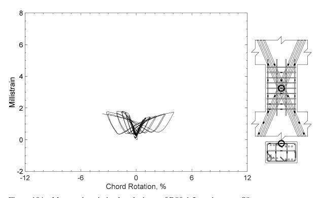
Figure 104 – Measured strain in closed stirrup of D80-1.5, strain gauge S8
