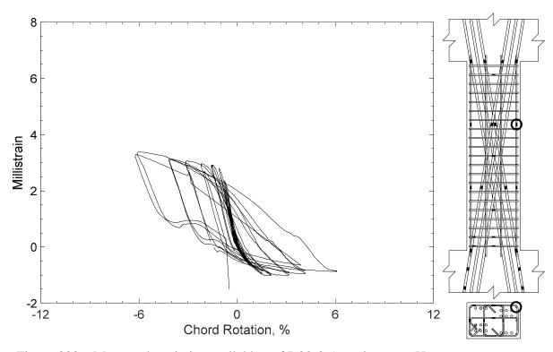
Figure 333 – Measured strain in parallel bar of D80-3.5, strain gauge H6
