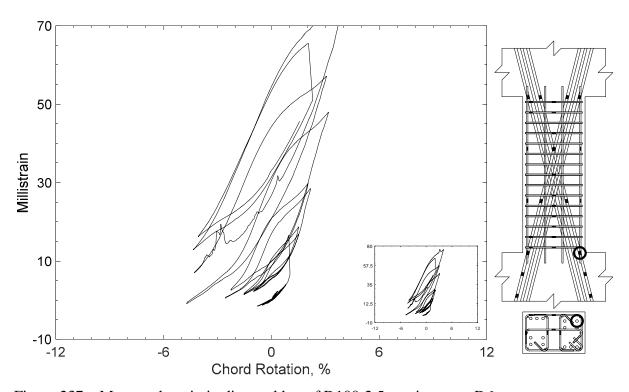
Figure 237 – Measured strain in diagonal bar of D100-2.5, strain gauge D6
