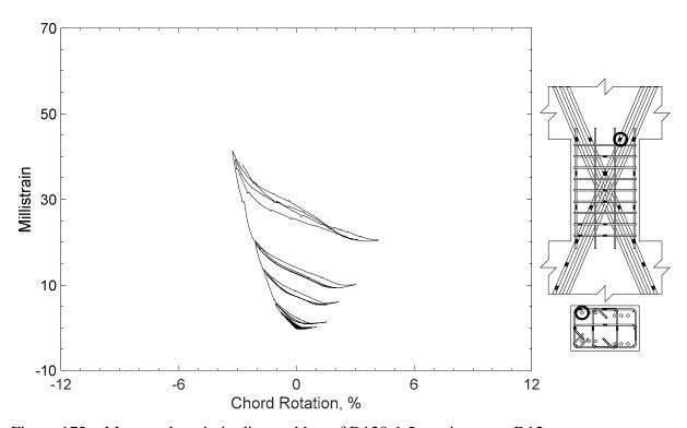
Figure 172 – Measured strain in diagonal bar of D120-1.5, strain gauge D12
