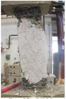
Figure C.71 – D80-3.5 at -10% chord rotation, first cycle
