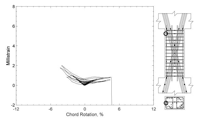
Figure 292 – Measured strain in closed stirrup of D120-2.5, strain gauge S15
