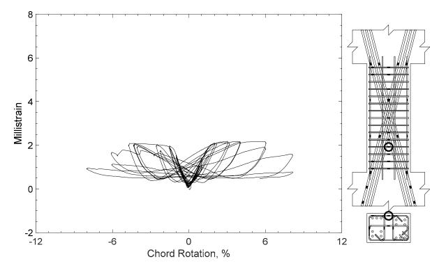
Figure 252 – Measured strain in closed stirrup of D100-2.5, strain gauge S7
