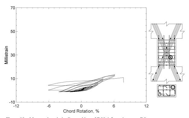
Figure 90 – Measured strain in diagonal bar of D80-1.5, strain gauge D8
