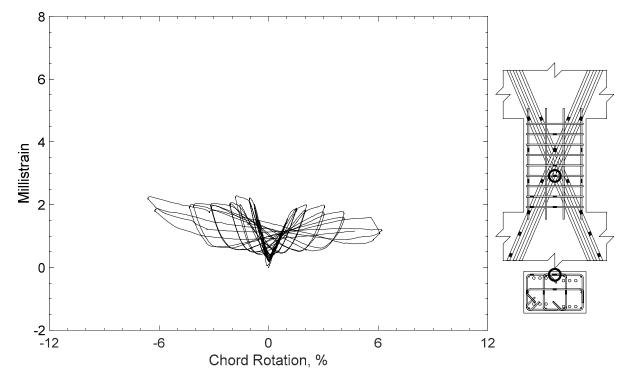
Figure 141 – Measured strain in closed stirrup of D100-1.5, strain gauge S7
