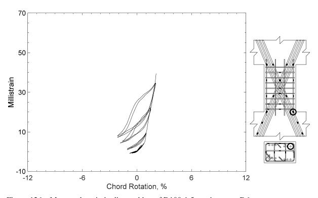
Figure 126 – Measured strain in diagonal bar of D100-1.5, strain gauge D6
