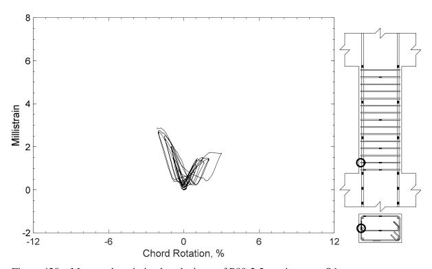
Figure 420 – Measured strain in closed stirrup of P80-2.5, strain gauge S6
