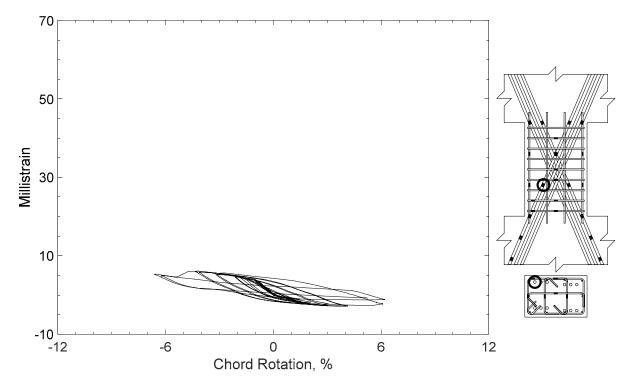
Figure 127 – Measured strain in diagonal bar of D100-1.5, strain gauge D7
