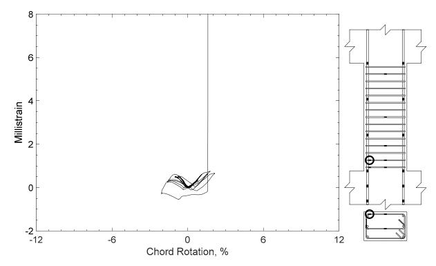
Figure 441 – Measured strain in closed stirrup of P100-2.5, strain gauge S5
