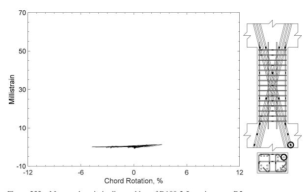
Figure 233 – Measured strain in diagonal bar of D100-2.5, strain gauge D2
