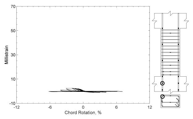
Figure 405 – Measured strain in parallel bar of P80-2.5, strain gauge P3
