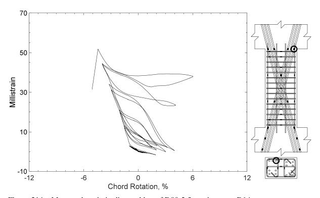
Figure 214 – Measured strain in diagonal bar of D80-2.5, strain gauge D14
