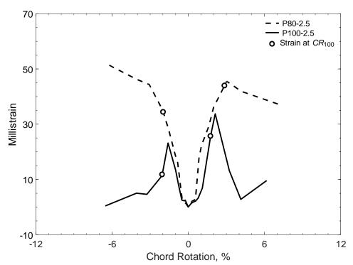
Figure 501 – Envelopes of measured strains in parallel bars of P-type beams with an aspect ratio of 2.5, P strain gauges
