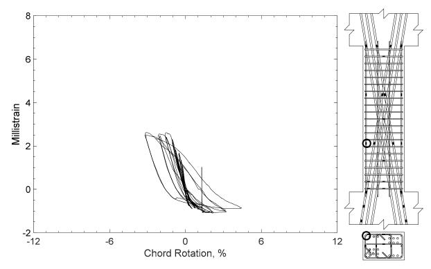
Figure 364 – Measured strain in parallel bar of D100-3.5, strain gauge H3
