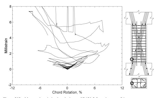
Figure 283 – Measured strain in closed stirrup of D120-2.5, strain gauge S6
