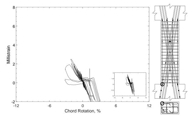
Figure 362 – Measured strain in parallel bar of D100-3.5, strain gauge H1
