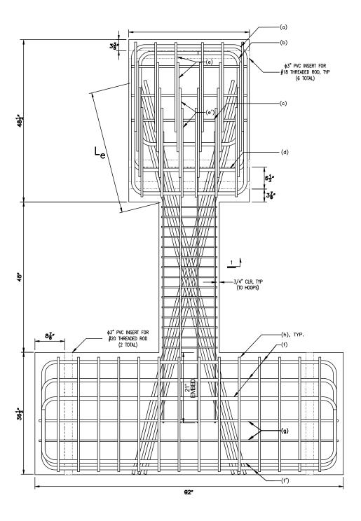
Figure 12 – Elevation view of D120-2.5 (1 in. = 25.4 mm)
