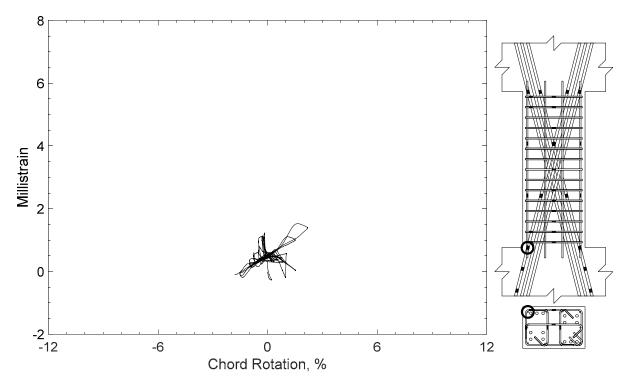
Figure 255 – Measured strain in parallel bar of D100-2.5, strain gauge H1
