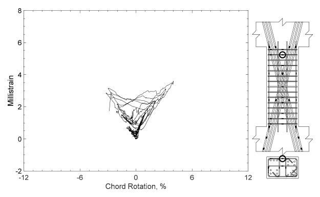
Figure 223 – Measured strain in closed stirrup of D80-2.5, strain gauge S9
