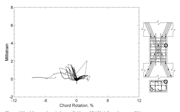
Figure 189 – Measured strain in parallel bar of D120-1.5, strain gauge H6
