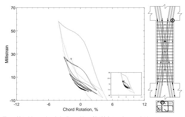
Figure 385 – Measured strain in diagonal bar of D120-3.5, strain gauge D14
