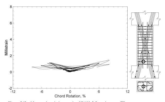
Figure 262 – Measured strain in crosstie of D100-2.5, strain gauge T2
