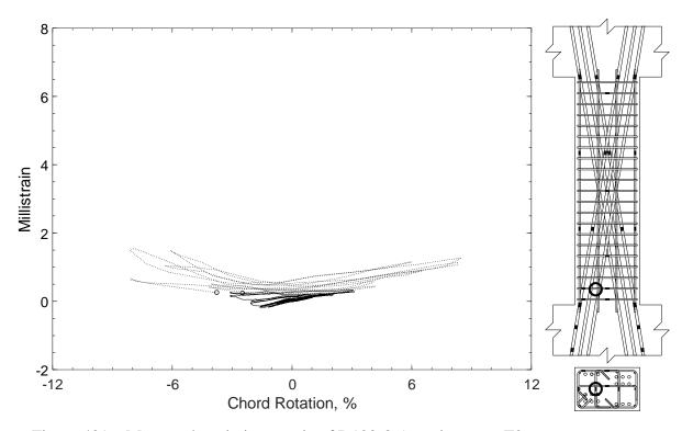
Figure 401 – Measured strain in crosstie of D120-3.5, strain gauge T2
