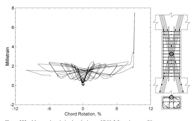
Figure 222 – Measured strain in closed stirrup of D80-2.5, strain gauge S8
