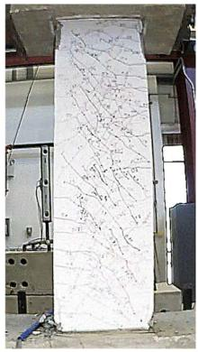
Figure C.86 – D120-3.5 at +2% chord rotation, second cycle
