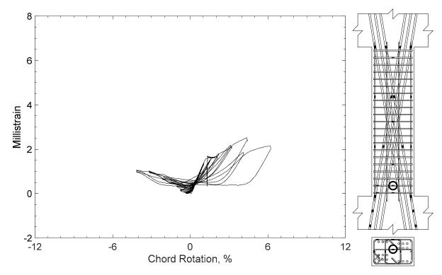
Figure 371 – Measured strain in crosstie of D100-3.5, strain gauge T3
