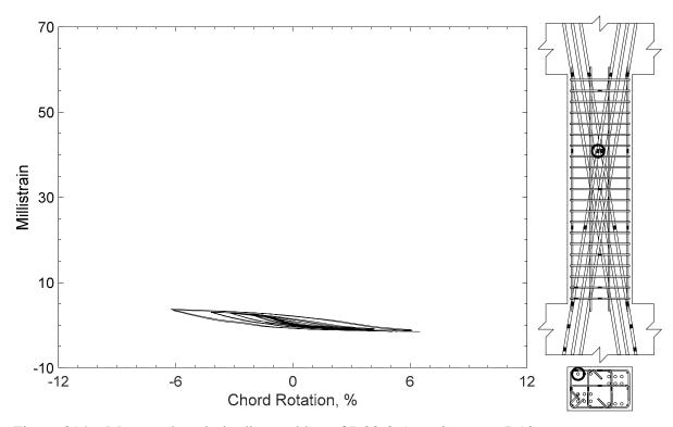
Figure 314 – Measured strain in diagonal bar of D80-3.5, strain gauge D10
