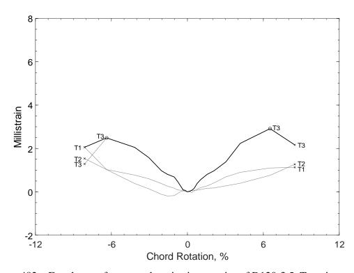
Figure 482 – Envelopes of measured strains in crossties of D120-3.5, T strain gauges
