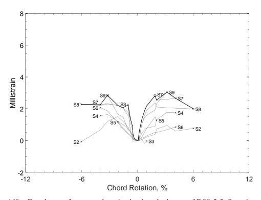
Figure 460 – Envelopes of measured strains in closed stirrups of D80-2.5, S strain gauges
