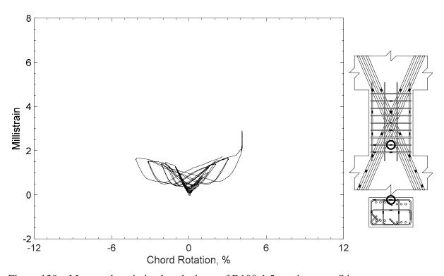
Figure 138 – Measured strain in closed stirrup of D100-1.5, strain gauge S4
