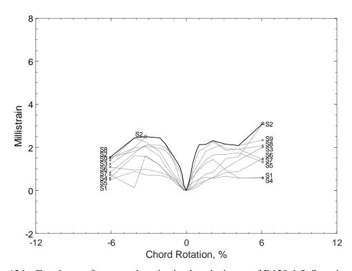
Figure 456 – Envelopes of measured strains in closed stirrups of D120-1.5, S strain gauges
