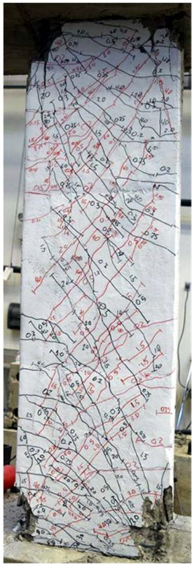
Figure C.61 – D80-3.5 during second cycle to 6% chord rotation
