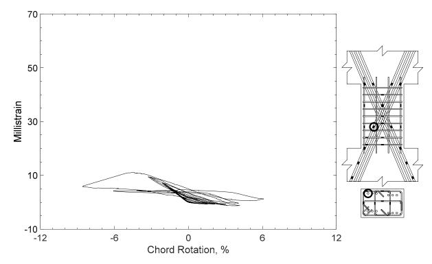
Figure 167 – Measured strain in diagonal bar of D120-1.5, strain gauge D7
