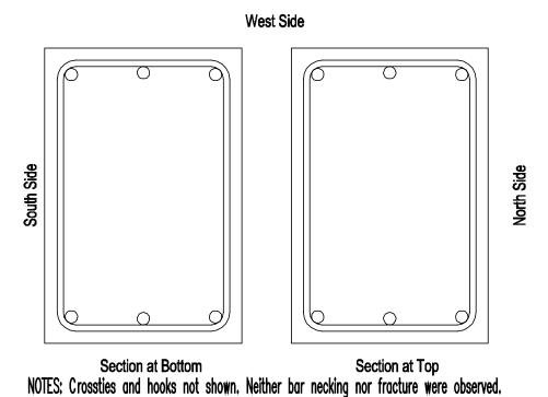
Figure 76 – Reinforcing bar fracture locations, P100-2.5
