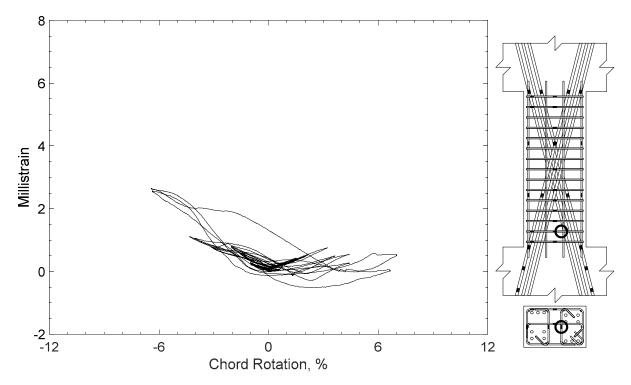
Figure 302 – Measured strain in crosstie of D120-2.5, strain gauge T1
