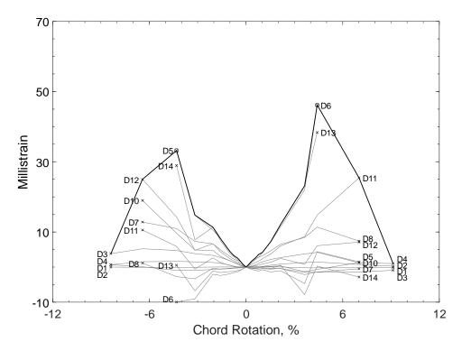
Figure 467 – Envelopes of measured strains in diagonal bars of D120-2.5, D strain gauges
