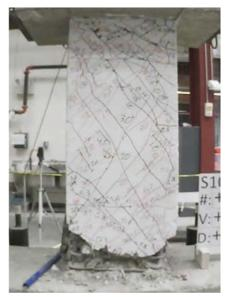
Figure C.106 – P100-2.5 at +4% chord rotation, second cycle
