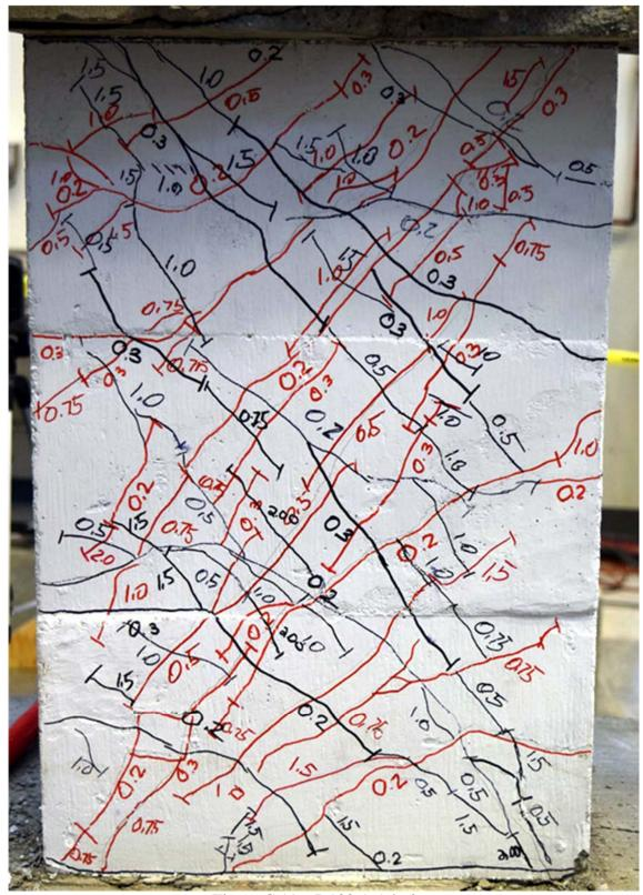
Figure C.11 – D100-1.5 during second cycle to 2% chord rotation
