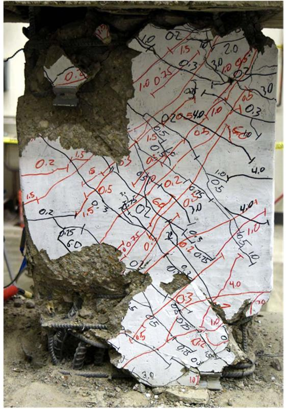
Figure C.2 – D80-1.5 during second cycle to 6% chord rotation
