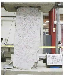
Figure C.44 – D100-2.5 at +4% chord rotation, second cycle
