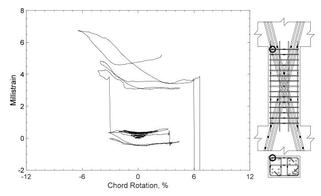
Figure 294 – Measured strain in closed stirrup of D120-2.5, strain gauge S17
