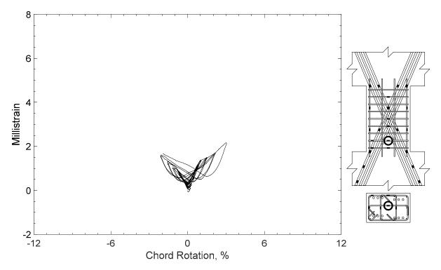
Figure 119 – Measured strain in crosstie of D80-1.5, strain gauge T3
