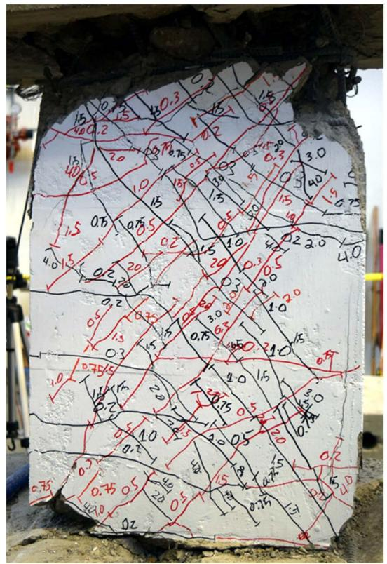
Figure C.21 – D120-1.5 during first cycle to 6% chord rotation
