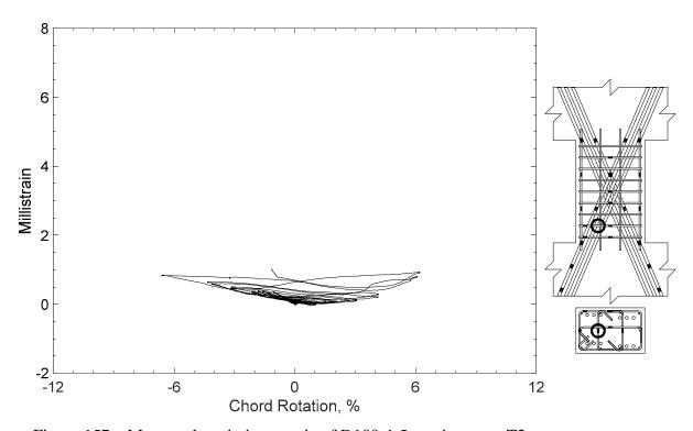
Figure 157 – Measured strain in crosstie of D100-1.5, strain gauge T2
