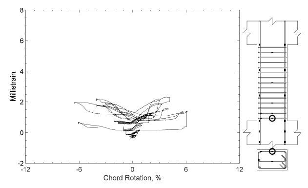
Figure 437 – Measured strain in closed stirrup of P100-2.5, strain gauge S1
