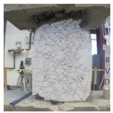
Figure C.26 – D120-1.5 at +6% chord rotation, first cycle
