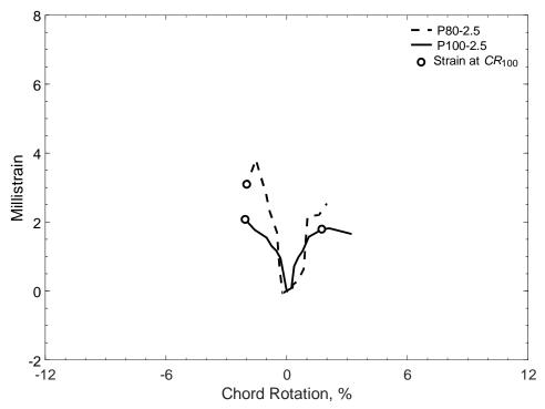
Figure 503 – Envelopes of measured strains in crossties of P-type beams with aspect ratio of 2.5, T strain gauges
