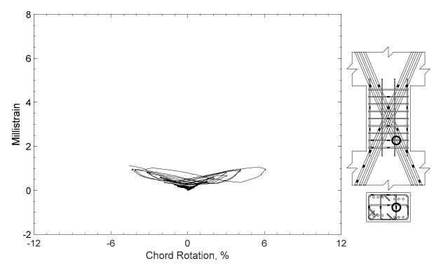
Figure 156 – Measured strain in crosstie of D100-1.5, strain gauge T1
