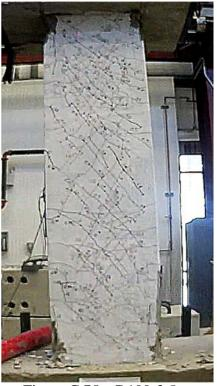
Figure C.75 – D100-3.5 at -2% chord rotation, second cycle
