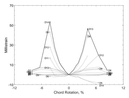
Figure 479 – Envelopes of measured strains in diagonal bars of D120-3.5, D strain gauges
