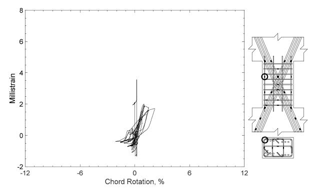
Figure 110 – Measured strain in parallel bar of D80-1.5, strain gauge H5
