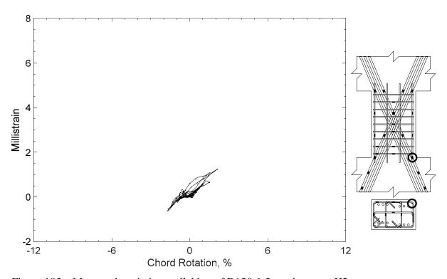
Figure 185 – Measured strain in parallel bar of D120-1.5, strain gauge H2
