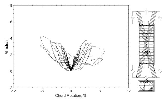
Figure 288 – Measured strain in closed stirrup of D120-2.5, strain gauge S11
