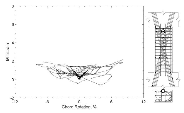
Figure 254 – Measured strain in closed stirrup of D100-2.5, strain gauge S9
