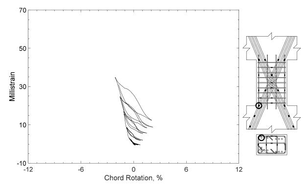
Figure 87 – Measured strain in diagonal bar of D80-1.5, strain gauge D5
