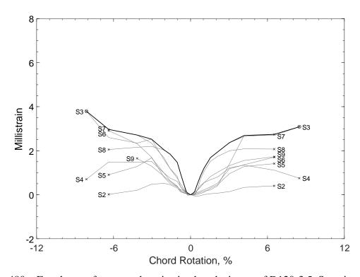
Figure 480 – Envelopes of measured strains in closed stirrups of D120-3.5, S strain gauges
