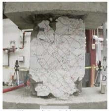
Figure C.7 – D80-1.5 at +6% chord rotation, second cycle
