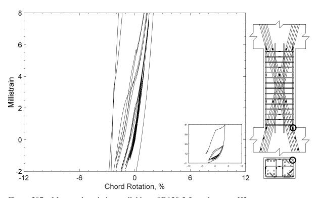
Figure 297 – Measured strain in parallel bar of D120-2.5, strain gauge H2
