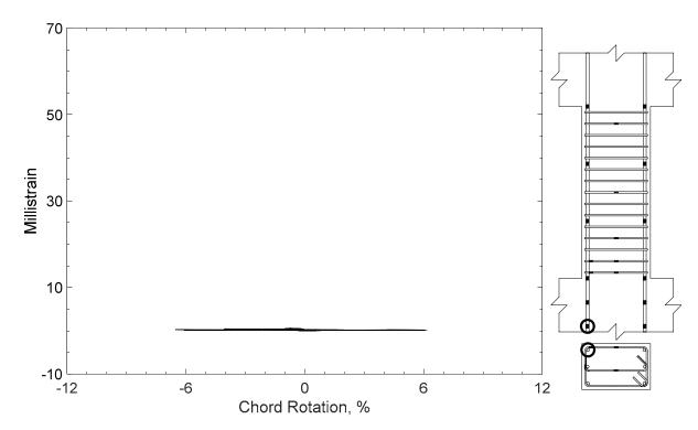
Figure 425 – Measured strain in parallel bar of P100-2.5, strain gauge P1
