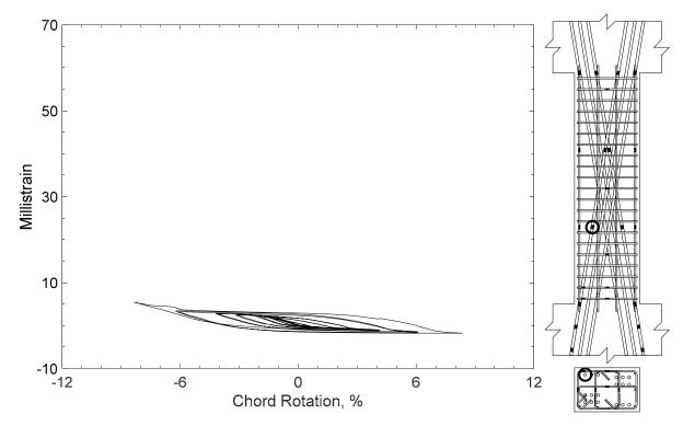
Figure 311 – Measured strain in diagonal bar of D80-3.5, strain gauge D7
