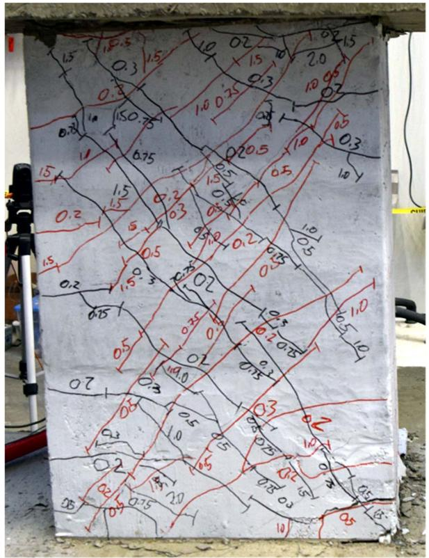
Figure C.1 – D80-1.5 during second cycle to 2% chord rotation
