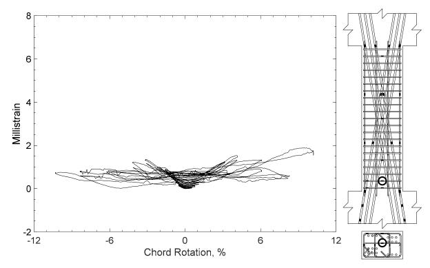
Figure 338 – Measured strain in crosstie of D80-3.5, strain gauge T3
