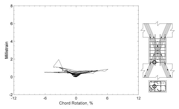
Figure 199 – Measured strain in crosstie of D120-1.5, strain gauge T5
