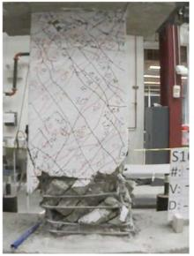
Figure C.109 – P100-2.5 at -6% chord rotation, second cycle
