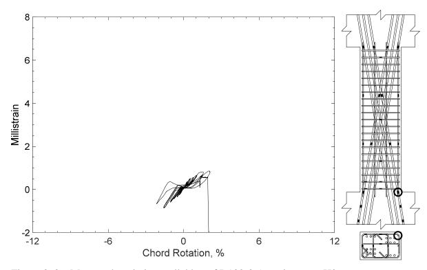
Figure 363 – Measured strain in parallel bar of D100-3.5, strain gauge H2
