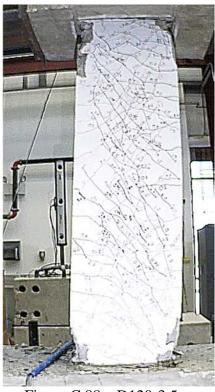
Figure C.88 – D120-3.5 at +4% chord rotation, second cycle
