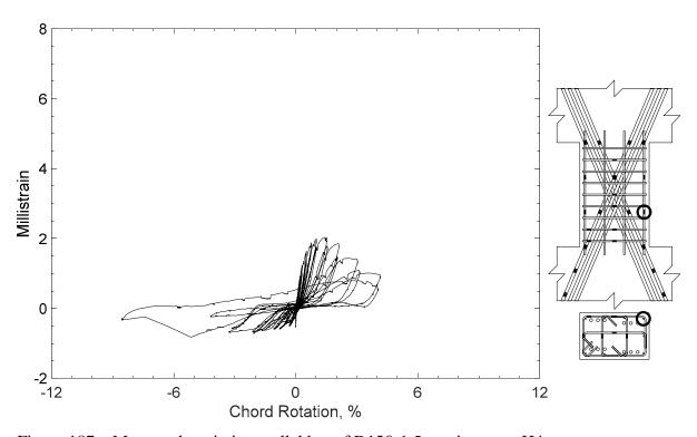
Figure 187 – Measured strain in parallel bar of D120-1.5, strain gauge H4
