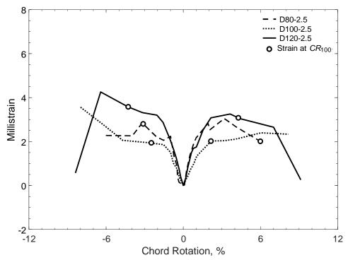
Figure 494 – Envelopes of measured strains in closed stirrups of D-type beams with an aspect ratio of 2.5, S strain gauges
