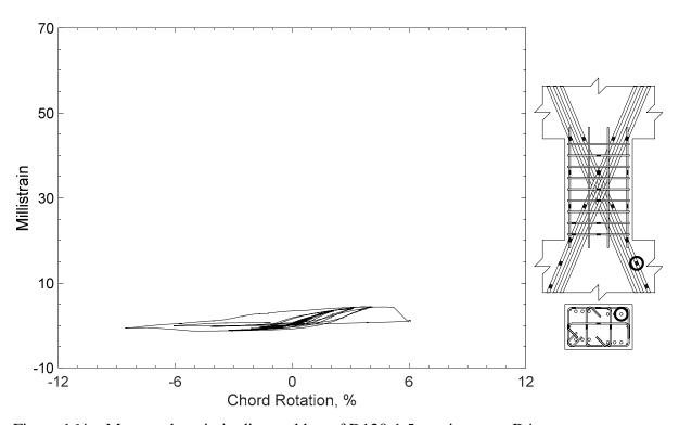
Figure 164 – Measured strain in diagonal bar of D120-1.5, strain gauge D4
