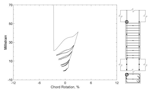
Figure 413 – Measured strain in parallel bar of P80-2.5, strain gauge P11
