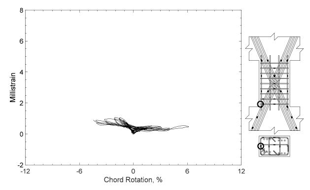
Figure 99 – Measured strain in closed stirrup of D80-1.5, strain gauge S3
