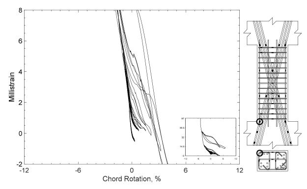
Figure 296 – Measured strain in parallel bar of D120-2.5, strain gauge H1
