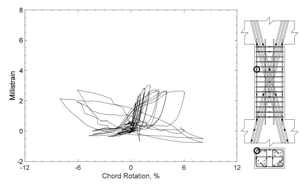
Figure 259 – Measured strain in parallel bar of D100-2.5, strain gauge H5
