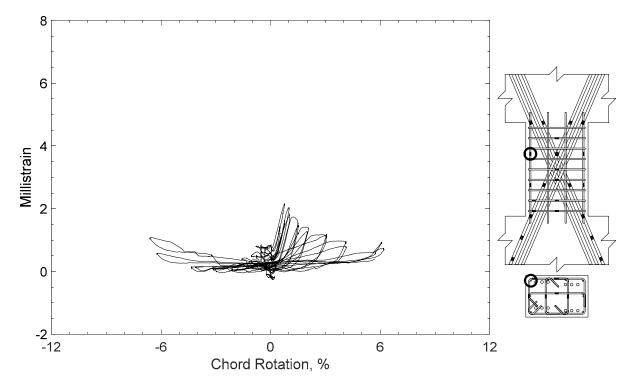
Figure 148 – Measured strain in parallel bar of D100-1.5, strain gauge H5
