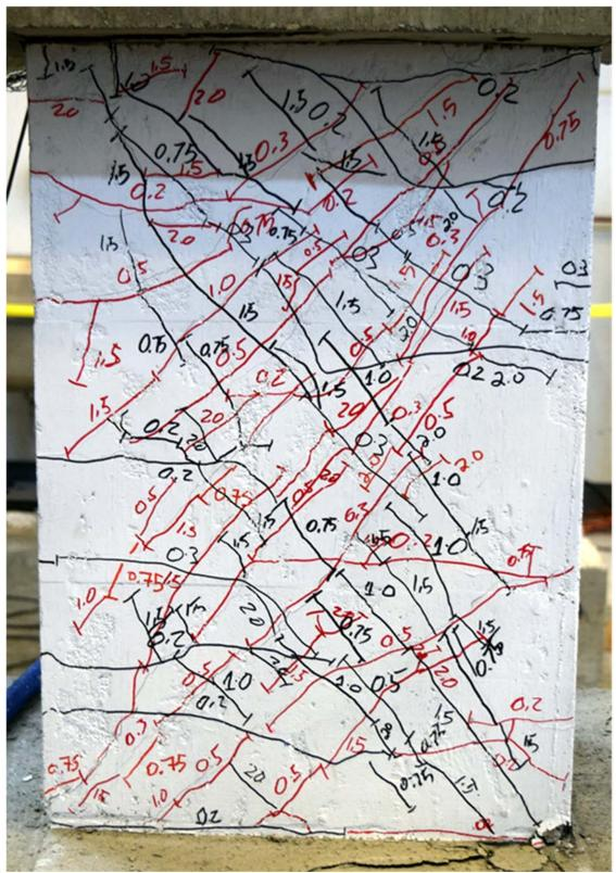
Figure C.20 – D120-1.5 during second cycle to 2% chord rotation
