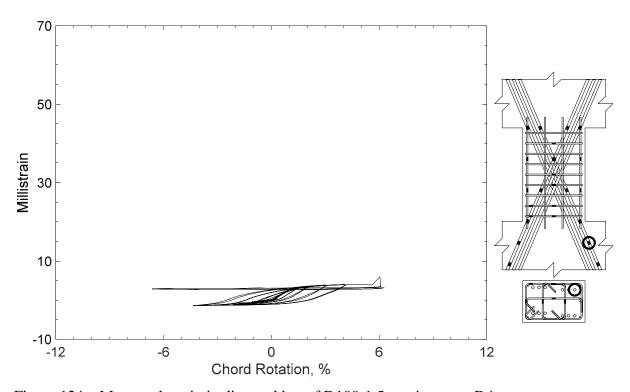
Figure 124 – Measured strain in diagonal bar of D100-1.5, strain gauge D4
