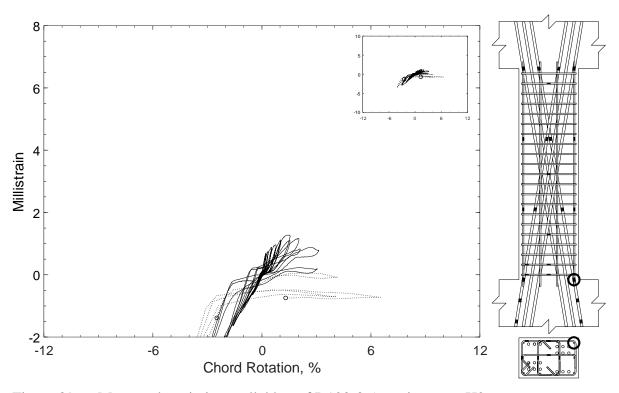
Figure 396 – Measured strain in parallel bar of D120-3.5, strain gauge H2
