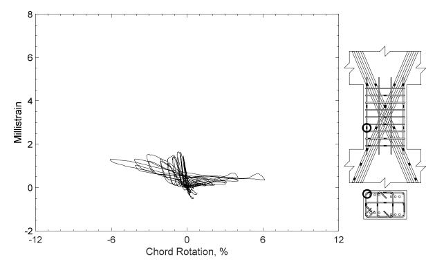
Figure 108 – Measured strain in parallel bar of D80-1.5, strain gauge H3
