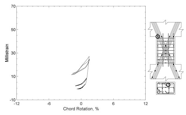
Figure 133 – Measured strain in diagonal bar of D100-1.5, strain gauge D13
