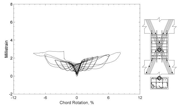
Figure 103 – Measured strain in closed stirrup of D80-1.5, strain gauge S7
