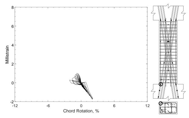
Figure 395 – Measured strain in parallel bar of D120-3.5, strain gauge H1
