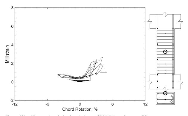
Figure 422 – Measured strain in closed stirrup of P80-2.5, strain gauge S8
