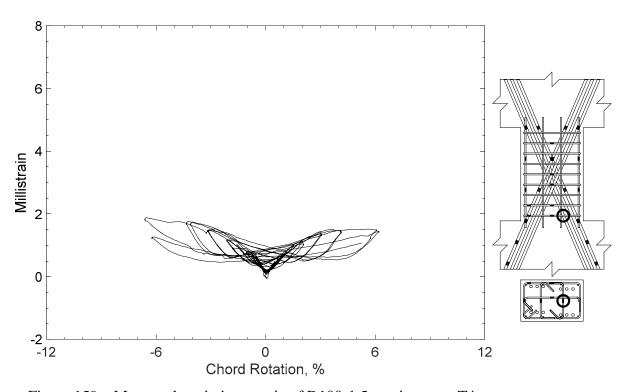
Figure 159 – Measured strain in crosstie of D100-1.5, strain gauge T4
