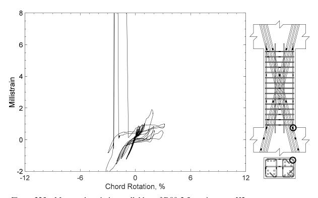
Figure 225 – Measured strain in parallel bar of D80-2.5, strain gauge H2
