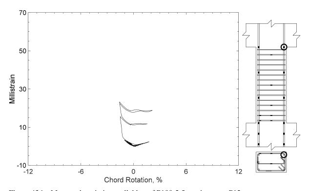
Figure 436 – Measured strain in parallel bar of P100-2.5, strain gauge P12
