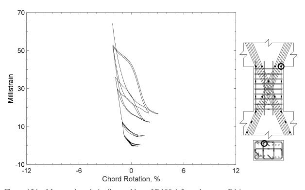
Figure 134 – Measured strain in diagonal bar of D100-1.5, strain gauge D14
