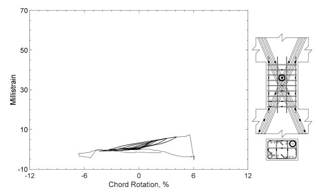
Figure 129 – Measured strain in diagonal bar of D100-1.5, strain gauge D9
