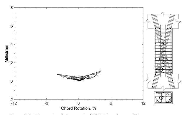
Figure 230 – Measured strain in crosstie of D80-2.5, strain gauge T2
