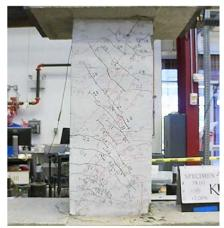
Figure C.30 – D80-2.5 at +2% chord rotation, second cycle
