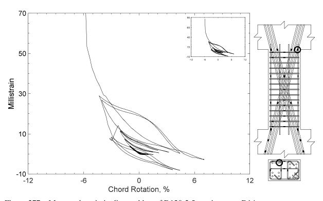
Figure 277 – Measured strain in diagonal bar of D120-2.5, strain gauge D14
