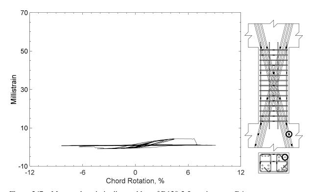
Figure 267 – Measured strain in diagonal bar of D120-2.5, strain gauge D4
