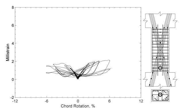
Figure 263 – Measured strain in crosstie of D100-2.5, strain gauge T3
