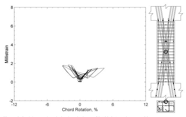
Figure 360 – Measured strain in closed stirrup of D100-3.5, strain gauge S8
