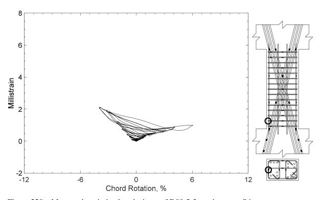
Figure 220 – Measured strain in closed stirrup of D80-2.5, strain gauge S6
