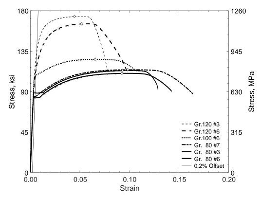
Figure 24 – Measured stress versus strain for reinforcement
