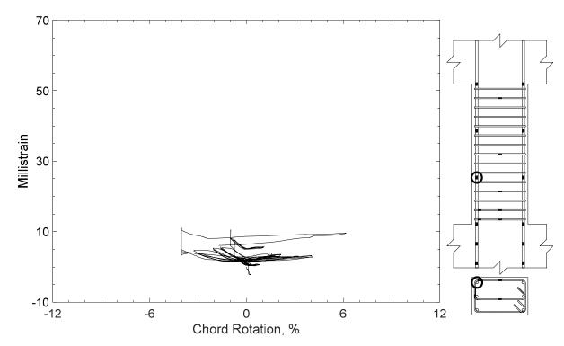
Figure 431 – Measured strain in parallel bar of P100-2.5, strain gauge P7
