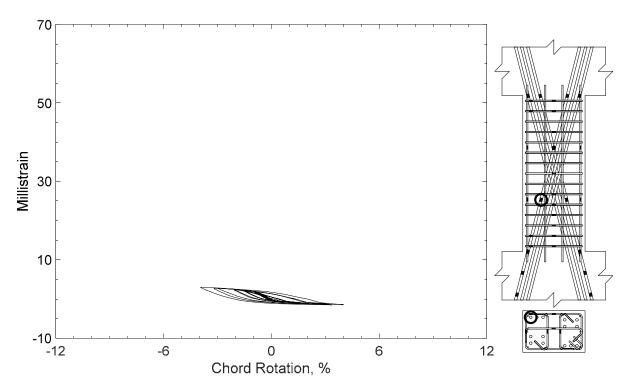
Figure 207 – Measured strain in diagonal bar of D80-2.5, strain gauge D7
