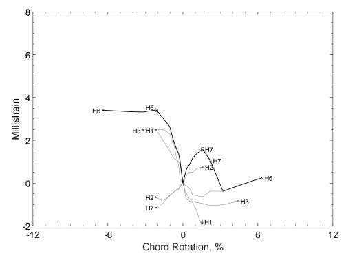
Figure 477 – Envelopes of measured strains in parallel bars of D100-3.5, H strain gauges
