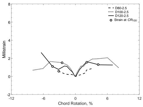
Figure 496 – Envelopes of measured strains in crossties of D-type beams with an aspect ratio of 2.5, T strain gauges
