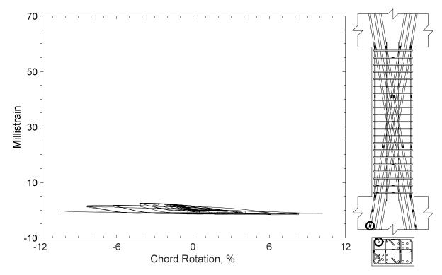
Figure 305 – Measured strain in diagonal bar of D80-3.5, strain gauge D1
