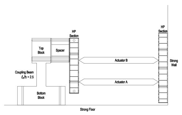
Figure 29 – Test setup for coupling beams with aspect ratio of 2.5<sup>a</sup>
