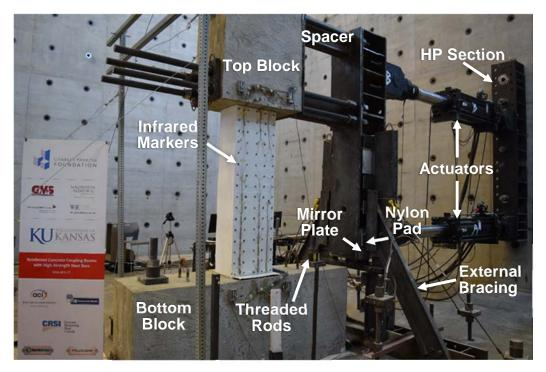
Figure 25 – Test setup, view from northeast
