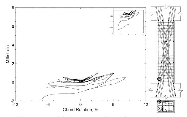
Figure 323 – Measured strain in closed stirrup of D80-3.5, strain gauge S5
