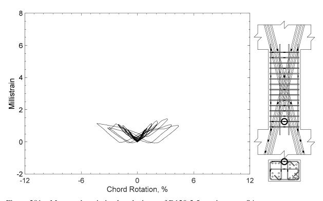
Figure 281 – Measured strain in closed stirrup of D120-2.5, strain gauge S4
