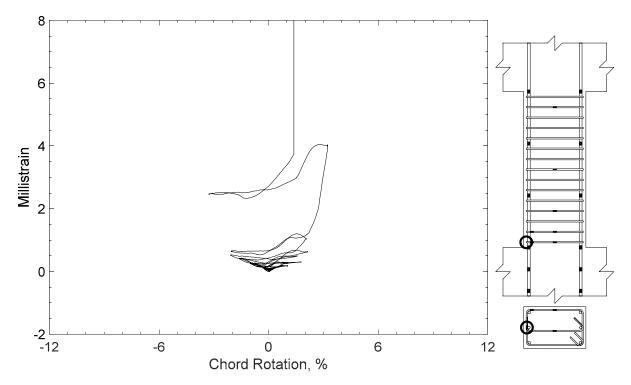
Figure 439 – Measured strain in closed stirrup of P100-2.5, strain gauge S3
