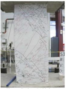
Figure C.105 – P100-2.5 at -2% chord rotation, second cycle
