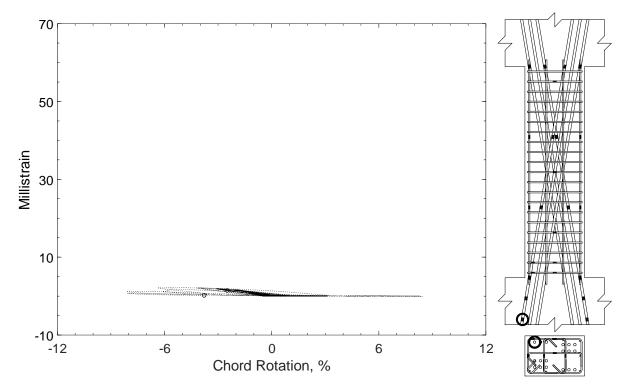
Figure 372 – Measured strain in diagonal bar of D120-3.5, strain gauge D1
