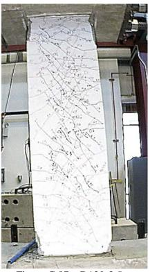
Figure C.87 – D120-3.5 at -2% chord rotation, second cycle
