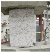
Figure C.6 – D80-1.5 at -4% chord rotation, second cycle
