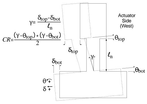
Figure 36 – General deformed shape of specimen, view from north<sup>b</sup>
