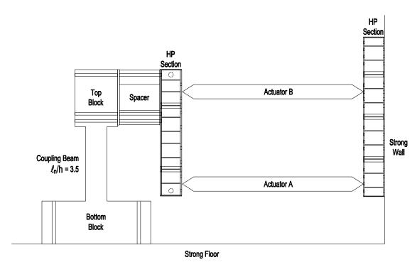
Figure 30 – Test setup for coupling beams with aspect ratio of  $3.5^{\rm a}$
