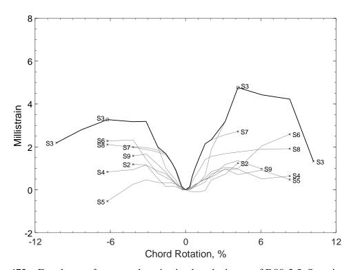
Figure 472 – Envelopes of measured strains in closed stirrups of D80-3.5, S strain gauges
