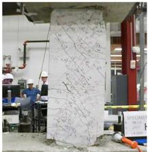
Figure C.32 – D80-2.5 at +4% chord rotation, second cycle
