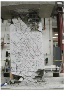
Figure C.57 – D120-2.5 at -6% chord rotation, second cycle
