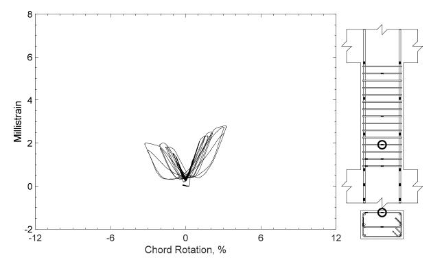
Figure 443 – Measured strain in closed stirrup of P100-2.5, strain gauge S7
