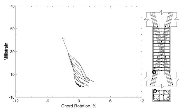
Figure 205 – Measured strain in diagonal bar of D80-2.5, strain gauge D5
