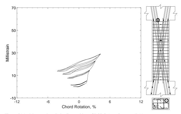
Figure 315 – Measured strain in diagonal bar of D80-3.5, strain gauge D11
