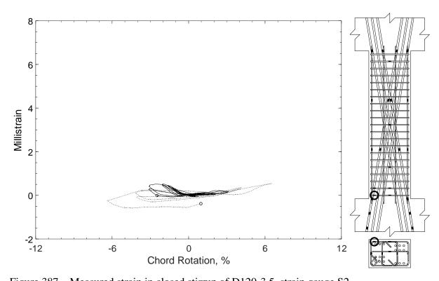
Figure 387 – Measured strain in closed stirrup of D120-3.5, strain gauge S2
