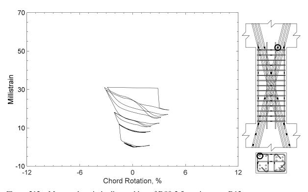
Figure 212 – Measured strain in diagonal bar of D80-2.5, strain gauge D12
