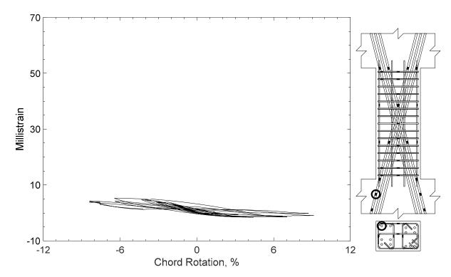
Figure 266 – Measured strain in diagonal bar of D120-2.5, strain gauge D3
