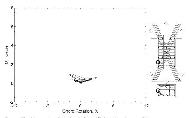
Figure 102 – Measured strain in closed stirrup of D80-1.5, strain gauge S6
