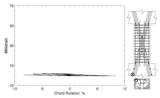
Figure 201 – Measured strain in diagonal bar of D80-2.5, strain gauge D1
