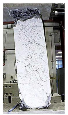
Figure C.93 – D120-3.5 at -8% chord rotation, second cycle
