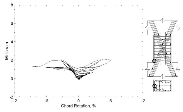
Figure 177 – Measured strain in closed stirrup of D120-1.5, strain gauge S3
