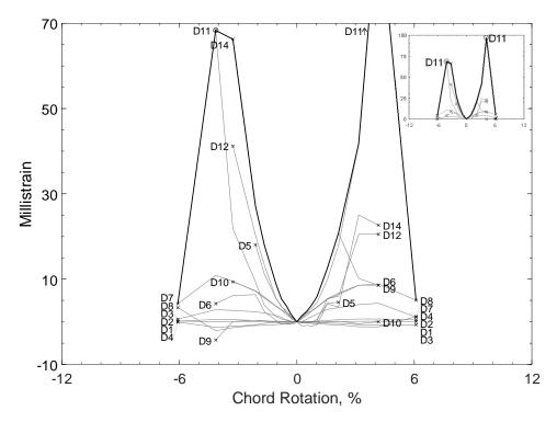
Figure 455 – Envelopes of measured strains in diagonal bars of D120-1.5, D strain gauges
