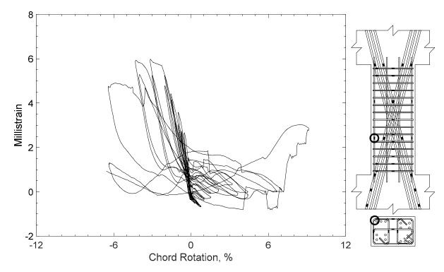
Figure 298 – Measured strain in parallel bar of D120-2.5, strain gauge H3
