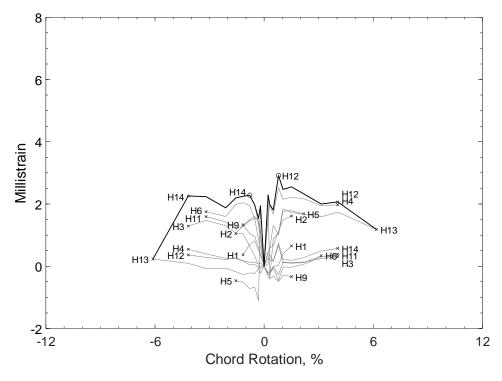
Figure 449 – Envelopes of measured strains in parallel bars of D80-1.5, H strain gauges
