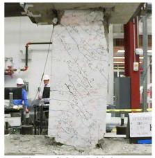
Figure C.34 – D80-2.5 at +6% chord rotation, second cycle
