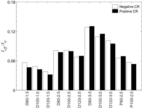
Figure 82 – Effective moment of inertia,  $I_{eff}$ , normalized by transformed uncracked moment of inertia,  $I_{tr}$
