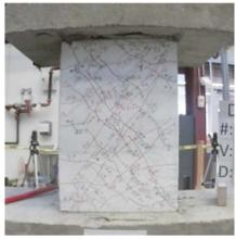
Figure C.3 – D80-1.5 at +2% chord rotation, second cycle
