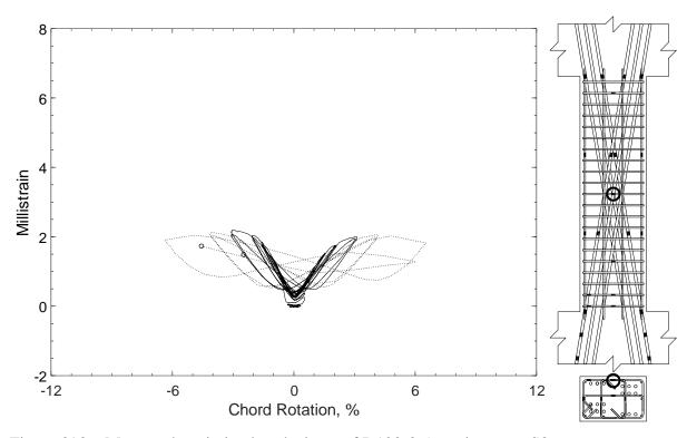
Figure 393 – Measured strain in closed stirrup of D120-3.5, strain gauge S8
