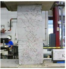
Figure C.31 – D80-2.5 at -2% chord rotation, second cycle
