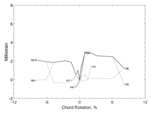
Figure 465 – Envelopes of measured strains in parallel bars of D100-2.5, H strain gauges
