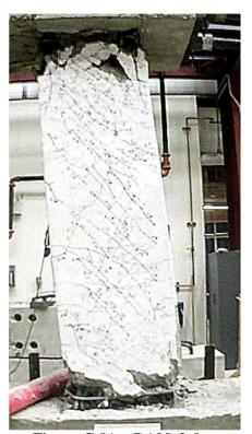
Figure C.81 – D100-3.5 at -8% chord rotation, second cycle
