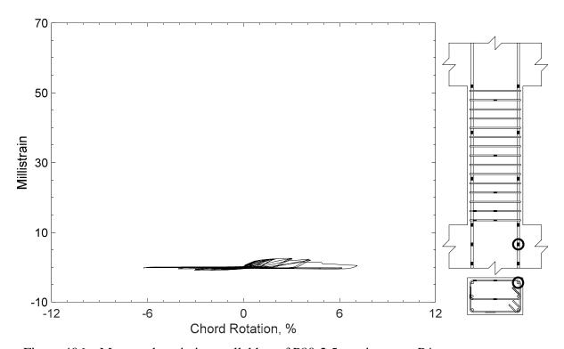
Figure 406 – Measured strain in parallel bar of P80-2.5, strain gauge P4
