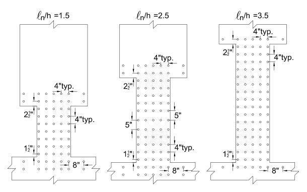
Figure 32 – Infrared marker positions (1 in. = 25.4 mm)
