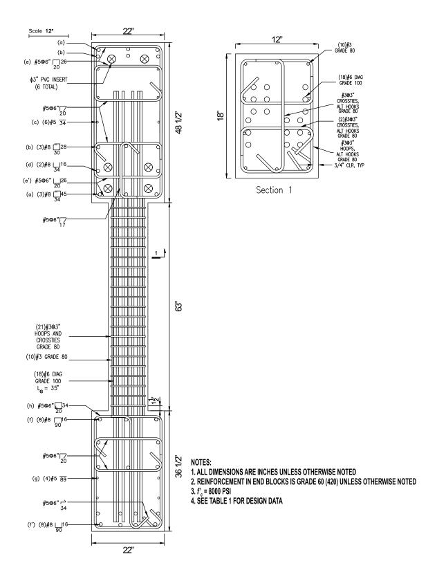
Figure 17 – Reinforcement details of D100-3.5 (1 in. = 25.4 mm, 1 ksi = 1,000 psi = 6.89 MPa)
