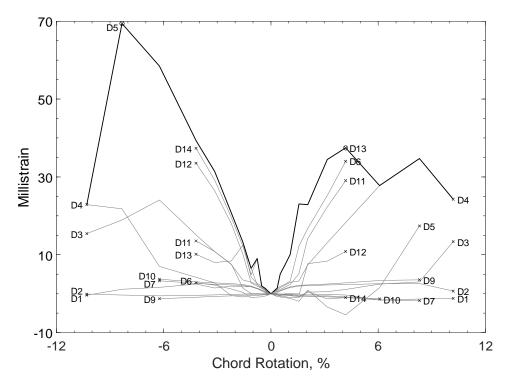
Figure 471 – Envelopes of measured strains in diagonal bars of D80-3.5, D strain gauges
