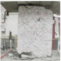
Figure C.19 – D100-1.5 at +8% chord rotation, first cycle
