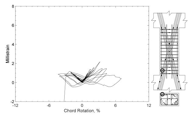
Figure 282 – Measured strain in closed stirrup of D120-2.5, strain gauge S5
