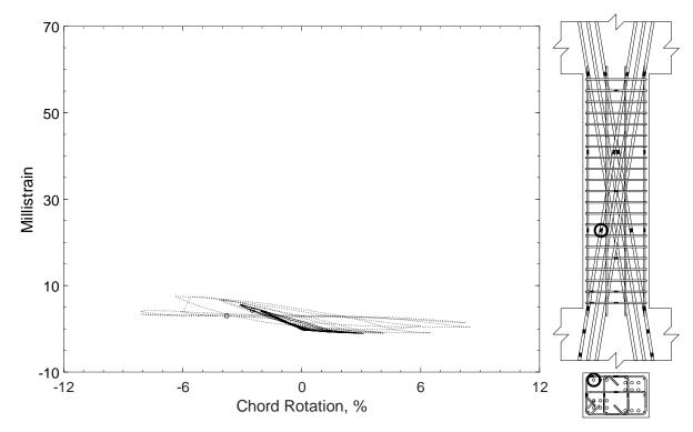
Figure 378 – Measured strain in diagonal bar of D120-3.5, strain gauge D7
