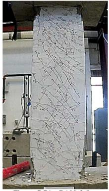
Figure C.74 – D100-3.5 at +2% chord rotation, second cycle
