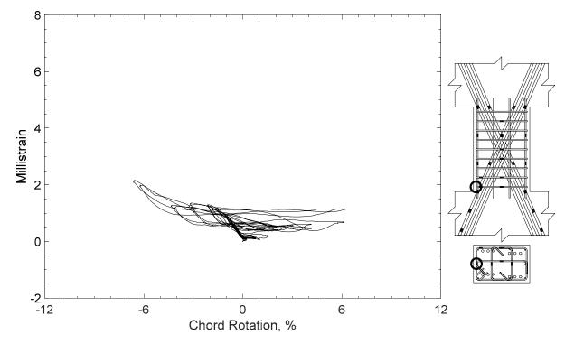
Figure 137 – Measured strain in closed stirrup of D100-1.5, strain gauge S3
