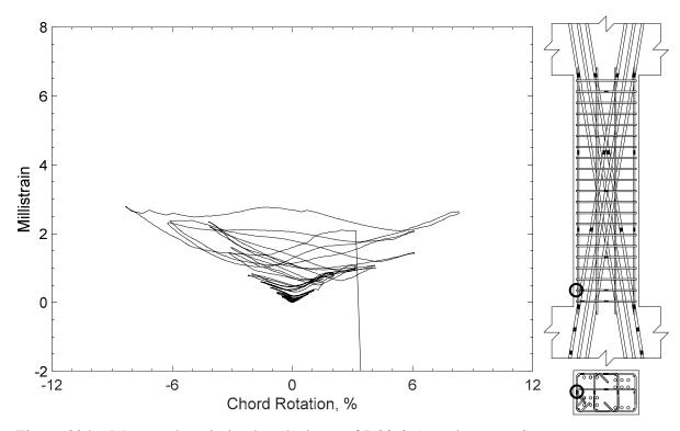
Figure 324 – Measured strain in closed stirrup of D80-3.5, strain gauge S6
