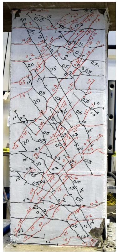
Figure C.102 – P100-2.5 during second cycle to 2% chord rotation
