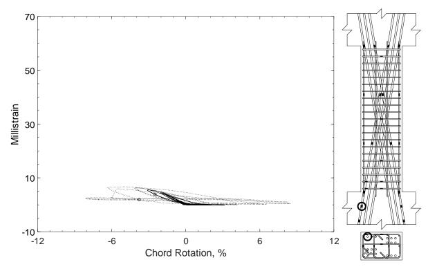
Figure 374 – Measured strain in diagonal bar of D120-3.5, strain gauge D3
