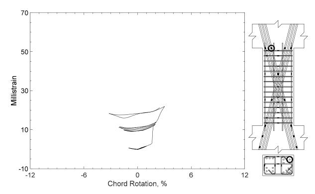
Figure 211 – Measured strain in diagonal bar of D80-2.5, strain gauge D11
