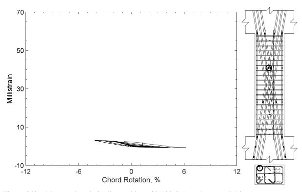
Figure 348 – Measured strain in diagonal bar of D100-3.5, strain gauge D10
