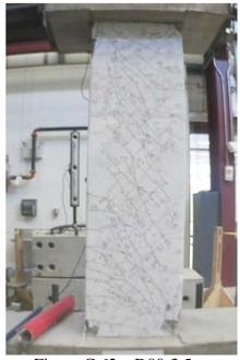
Figure C.62 – D80-3.5 at +2% chord rotation, second cycle
