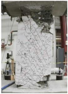
Figure C.56 – D120-2.5 at +6% chord rotation, second cycle
