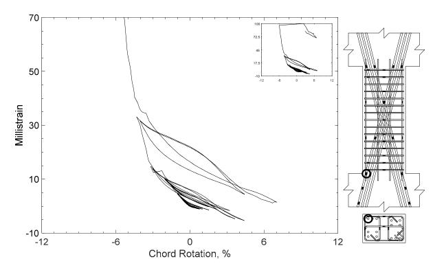
Figure 268 – Measured strain in diagonal bar of D120-2.5, strain gauge D5
