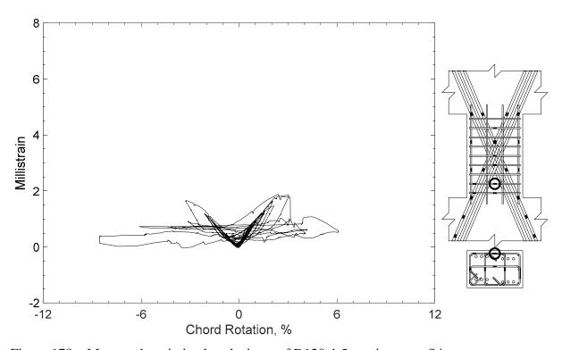
Figure 178 – Measured strain in closed stirrup of D120-1.5, strain gauge S4
