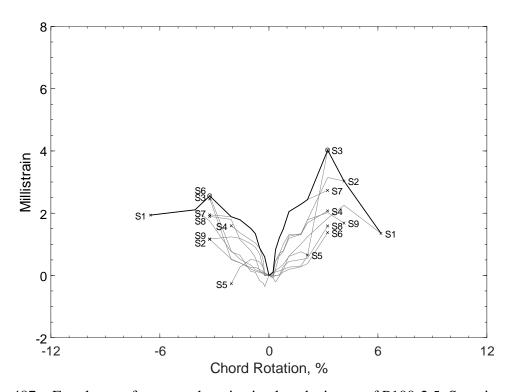
Figure 487 – Envelopes of measured strains in closed stirrups of P100-2.5, S strain gauges
