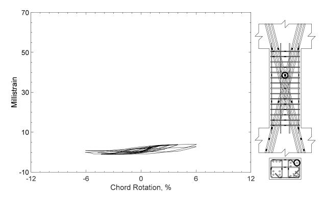
Figure 240 – Measured strain in diagonal bar of D100-2.5, strain gauge D9
