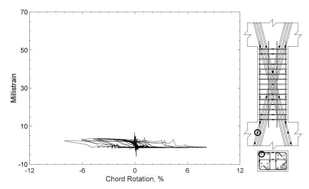
Figure 234 – Measured strain in diagonal bar of D100-2.5, strain gauge D3
