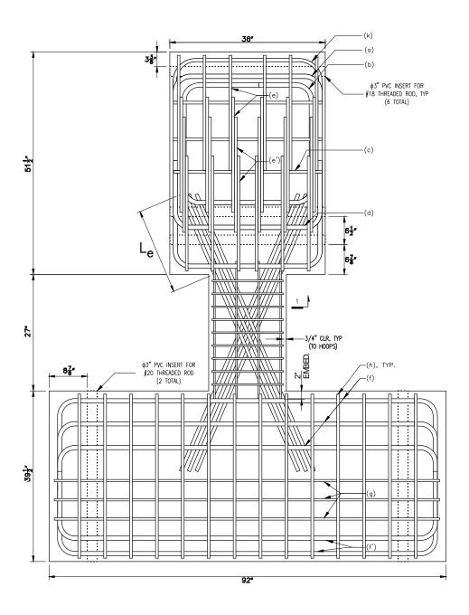
Figure 2 – Elevation view of D80-1.5 (1 in. = 25.4 mm)
