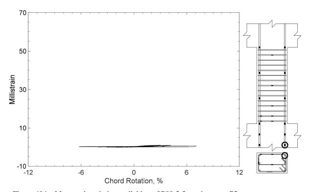
Figure 404 – Measured strain in parallel bar of P80-2.5, strain gauge P2
