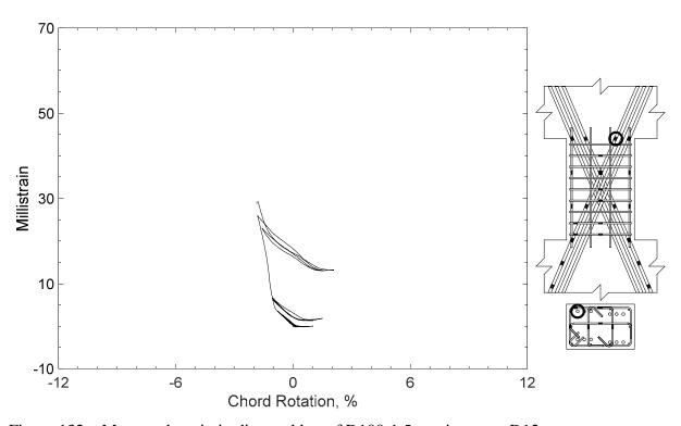
Figure 132 – Measured strain in diagonal bar of D100-1.5, strain gauge D12
