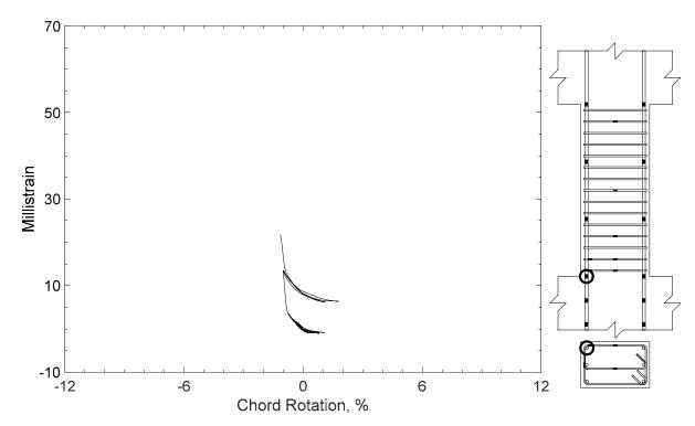
Figure 429 – Measured strain in parallel bar of P100-2.5, strain gauge P5
