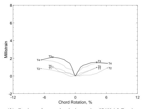
Figure 454 – Envelopes of measured strains in crossties of D100-1.5, T strain gauges
