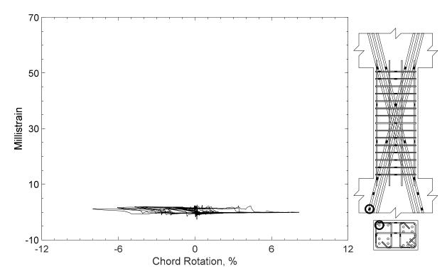
Figure 232 – Measured strain in diagonal bar of D100-2.5, strain gauge D1
