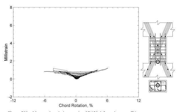
Figure 200 – Measured strain in crosstie of D120-1.5, strain gauge T6
