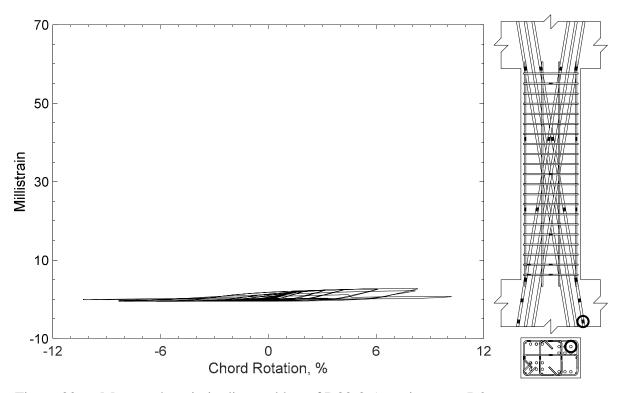
Figure 306 – Measured strain in diagonal bar of D80-3.5, strain gauge D2
