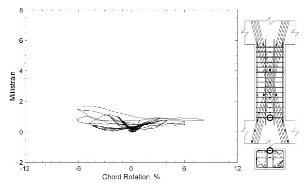
Figure 246 – Measured strain in closed stirrup of D100-2.5, strain gauge S1
