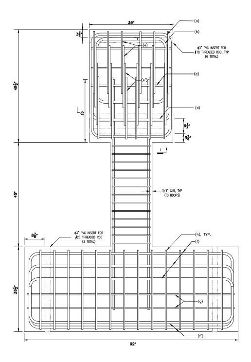
Figure 20 – Elevation view of P80-2.5 (1 in. = 25.4 mm)
