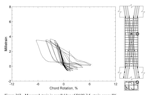
Figure 367 – Measured strain in parallel bar of D100-3.5, strain gauge H6
