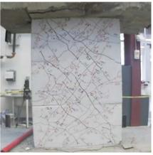
Figure C.14 – D100-1.5 at -2% chord rotation, second cycle
