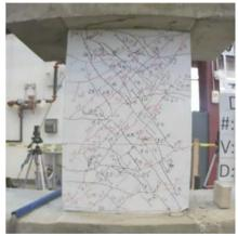
Figure C.22 – D120-1.5 at +2% chord rotation, second cycle
