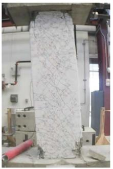
Figure C.67 – D80-3.5 at -6% chord rotation, second cycle
