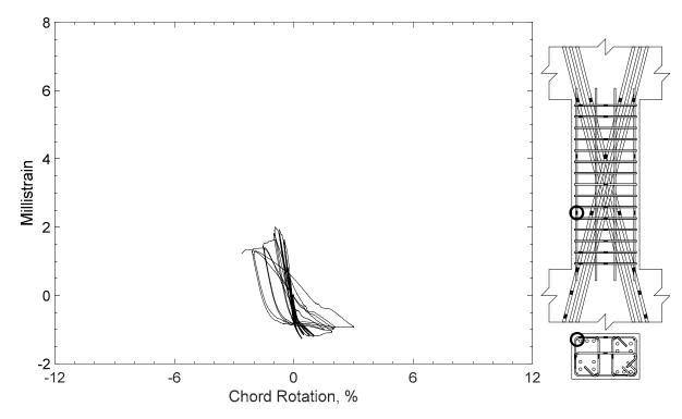
Figure 226 – Measured strain in parallel bar of D80-2.5, strain gauge H3
