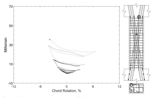
Figure 383 – Measured strain in diagonal bar of D120-3.5, strain gauge D12
