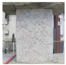
Figure C.13 – D100-1.5 at +2% chord rotation, second cycle
