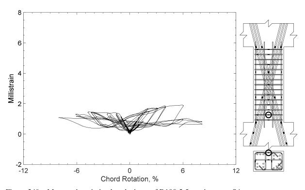
Figure 249 – Measured strain in closed stirrup of D100-2.5, strain gauge S4
