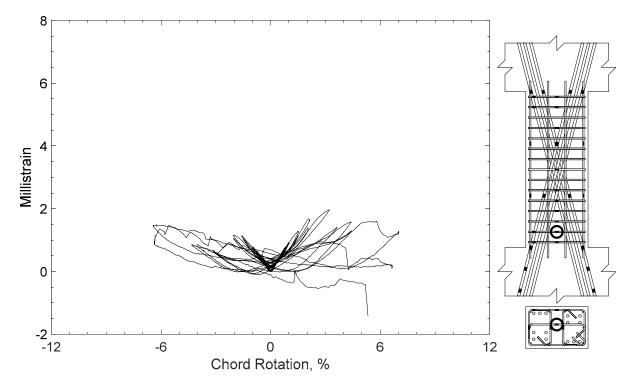
Figure 304 – Measured strain in crosstie of D120-2.5, strain gauge T3
