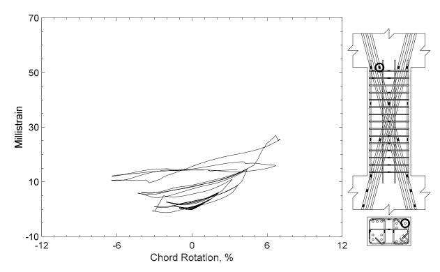
Figure 274 – Measured strain in diagonal bar of D120-2.5, strain gauge D11
