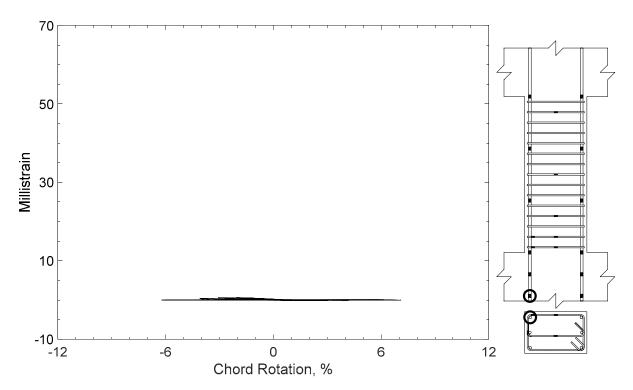
Figure 403 – Measured strain in parallel bar of P80-2.5, strain gauge P1
