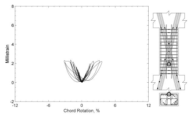
Figure 284 – Measured strain in closed stirrup of D120-2.5, strain gauge S7
