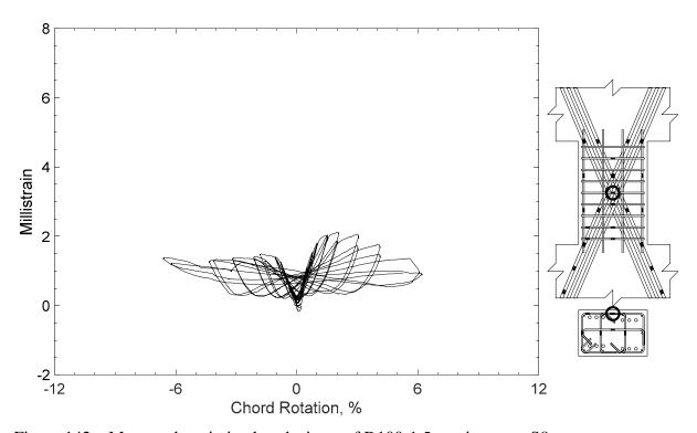
Figure 142 – Measured strain in closed stirrup of D100-1.5, strain gauge S8
