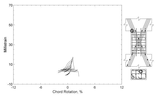
Figure 95 – Measured strain in diagonal bar of D80-1.5, strain gauge D13
