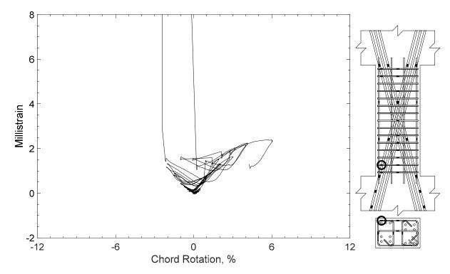
Figure 219 – Measured strain in closed stirrup of D80-2.5, strain gauge S5
