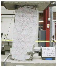
Figure C.46 – D100-2.5 at +6% chord rotation, second cycle
