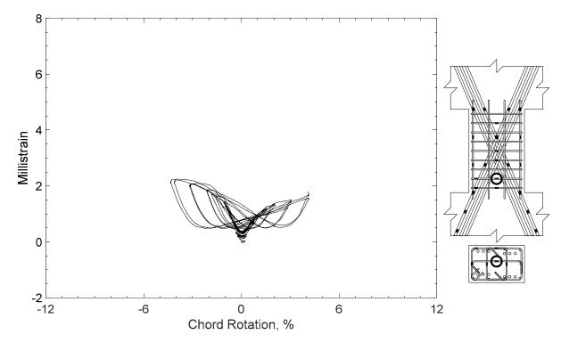
Figure 158 – Measured strain in crosstie of D100-1.5, strain gauge T3
