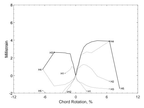
Figure 481 – Envelopes of measured strains in parallel bars of D120-3.5, H strain gauges
