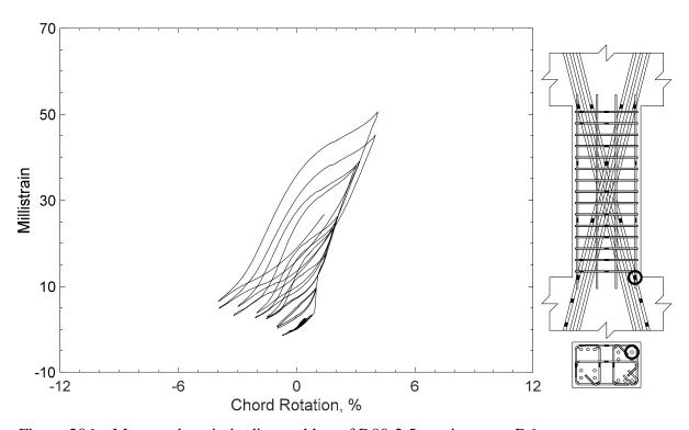
Figure 206 – Measured strain in diagonal bar of D80-2.5, strain gauge D6
