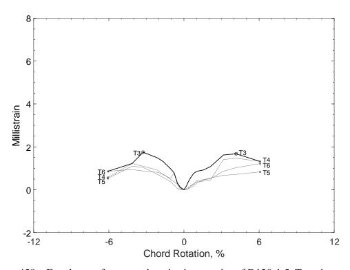
Figure 458 – Envelopes of measured strains in crossties of D120-1.5, T strain gauges
