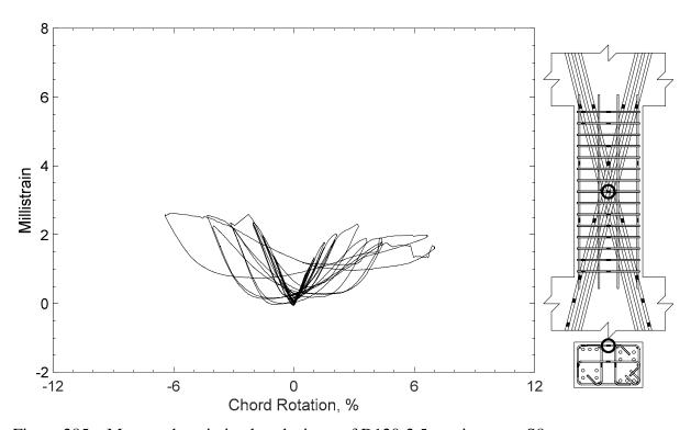
Figure 285 – Measured strain in closed stirrup of D120-2.5, strain gauge S8
