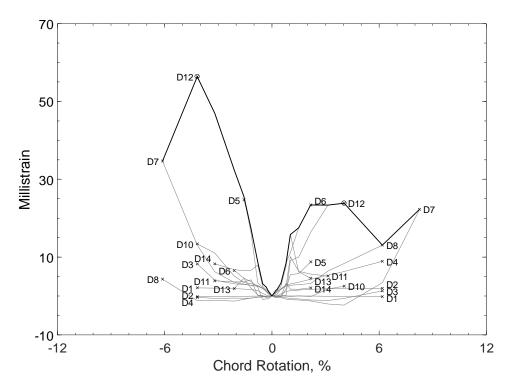
Figure 447 – Envelopes of measured strains in diagonal bars of D80-1.5, D strain gauges
