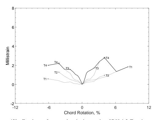
Figure 450 – Envelopes of measured strains in crossties of D80-1.5, T strain gauges
