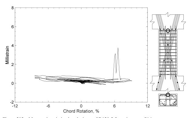
Figure 293 – Measured strain in closed stirrup of D120-2.5, strain gauge S16
