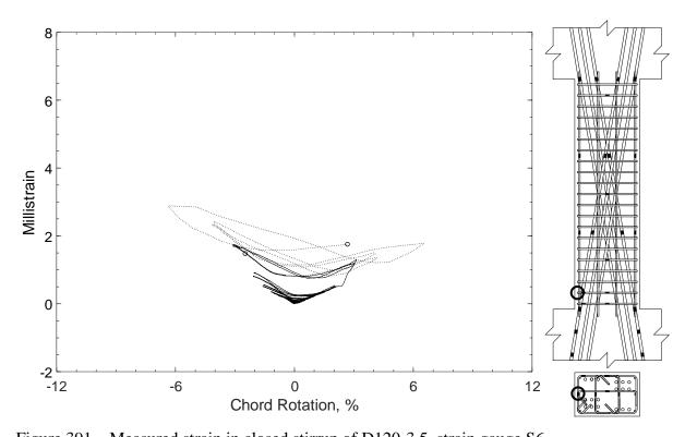
Figure 391 – Measured strain in closed stirrup of D120-3.5, strain gauge S6
