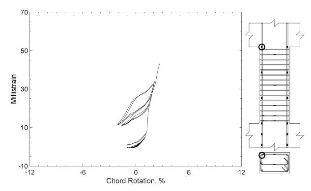
Figure 435 – Measured strain in parallel bar of P100-2.5, strain gauge P11
