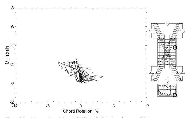
Figure 116 – Measured strain in parallel bar of D80-1.5, strain gauge H14
