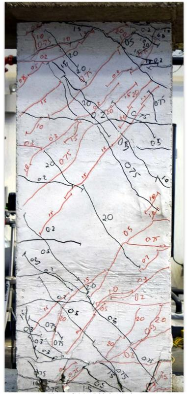
Figure C.94 – P80-2.5 during second cycle to 2% chord rotation
