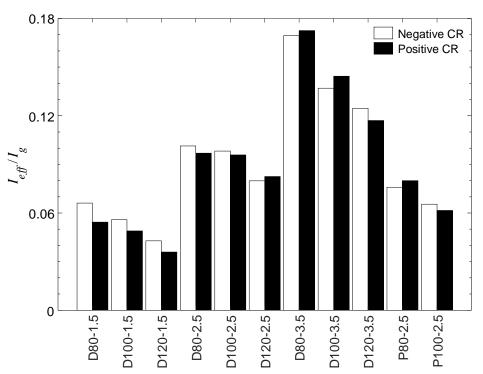
Figure 81 – Effective moment of inertia,  $I_{eff}$ , normalized by gross moment of inertia,  $I_g$
