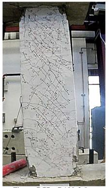
Figure C.77 – D100-3.5 at -4% chord rotation, second cycle
