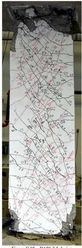
Figure C.85 – D120-3.5 during second cycle to 6% chord rotation
