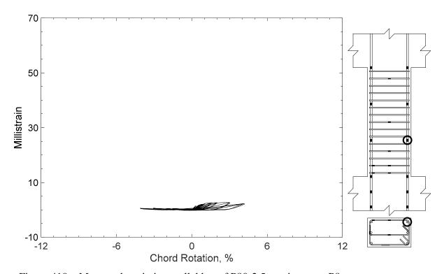
Figure 410 – Measured strain in parallel bar of P80-2.5, strain gauge P8
