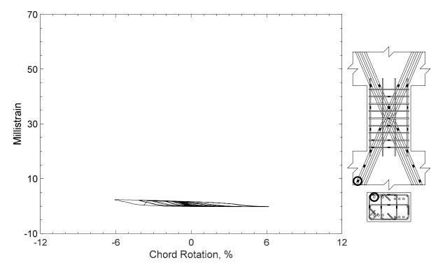
Figure 83 – Measured strain in diagonal bar of D80-1.5, strain gauge D1
