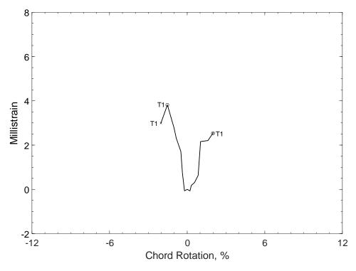
Figure 485 – Envelopes of measured strains in crossties of P80-2.5, T strain gauges
