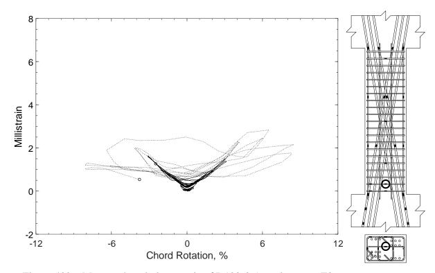
Figure 402 – Measured strain in crosstie of D120-3.5, strain gauge T3
