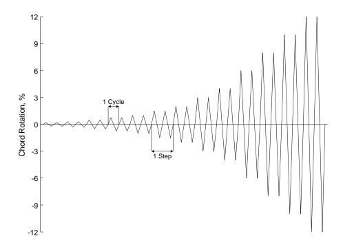
Figure 35 – Loading protocol<sup>a</sup>
