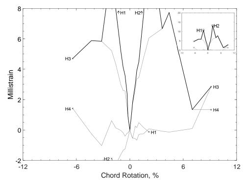
Figure 469 – Envelopes of measured strains in parallel bars of D120-2.5, H strain gauges
