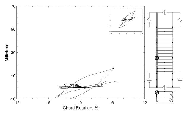
Figure 409 – Measured strain in parallel bar of P80-2.5, strain gauge P7
