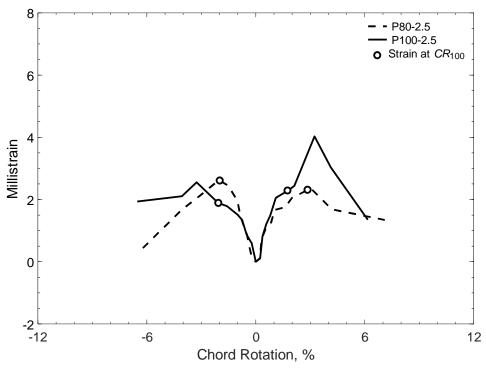
Figure 502 – Envelopes of measured strains in closed stirrups of P-type beams with an aspect ratio of 2.5, S strain gauges
