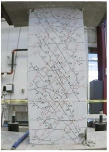
Figure C.53 – D120-2.5 at -2% chord rotation, second cycle
