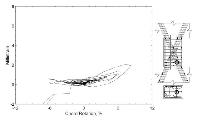
Figure 117 – Measured strain in crosstie of D80-1.5, strain gauge T1
