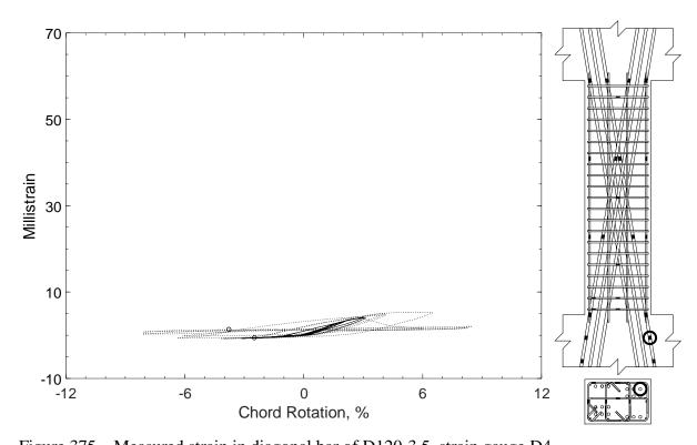
Figure 375 – Measured strain in diagonal bar of D120-3.5, strain gauge D4
