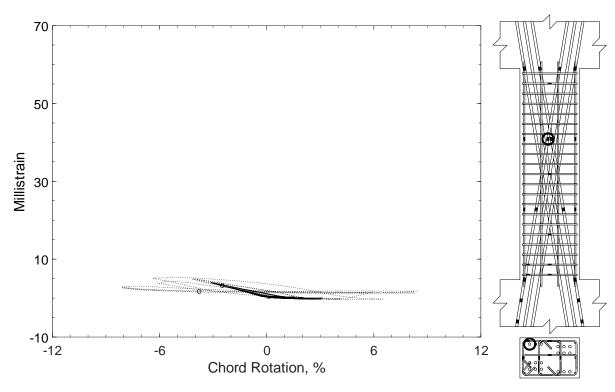
Figure 381 – Measured strain in diagonal bar of D120-3.5, strain gauge D10
