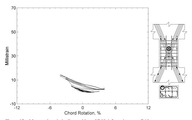
Figure 92 – Measured strain in diagonal bar of D80-1.5, strain gauge D10
