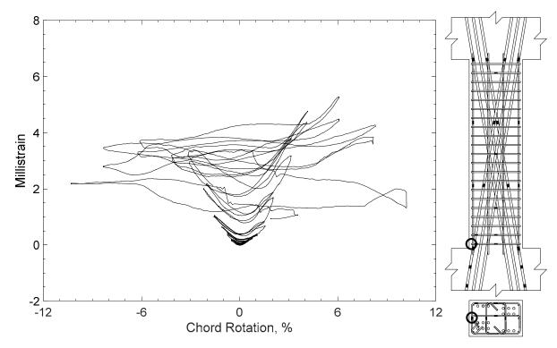
Figure 321 – Measured strain in closed stirrup of D80-3.5, strain gauge S3
