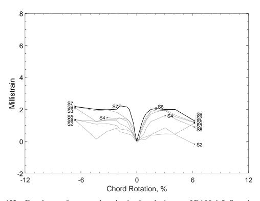
Figure 452 – Envelopes of measured strains in closed stirrups of D100-1.5, S strain gauges
