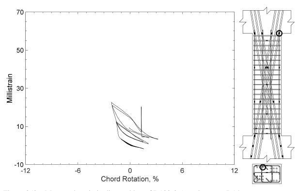
Figure 352 – Measured strain in diagonal bar of D100-3.5, strain gauge D14
