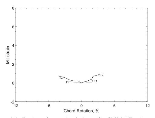
Figure 462 – Envelopes of measured strains in crossties of D80-2.5, T strain gauges
