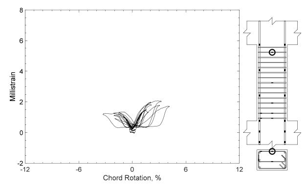
Figure 445 – Measured strain in closed stirrup of P100-2.5, strain gauge S9
