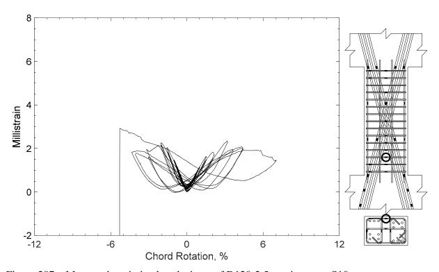
Figure 287 – Measured strain in closed stirrup of D120-2.5, strain gauge S10
