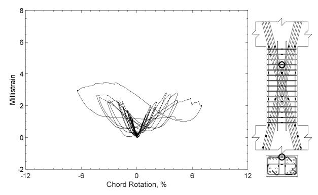
Figure 290 – Measured strain in closed stirrup of D120-2.5, strain gauge S13
