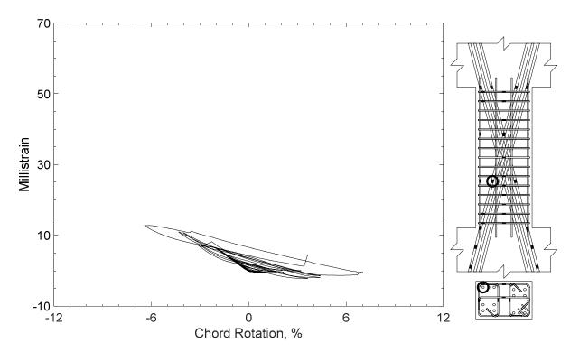
Figure 270 – Measured strain in diagonal bar of D120-2.5, strain gauge D7
