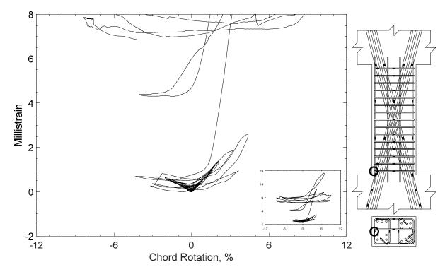
Figure 280 – Measured strain in closed stirrup of D120-2.5, strain gauge S3
