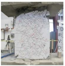
Figure C.25 – D120-1.5 at -4% chord rotation, second cycle
