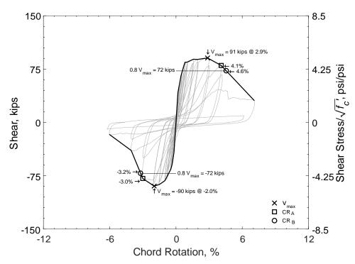
Figure 57 – Shear versus chord rotation envelope for P80-2.5 (1,000 psi = 6.89 MPa, 1 kip = 4.45 kN)
