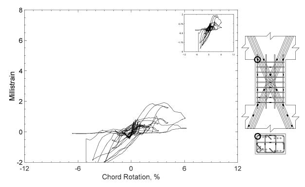
Figure 150 – Measured strain in parallel bar of D100-1.5, strain gauge H7
