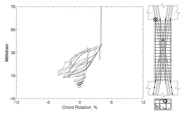
Figure 317 – Measured strain in diagonal bar of D80-3.5, strain gauge D13
