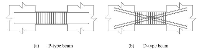
Figure 1 – Reinforcement layout types, parallel (P) and diagonal (D)
