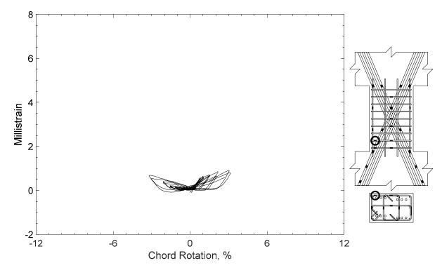
Figure 101 – Measured strain in closed stirrup of D80-1.5, strain gauge S5
