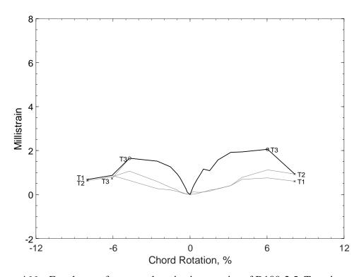
Figure 466 – Envelopes of measured strains in crossties of D100-2.5, T strain gauges
