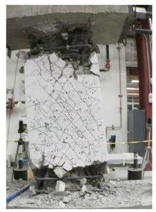
Figure C.59 – D120-2.5 at -8% chord rotation, second cycle
