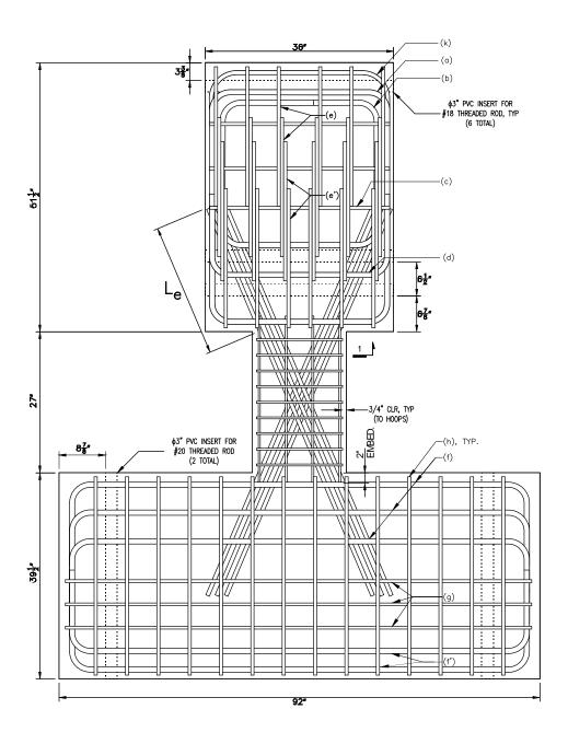
Figure 4 – Elevation view of D100-1.5 (1 in. = 25.4 mm)
