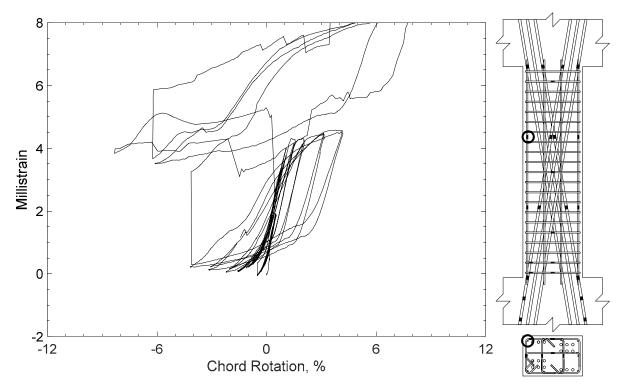
Figure 332 – Measured strain in parallel bar of D80-3.5, strain gauge H5
