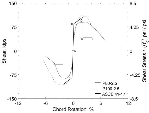
Figure 63 – Shear versus chord rotation envelopes for P80-2.5 and P100-2.5 (1,000 psi = 6.89 MPa, 1 kip = 4.45 kN)
