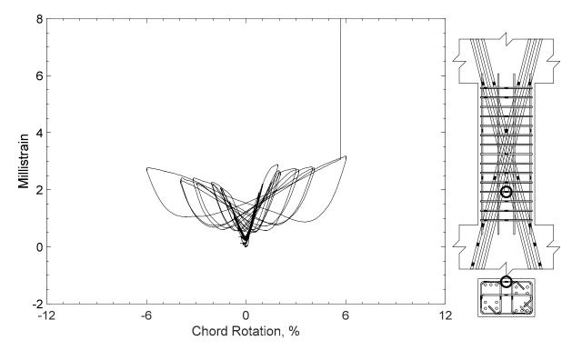
Figure 221 – Measured strain in closed stirrup of D80-2.5, strain gauge S7
