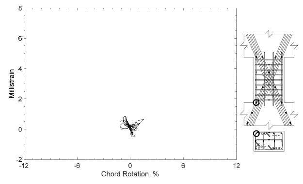
Figure 106 – Measured strain in parallel bar of D80-1.5, strain gauge H1
