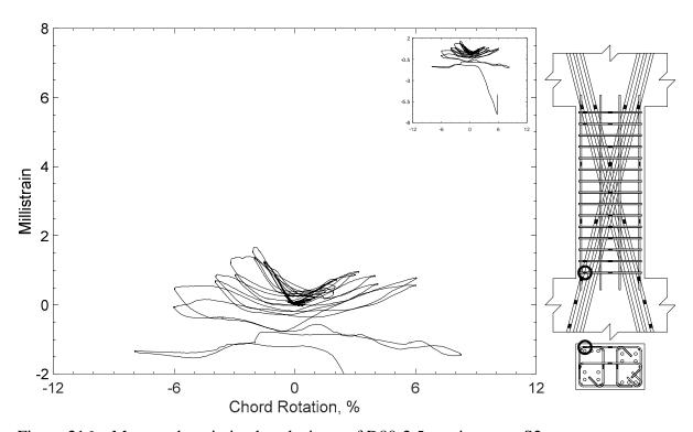
Figure 216 – Measured strain in closed stirrup of D80-2.5, strain gauge S2
