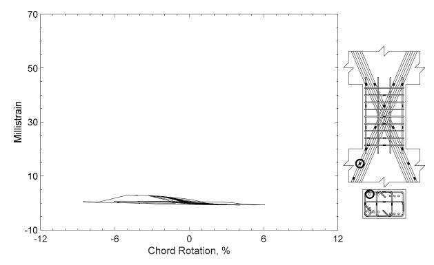
Figure 163 – Measured strain in diagonal bar of D120-1.5, strain gauge D3
