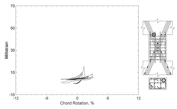
Figure 93 – Measured strain in diagonal bar of D80-1.5, strain gauge D11
