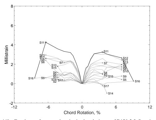
Figure 468 – Envelopes of measured strains in closed stirrups of D120-2.5, S strain gauges
