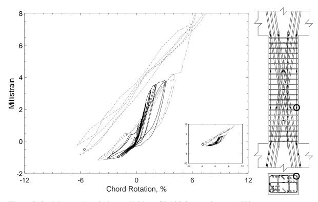
Figure 398 – Measured strain in parallel bar of D120-3.5, strain gauge H4
