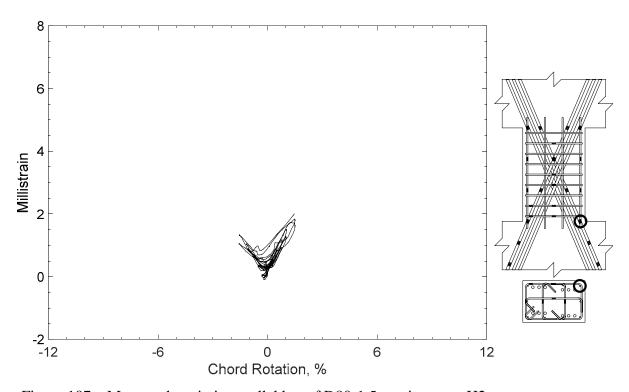
Figure 107 – Measured strain in parallel bar of D80-1.5, strain gauge H2
