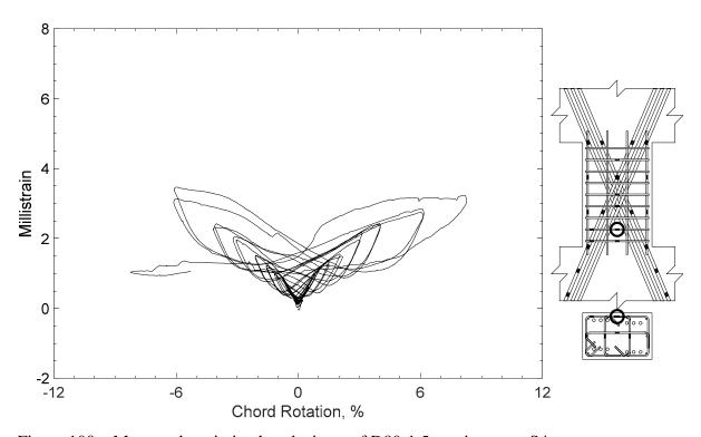
Figure 100 – Measured strain in closed stirrup of D80-1.5, strain gauge S4
