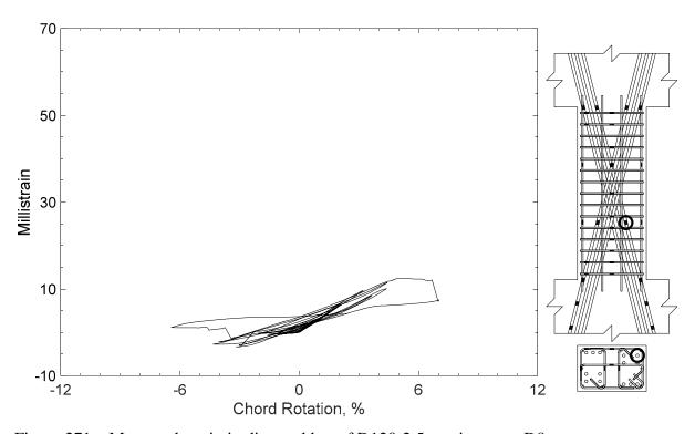
Figure 271 – Measured strain in diagonal bar of D120-2.5, strain gauge D8
