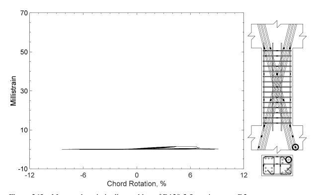
Figure 265 – Measured strain in diagonal bar of D120-2.5, strain gauge D2
