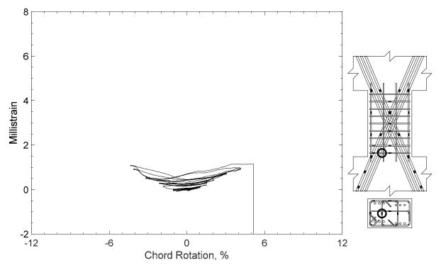
Figure 160 – Measured strain in crosstie of D100-1.5, strain gauge T5
