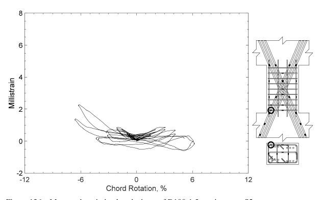
Figure 136 – Measured strain in closed stirrup of D100-1.5, strain gauge S2
