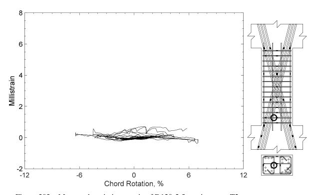
Figure 303 – Measured strain in crosstie of D120-2.5, strain gauge T2
