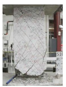
Figure C.107 – P100-2.5 at -4% chord rotation, second cycle
