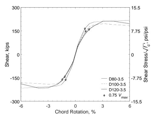
Figure 79 – Shear versus chord rotation envelopes for D80-3.5, D100-3.5, and D120-3.5
