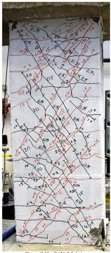
Figure C.50 – D120-2.5 during second cycle to 2% chord rotation
