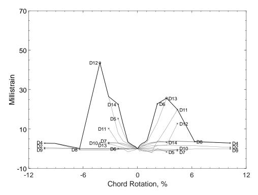
Figure 475 – Envelopes of measured strains in diagonal bars of D100-3.5, D strain gauges
