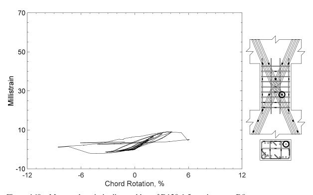
Figure 168 – Measured strain in diagonal bar of D120-1.5, strain gauge D8
