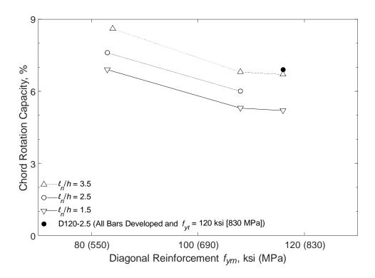
Figure 59 – Chord rotation capacity versus primary reinforcement grade for D-type coupling beams (1,000 psi = 6.89 MPa)
