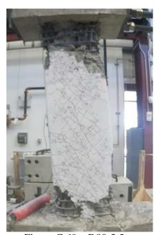
Figure C.69 – D80-3.5 at -8% chord rotation, second cycle
