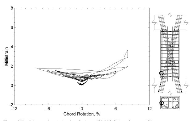
Figure 251 – Measured strain in closed stirrup of D100-2.5, strain gauge S6
