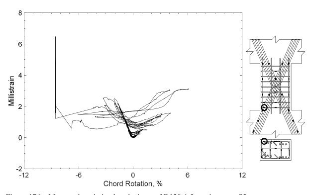
Figure 176 – Measured strain in closed stirrup of D120-1.5, strain gauge S2
