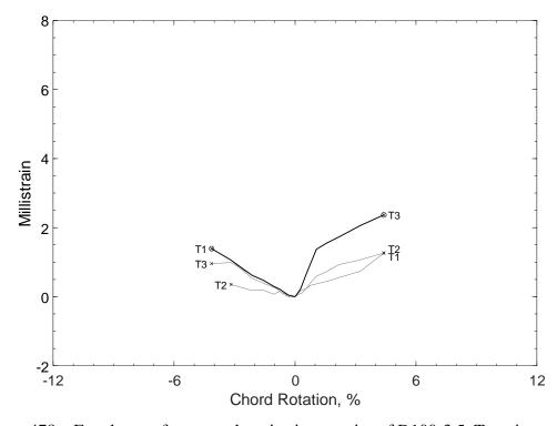
Figure 478 – Envelopes of measured strains in crossties of D100-3.5, T strain gauges
