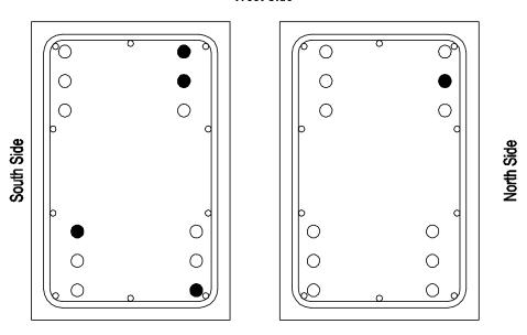
Section at Bottom Section at Top NOTES; Crossties and hooks not shown, Gray circle for bar necking and black circle for bar fracture.
