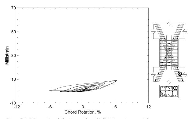
Figure 86 – Measured strain in diagonal bar of D80-1.5, strain gauge D4
