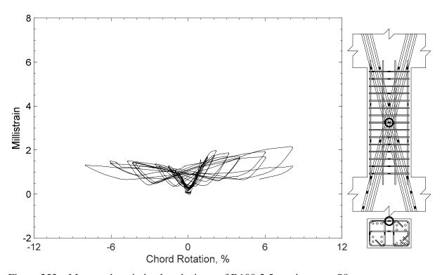
Figure 253 – Measured strain in closed stirrup of D100-2.5, strain gauge S8
