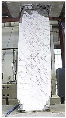
Figure C.90 – D120-3.5 at +6% chord rotation, second cycle
