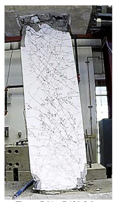
Figure C.91 – D120-3.5 at -6% chord rotation, second cycle
