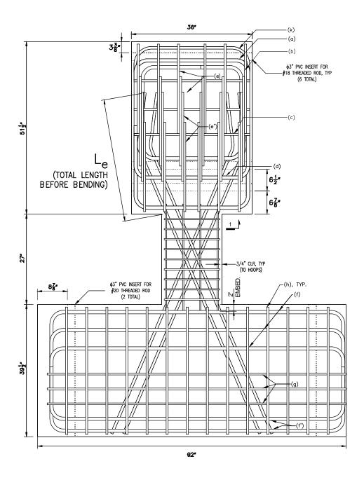
Figure 6 – Elevation view of D120-1.5 (1 in. = 25.4 mm)
