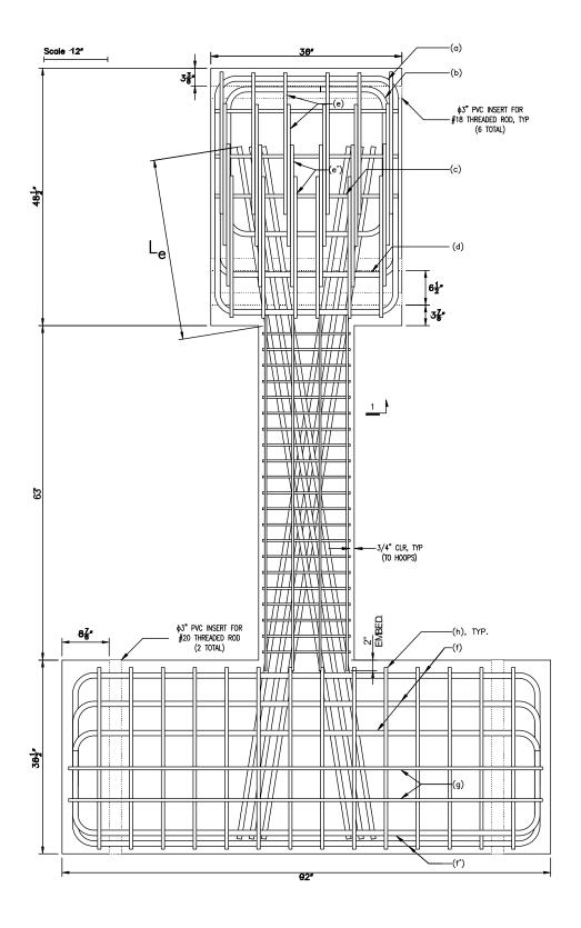
Figure 16 – Elevation view of D100-3.5 (1 in. = 25.4 mm)
