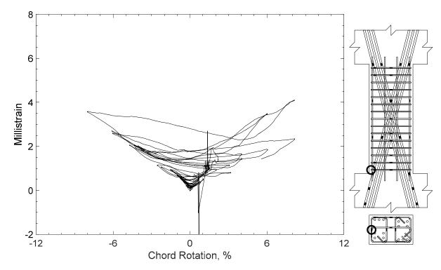
Figure 248 – Measured strain in closed stirrup of D100-2.5, strain gauge S3
