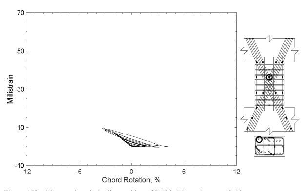
Figure 170 – Measured strain in diagonal bar of D120-1.5, strain gauge D10
