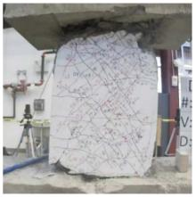
Figure C.27 – D120-1.5 at -6% chord rotation, first cycle
