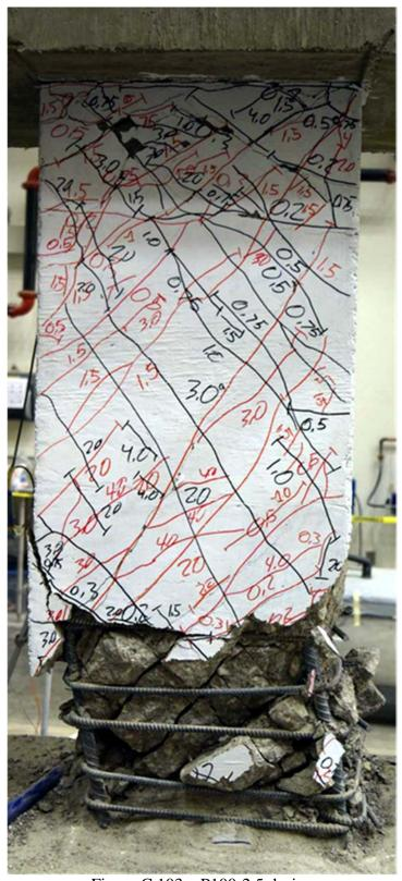
Figure C.103 – P100-2.5 during second cycle to 6% chord rotation
