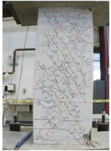
Figure C.52 – D120-2.5 at +2% chord rotation, second cycle
