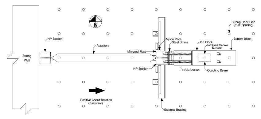
Figure 27 – Test setup, plan view
