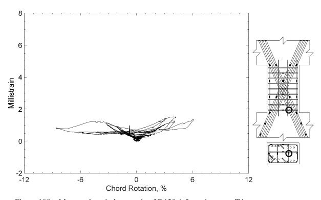
Figure 198 – Measured strain in crosstie of D120-1.5, strain gauge T4
