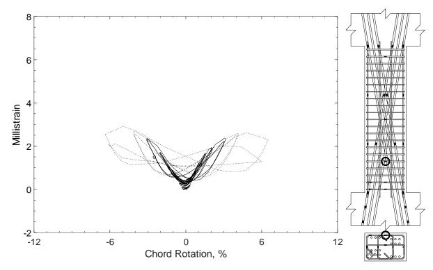
Figure 392 – Measured strain in closed stirrup of D120-3.5, strain gauge S7
