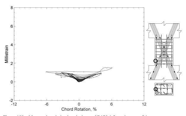
Figure 180 – Measured strain in closed stirrup of D120-1.5, strain gauge S6
