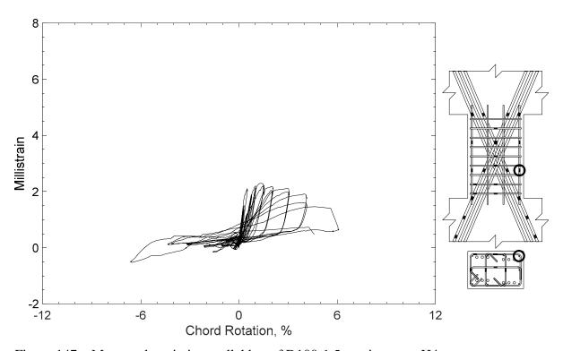
Figure 147 – Measured strain in parallel bar of D100-1.5, strain gauge H4
