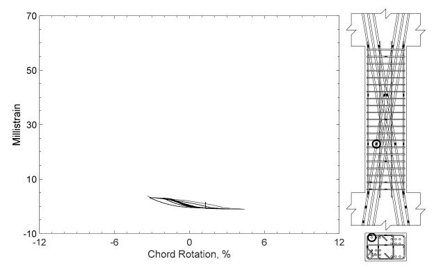
Figure 345 – Measured strain in diagonal bar of D100-3.5, strain gauge D7
