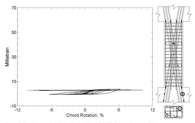
Figure 342 – Measured strain in diagonal bar of D100-3.5, strain gauge D4
