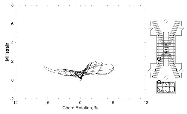
Figure 139 – Measured strain in closed stirrup of D100-1.5, strain gauge S5
