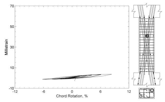
Figure 313 – Measured strain in diagonal bar of D80-3.5, strain gauge D9
