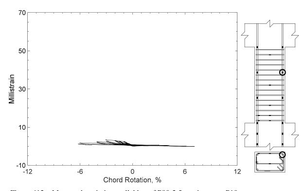
Figure 412 – Measured strain in parallel bar of P80-2.5, strain gauge P10
