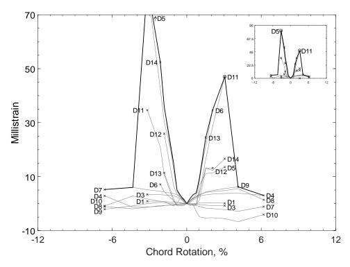
Figure 451 – Envelopes of measured strains in diagonal bars of D100-1.5, D strain gauges
