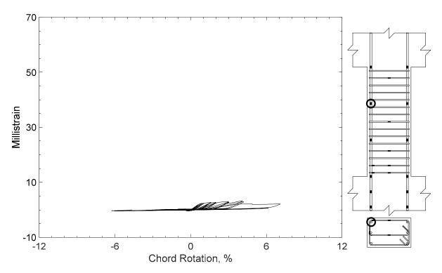
Figure 411 – Measured strain in parallel bar of P80-2.5, strain gauge P9
