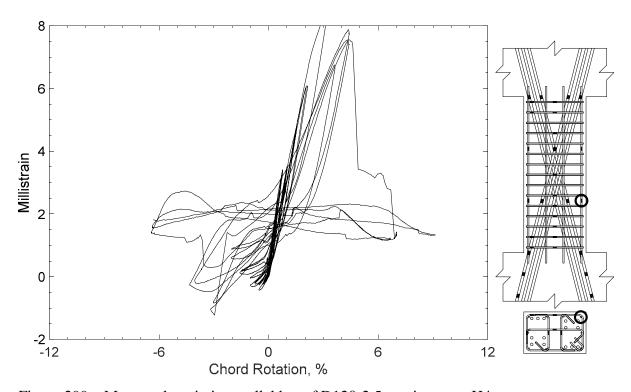
Figure 299 – Measured strain in parallel bar of D120-2.5, strain gauge H4
