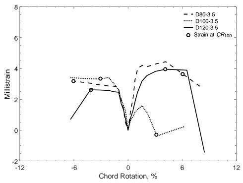
Figure 499 – Envelopes of measured strains in parallel bars of D-type beams with an aspect ratio of 3.5, H strain gauges
