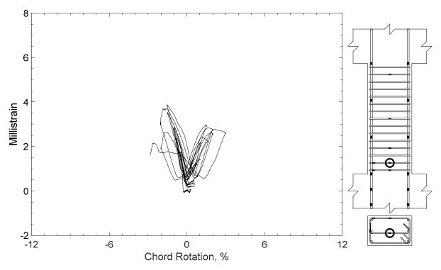
Figure 424 – Measured strain in crosstie of P80-2.5, strain gauge T1
