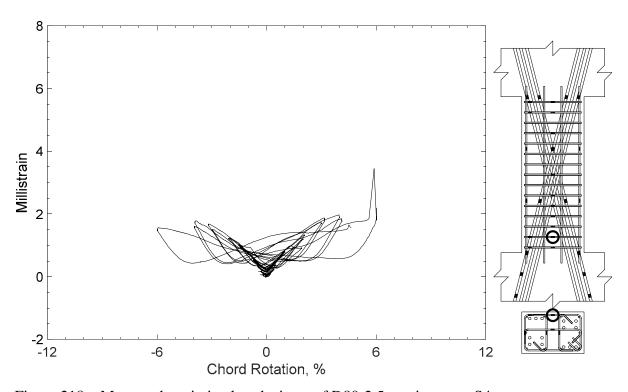
$Figure\ 218-Measured\ strain\ in\ closed\ stirrup\ of\ D80-2.5,\ strain\ gauge\ S4$
