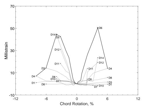
Figure 459 – Envelopes of measured strains in diagonal bars of D80-2.5, D strain gauges
