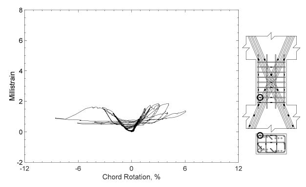
Figure 179 – Measured strain in closed stirrup of D120-1.5, strain gauge S5
