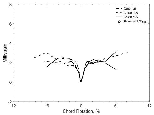
Figure 490 – Envelopes of measured strains in closed stirrups of D-type beams with an aspect ratio of 1.5, S strain gauges
