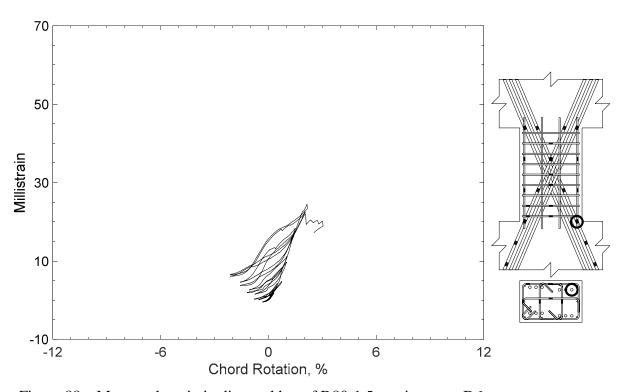
Figure 88 – Measured strain in diagonal bar of D80-1.5, strain gauge D6
