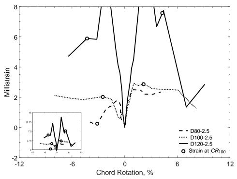
Figure 495 – Envelopes of measured strains in parallel bars of D-type beams with an aspect ratio of 2.5, H strain gauges
