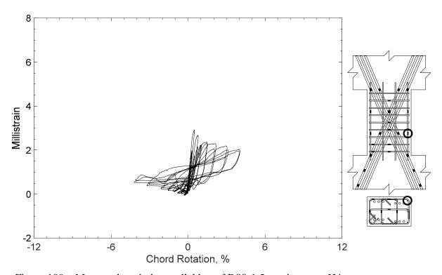
Figure 109 – Measured strain in parallel bar of D80-1.5, strain gauge H4
