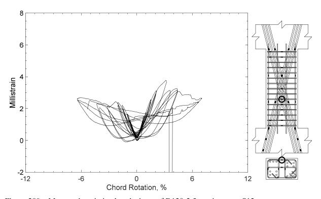
Figure 289 – Measured strain in closed stirrup of D120-2.5, strain gauge S12
