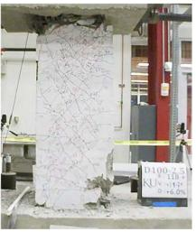
Figure C.47 – D100-2.5 at -6% chord rotation, second cycle
