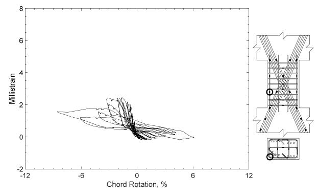
Figure 194 – Measured strain in parallel bar of D120-1.5, strain gauge H11
