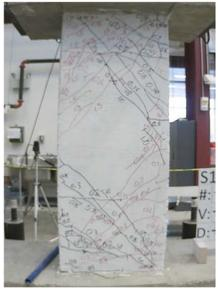
Figure C.104 – P100-2.5 at +2% chord rotation, second cycle
