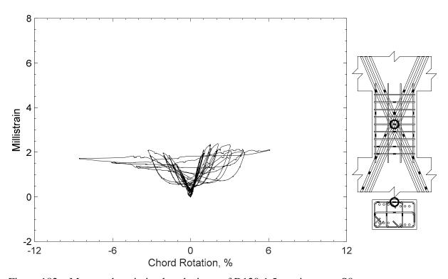
Figure 182 – Measured strain in closed stirrup of D120-1.5, strain gauge S8
