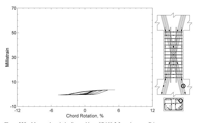
Figure 235 – Measured strain in diagonal bar of D100-2.5, strain gauge D4
