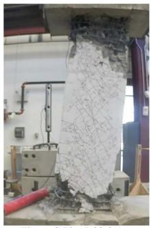
Figure C.70 – D80-3.5 at +10% chord rotation, first cycle
