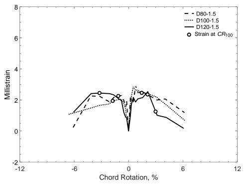
Figure 491 – Envelopes of measured strains in parallel bars of D-type beams with an aspect ratio of 1.5, H strain gauges
