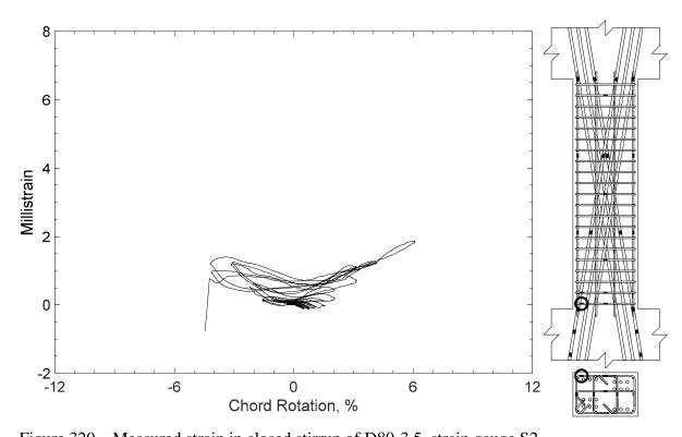
Figure 320 – Measured strain in closed stirrup of D80-3.5, strain gauge S2
