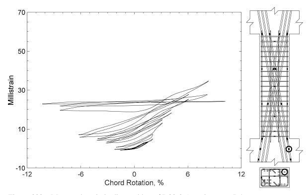
Figure 308 – Measured strain in diagonal bar of D80-3.5, strain gauge D4
