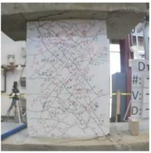
Figure C.23 – D120-1.5 at -2% chord rotation, second cycle
