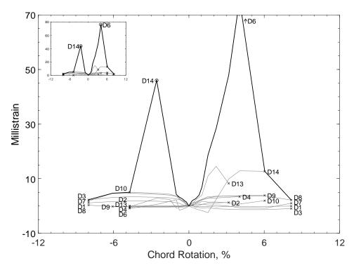
Figure 463 – Envelopes of measured strains in diagonal bars of D100-2.5, D strain gauges
