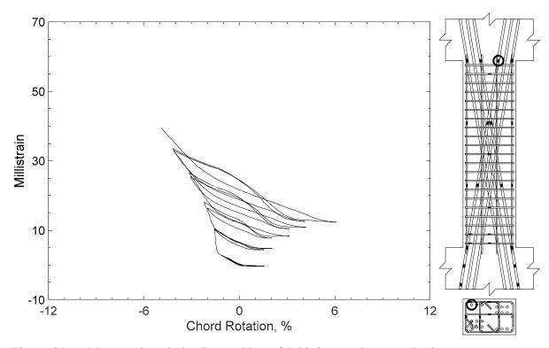
Figure 316 – Measured strain in diagonal bar of D80-3.5, strain gauge D12
