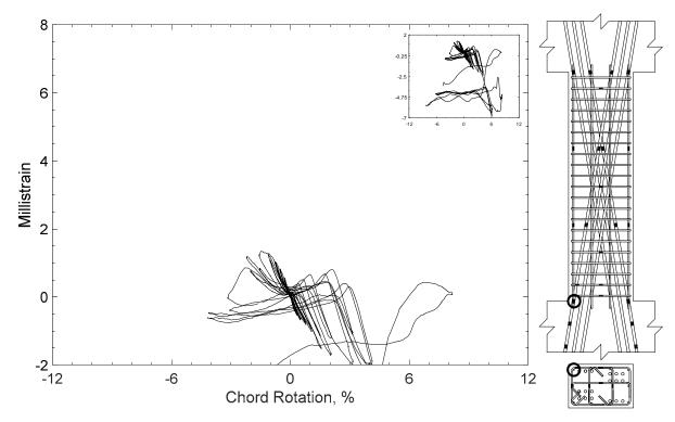
Figure 328 – Measured strain in parallel bar of D80-3.5, strain gauge H1
