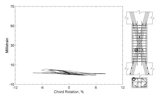
Figure 238 – Measured strain in diagonal bar of D100-2.5, strain gauge D7
