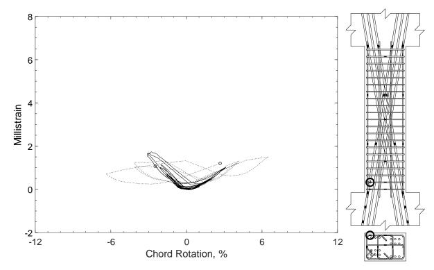
Figure 390 – Measured strain in closed stirrup of D120-3.5, strain gauge S5
