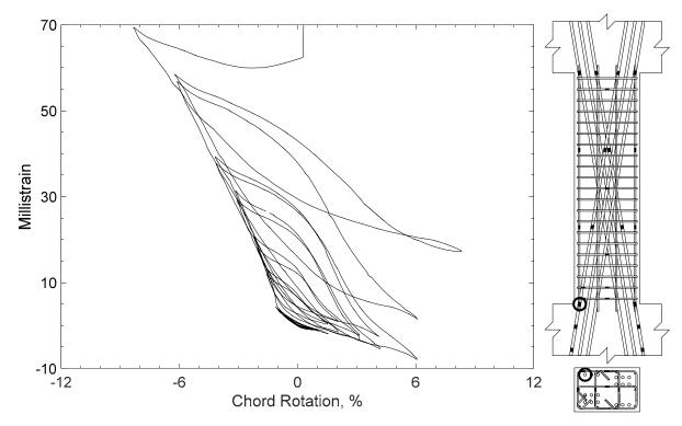
Figure 309 – Measured strain in diagonal bar of D80-3.5, strain gauge D5
