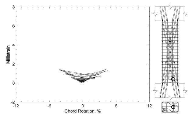
Figure 369 – Measured strain in crosstie of D100-3.5, strain gauge T1
