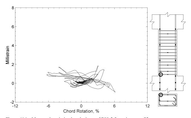
Figure 416 – Measured strain in closed stirrup of P80-2.5, strain gauge S2
