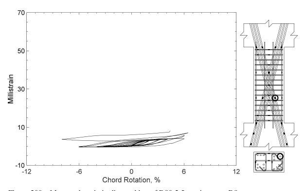
Figure 208 – Measured strain in diagonal bar of D80-2.5, strain gauge D8
