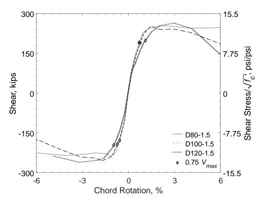
Figure 77 – Shear versus chord rotation envelopes for D80-1.5, D100-1.5, and D120-1.5
