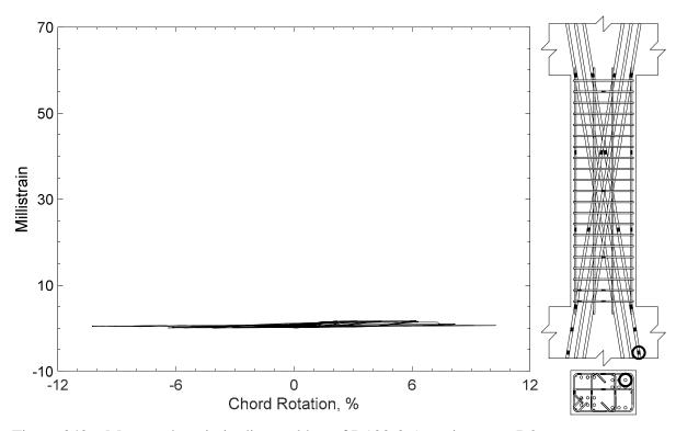
Figure 340 – Measured strain in diagonal bar of D100-3.5, strain gauge D2
