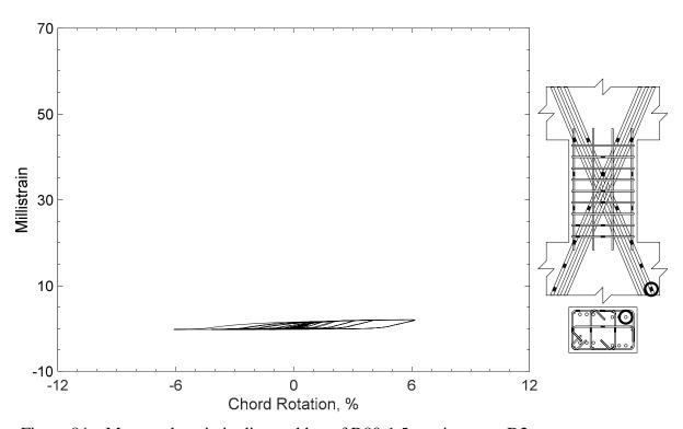
Figure 84 – Measured strain in diagonal bar of D80-1.5, strain gauge D2
