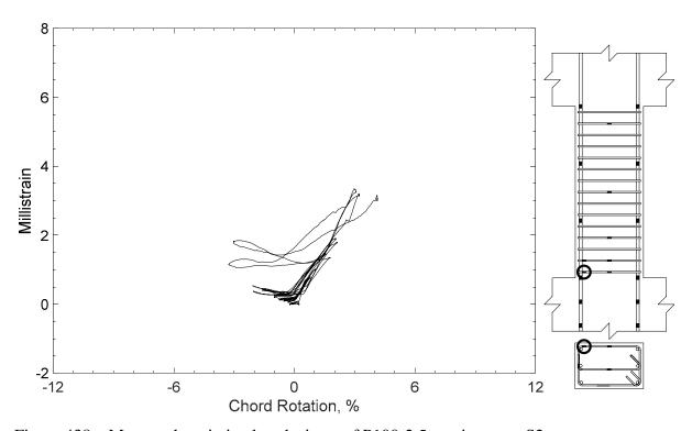
Figure 438 – Measured strain in closed stirrup of P100-2.5, strain gauge S2
