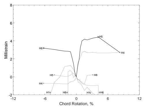
Figure 473 – Envelopes of measured strains in parallel bars of D80-3.5, H strain gauges
