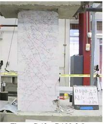
Figure C.43 – D100-2.5 at -2% chord rotation, second cycle
