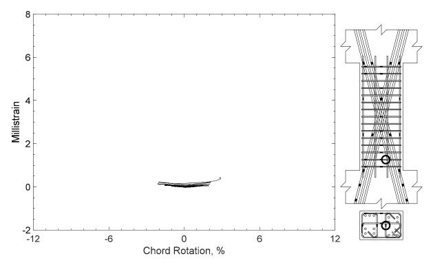
Figure 229 – Measured strain in crosstie of D80-2.5, strain gauge T1
