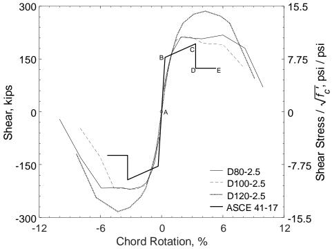
Figure 61 – Shear versus chord rotation envelopes for D80-2.5, D100-2.5, and D120-2.5 (1,000 psi = 6.89 MPa, 1 kip = 4.45 kN)
