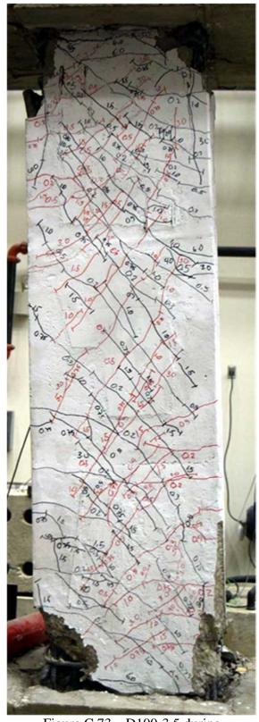
Figure C.73 – D100-3.5 during second cycle to 6% chord rotation
