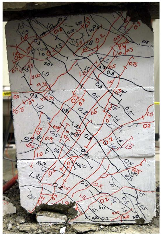
Figure C.12 – D100-1.5 during second cycle to 6% chord rotation
