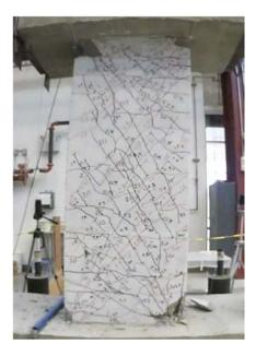
Figure C.54 – D120-2.5 at +4% chord rotation, second cycle
