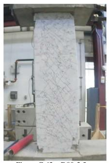
Figure C.63 – D80-3.5 at -2% chord rotation, second cycle
