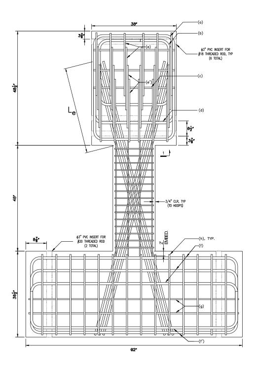
Figure 10 – Elevation view of D100-2.5 (1 in. = 25.4 mm)
