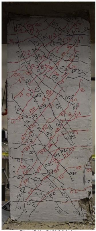
Figure C.40 – D100-2.5 during second cycle to 2% chord rotation
