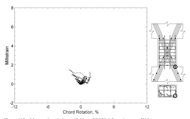
Figure 193 – Measured strain in parallel bar of D120-1.5, strain gauge H10
