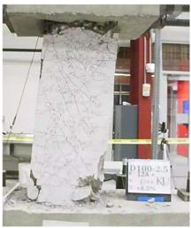
Figure C.48 – D100-2.5 at +8% chord rotation, first cycle
