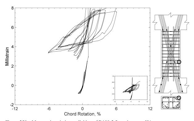
Figure 258 – Measured strain in parallel bar of D100-2.5, strain gauge H4
