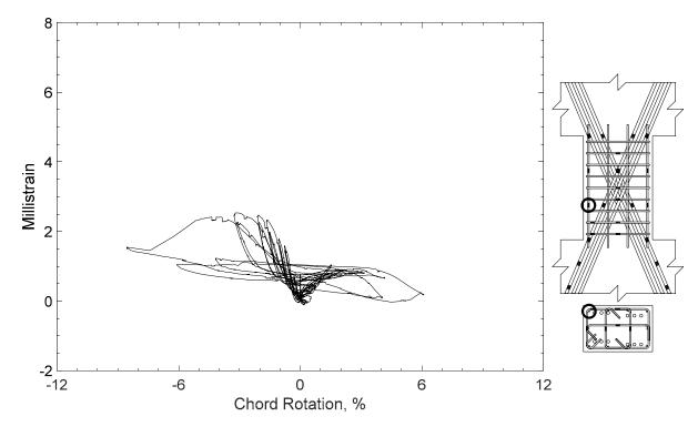
Figure 186 – Measured strain in parallel bar of D120-1.5, strain gauge H3
