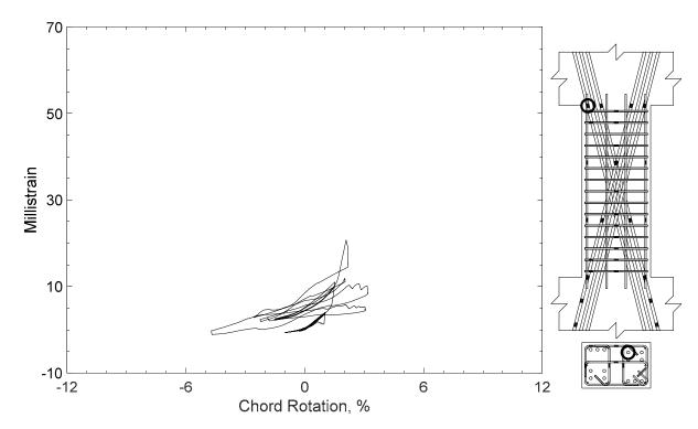
Figure 244 – Measured strain in diagonal bar of D100-2.5, strain gauge D13
