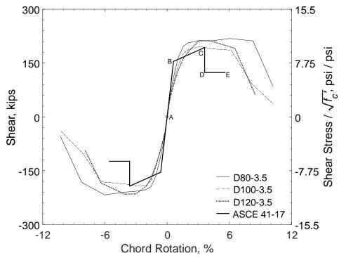
Figure 62 – Shear versus chord rotation envelopes for D80-3.5, D100-3.5, and D120-3.5 (1,000 psi = 6.89 MPa, 1 kip = 4.45 kN)
