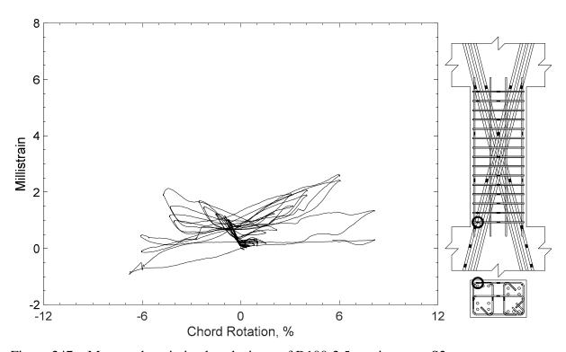
Figure 247 – Measured strain in closed stirrup of D100-2.5, strain gauge S2
