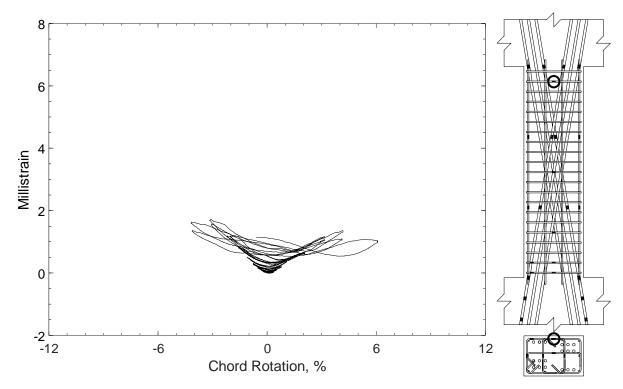
Figure 327 – Measured strain in closed stirrup of D80-3.5, strain gauge S9
