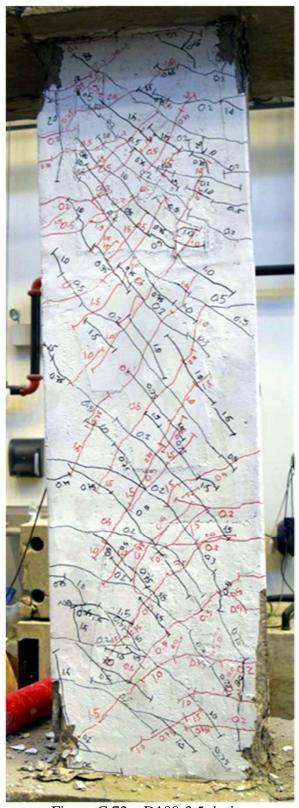
Figure C.72 – D100-3.5 during second cycle to 2% chord rotation
