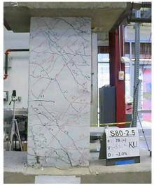
Figure C.96 – P80-2.5 at +2% chord rotation, second cycle
