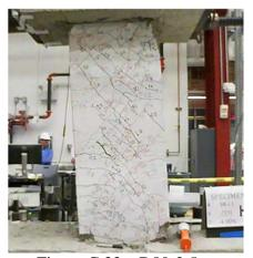
Figure C.33 – D80-2.5 at -4% chord rotation, second cycle
