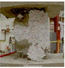
Figure C.8 – D80-1.5 at -6% chord rotation, second cycle
