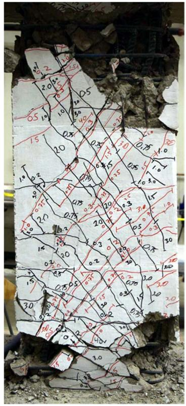
Figure C.51 – D120-2.5 during second cycle to 6% chord rotation
