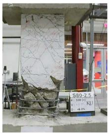
Figure C.100 – P80-2.5 at +6% chord rotation, second cycle
