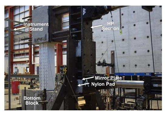
Figure 26 – Test setup, view from northwest
