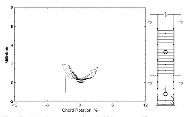
Figure 444 – Measured strain in closed stirrup of P100-2.5, strain gauge S8
