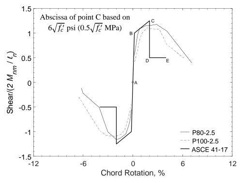
Figure 64 – Normalized shear versus chord rotation envelopes for P80-2.5 and P100-2.5 (1,000 psi = 6.89 MPa, 1 kip = 4.45 kN)
