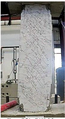
Figure C.76 – D100-3.5 at +4% chord rotation, second cycle
