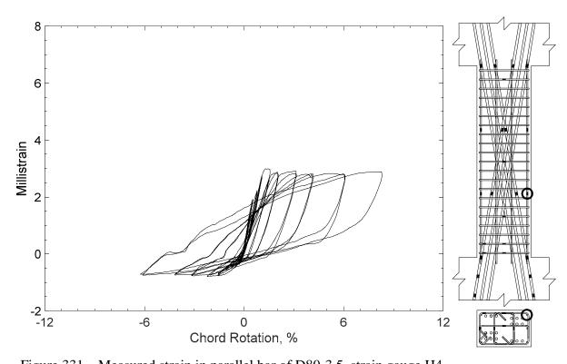
Figure 331 – Measured strain in parallel bar of D80-3.5, strain gauge H4
