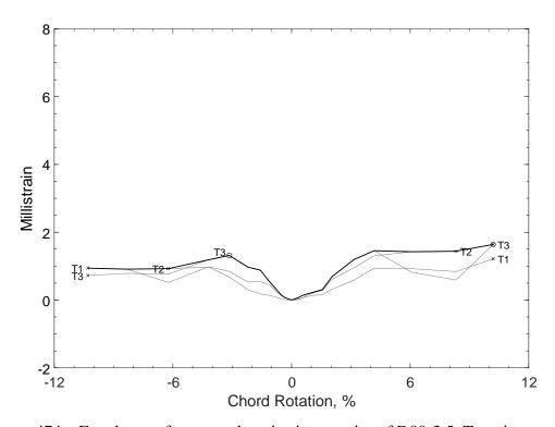
Figure 474 – Envelopes of measured strains in crossties of D80-3.5, T strain gauges
