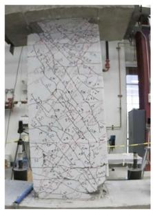
Figure C.55 – D120-2.5 at -4% chord rotation, second cycle
