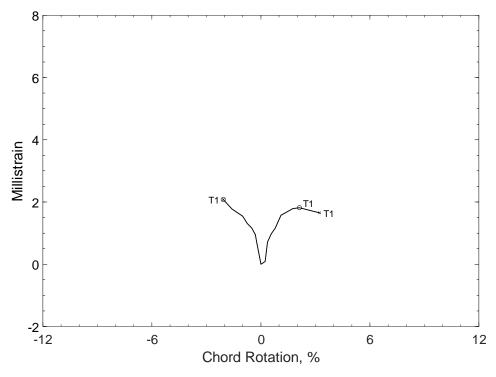
Figure 488 – Envelopes of measured strains in crossties of P100-2.5, T strain gauges
