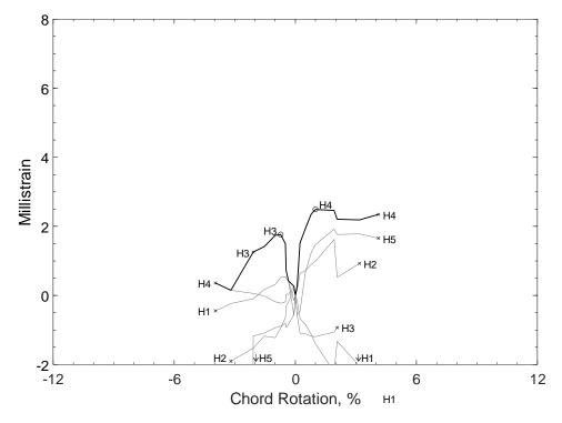
Figure 461 – Envelopes of measured strains in parallel bars of D80-2.5, H strain gauges
