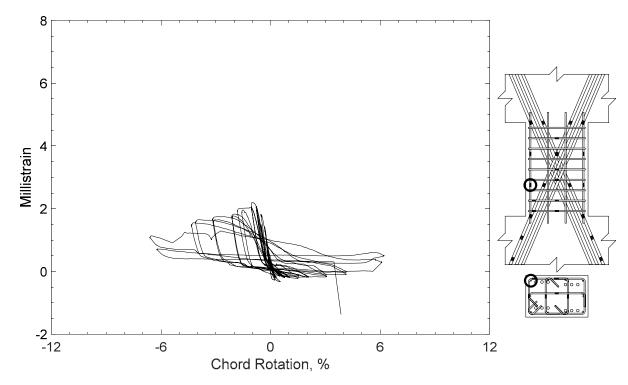
Figure 146 – Measured strain in parallel bar of D100-1.5, strain gauge H3
