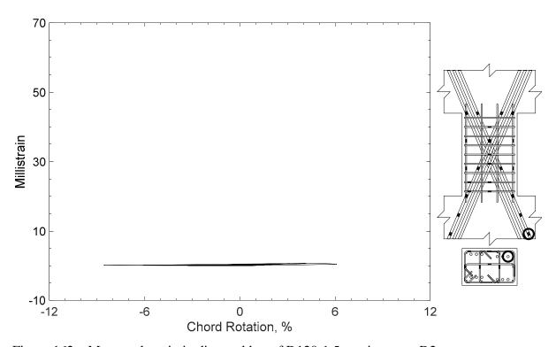
Figure 162 – Measured strain in diagonal bar of D120-1.5, strain gauge D2
