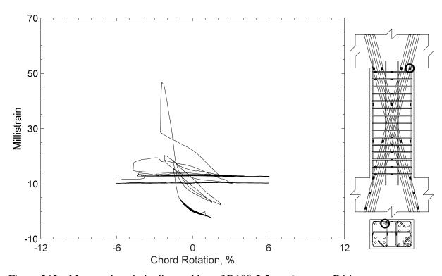
Figure 245 – Measured strain in diagonal bar of D100-2.5, strain gauge D14
