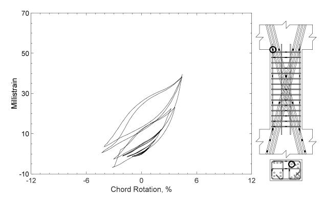
Figure 276 – Measured strain in diagonal bar of D120-2.5, strain gauge D13
