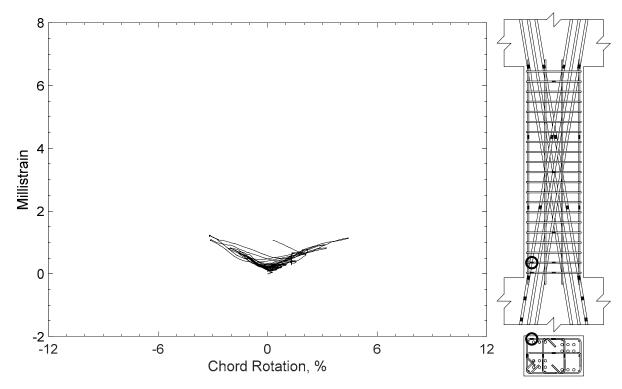
Figure 357 – Measured strain in closed stirrup of D100-3.5, strain gauge S5
