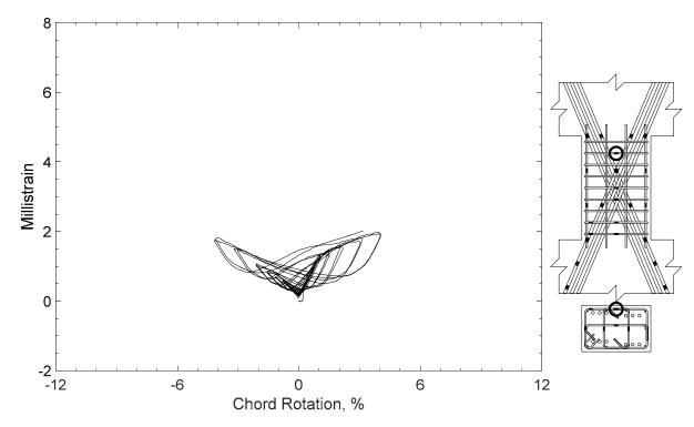
Figure 105 – Measured strain in closed stirrup of D80-1.5, strain gauge S9
