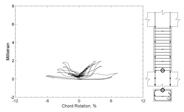
Figure 415 – Measured strain in closed stirrup of P80-2.5, strain gauge S1
