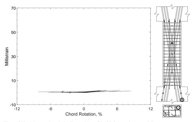
Figure 373 – Measured strain in diagonal bar of D120-3.5, strain gauge D2
