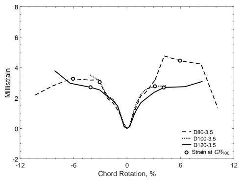
Figure 498 – Envelopes of measured strains in closed stirrups of D-type beams with an aspect ratio of 3.5, S strain gauges
