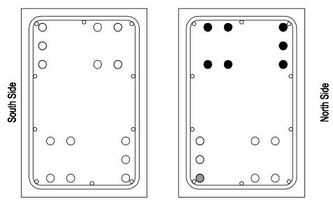
Section at Bottom Section at Top NOTES: Crossties and hooks not shown, Gray circle for bar necking and black circle for bar fracture.
