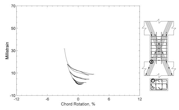
Figure 165 – Measured strain in diagonal bar of D120-1.5, strain gauge D5
