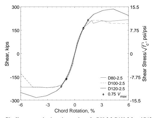
Figure 78 – Shear versus chord rotation envelopes for D80-2.5, D100-2.5, and D120-2.5
