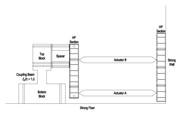
Figure 28 – Test setup for coupling beams with aspect ratio of 1.5<sup>a</sup>
