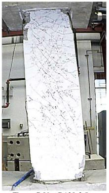
Figure C.89 – D120-3.5 at -4% chord rotation, second cycle
