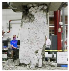
Figure C.38 – D80-2.5 at +10% chord rotation, first cycle
