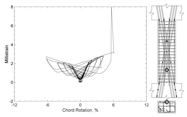
Figure 325 – Measured strain in closed stirrup of D80-3.5, strain gauge S7
