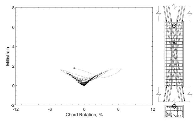
Figure 394 – Measured strain in closed stirrup of D120-3.5, strain gauge S9
