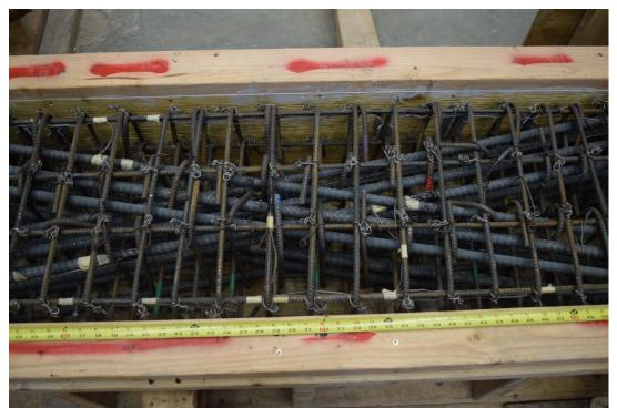
$Figure\ B.3-Coupling\ beam\ reinforcement,\ D120-3.5$
