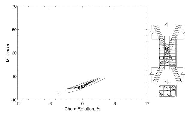
Figure 169 – Measured strain in diagonal bar of D120-1.5, strain gauge D9
