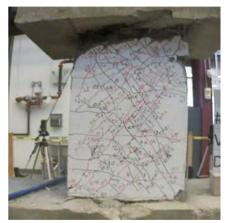
Figure C.24 – D120-1.5 at +4% chord rotation, second cycle
