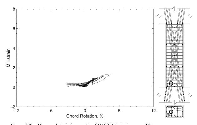
Figure 370 – Measured strain in crosstie of D100-3.5, strain gauge T2
