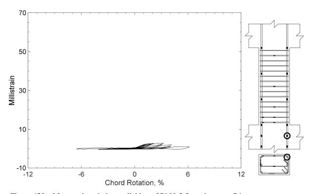
Figure 428 – Measured strain in parallel bar of P100-2.5, strain gauge P4
