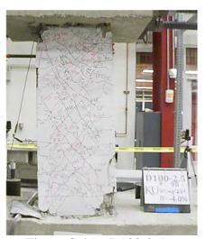
Figure C.45 – D100-2.5 at -4% chord rotation, second cycle
