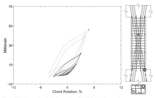
Figure 377 – Measured strain in diagonal bar of D120-3.5, strain gauge D6
