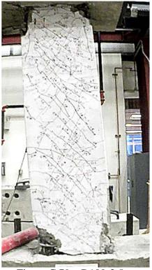
Figure C.79 – D100-3.5 at -6% chord rotation, second cycle
