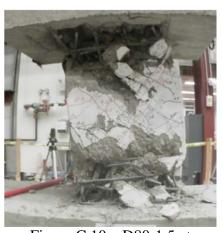
Figure C.10 – D80-1.5 at -8% chord rotation, first cycle
