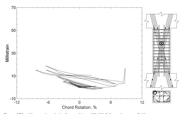
Figure 273 – Measured strain in diagonal bar of D120-2.5, strain gauge D10
