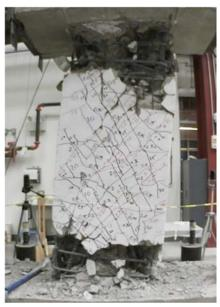
Figure C.58 – D120-2.5 at +8% chord rotation, second cycle
