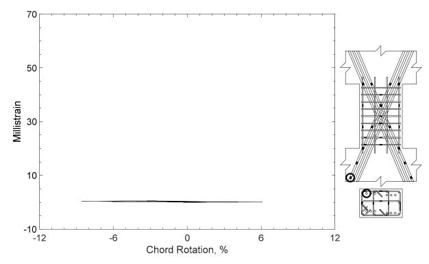
Figure 161 – Measured strain in diagonal bar of D120-1.5, strain gauge D1
