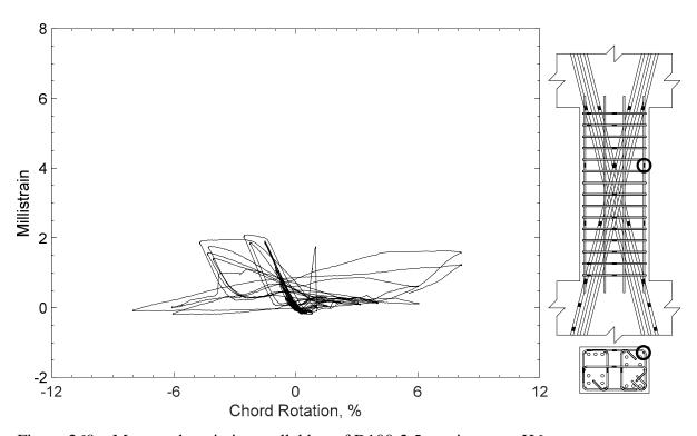
Figure 260 – Measured strain in parallel bar of D100-2.5, strain gauge H6
