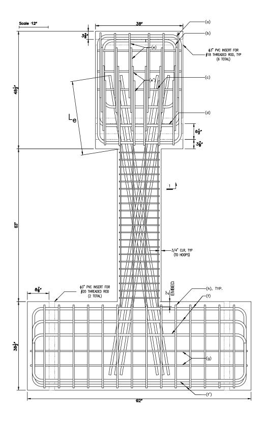
Figure 14 - Elevation view of D80-3.5 (1 in. = 25.4 mm)
