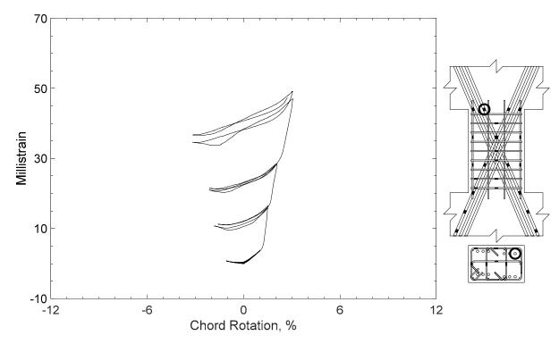
Figure 131 – Measured strain in diagonal bar of D100-1.5, strain gauge D11
