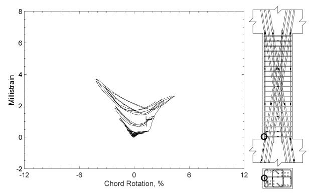
Figure 355 – Measured strain in closed stirrup of D100-3.5, strain gauge S3
