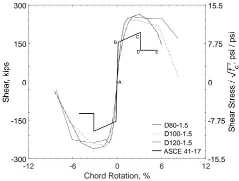
Figure 60 – Shear versus chord rotation envelopes for D80-1.5, D100-1.5, and D120-1.5 (1,000 psi = 6.89 MPa, 1 kip = 4.45 kN)
