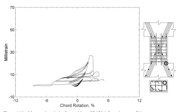
Figure 166 – Measured strain in diagonal bar of D120-1.5, strain gauge D6
