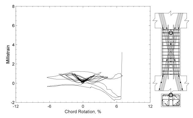
Figure 286 – Measured strain in closed stirrup of D120-2.5, strain gauge S9
