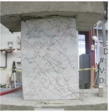
Figure C.4 – D80-1.5 at -2% chord rotation, second cycle
