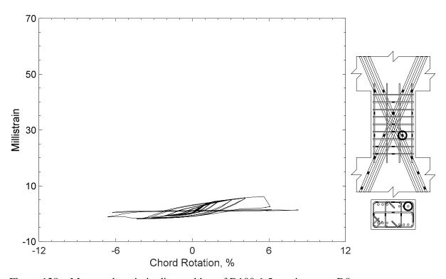
Figure 128 – Measured strain in diagonal bar of D100-1.5, strain gauge D8
