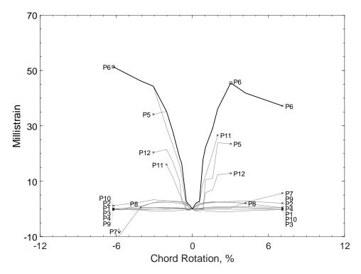
Figure 483 – Envelopes of measured strains in parallel bars of P80-2.5, P strain gauges
