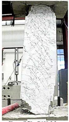
Figure C.78 – D100-3.5 at +6% chord rotation, second cycle
