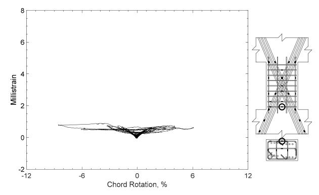
Figure 175 – Measured strain in closed stirrup of D120-1.5, strain gauge S1
