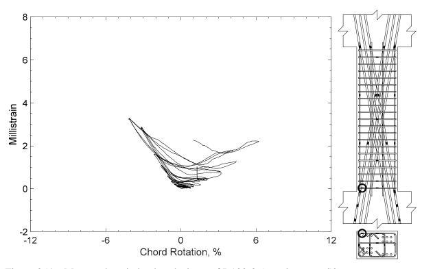
Figure 354 – Measured strain in closed stirrup of D100-3.5, strain gauge S2
