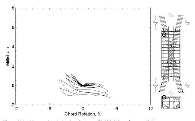
Figure 291 – Measured strain in closed stirrup of D120-2.5, strain gauge S14
