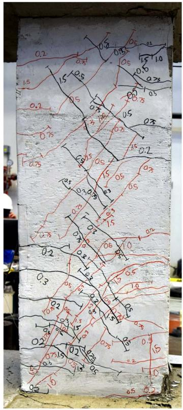
Figure C.28 – D80-2.5 during second cycle to 2% chord rotation
