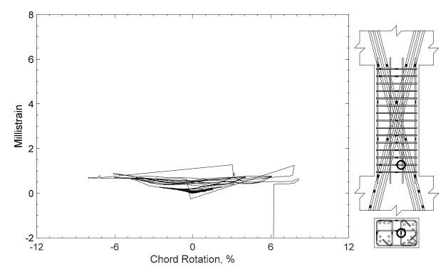
Figure 261 – Measured strain in crosstie of D100-2.5, strain gauge T1
