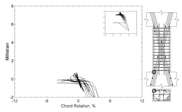
Figure 224 – Measured strain in parallel bar of D80-2.5, strain gauge H1
