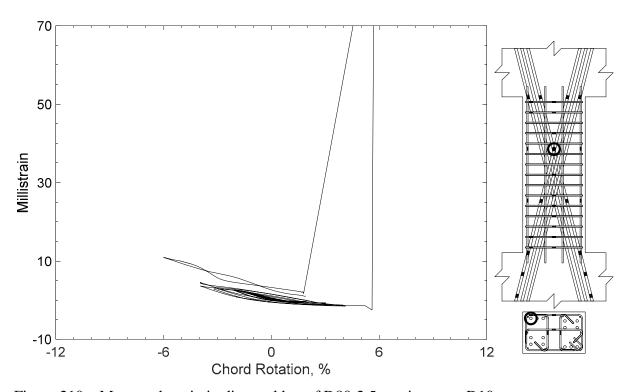
Figure 210 – Measured strain in diagonal bar of D80-2.5, strain gauge D10
