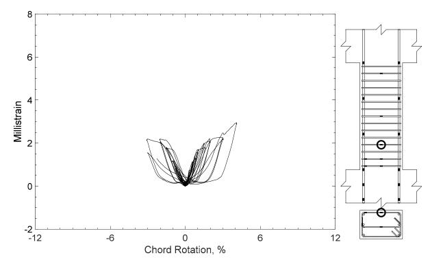
Figure 421 – Measured strain in closed stirrup of P80-2.5, strain gauge S7
