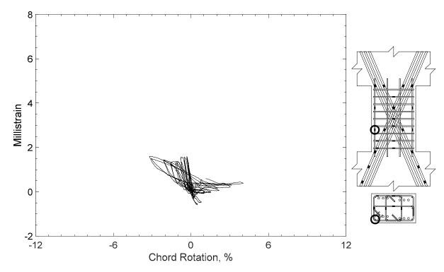
Figure 113 – Measured strain in parallel bar of D80-1.5, strain gauge H11
