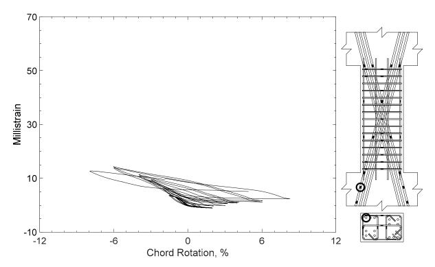
Figure 203 – Measured strain in diagonal bar of D80-2.5, strain gauge D3
