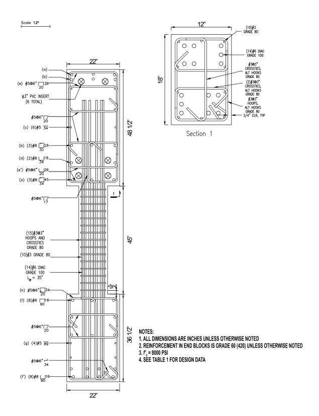
Figure 11 – Reinforcement details of D100-2.5 (1 in. = 25.4 mm, 1 ksi = 1,000 psi = 6.89 MPa)
