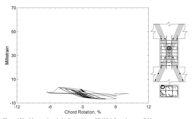
Figure 130 – Measured strain in diagonal bar of D100-1.5, strain gauge D10
