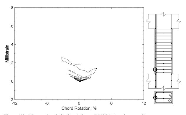
Figure 442 – Measured strain in closed stirrup of P100-2.5, strain gauge S6
