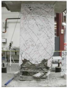
Figure C.108 – P100-2.5 at +6% chord rotation, second cycle
