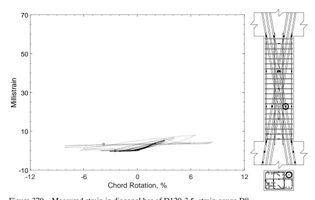
Figure 379 – Measured strain in diagonal bar of D120-3.5, strain gauge D8
