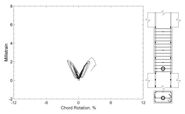
Figure 446 – Measured strain in crosstie of P100-2.5, strain gauge T1
