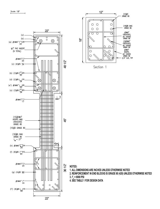
Figure 9 – Reinforcement details of D80-2.5 (1 in. = 25.4 mm, 1 ksi = 1,000 psi = 6.89 MPa)
