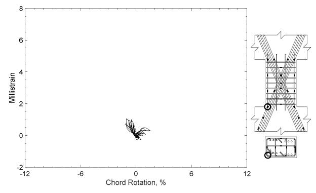
Figure 152 – Measured strain in parallel bar of D100-1.5, strain gauge H9
