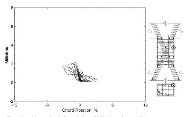
Figure 111 – Measured strain in parallel bar of D80-1.5, strain gauge H6
