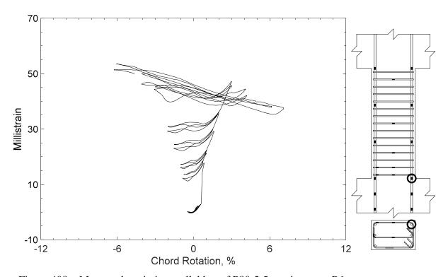
Figure 408 – Measured strain in parallel bar of P80-2.5, strain gauge P6
