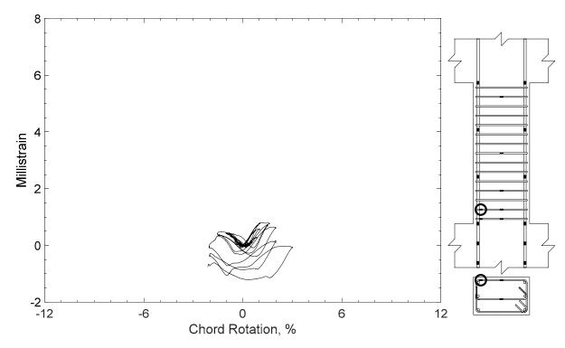
Figure 419 – Measured strain in closed stirrup of P80-2.5, strain gauge S5
