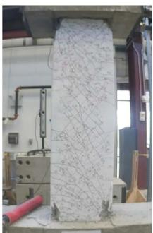
Figure C.64 – D80-3.5 at +4% chord rotation, second cycle
