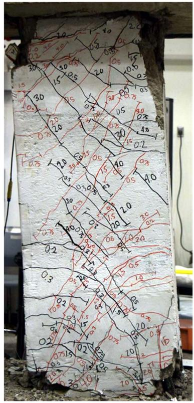
Figure C.29 – D80-2.5 during second cycle to 6% chord rotation
