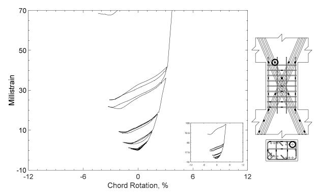
Figure 171 – Measured strain in diagonal bar of D120-1.5, strain gauge D11
