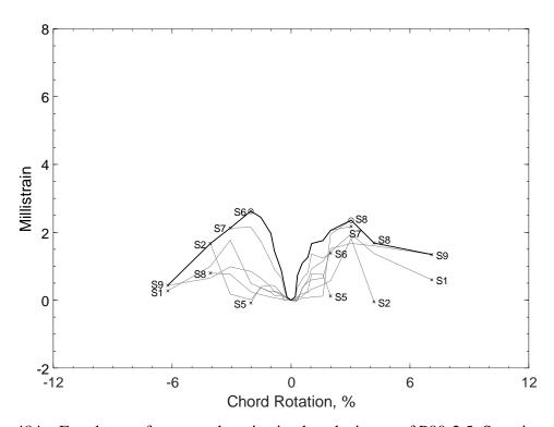
Figure 484 – Envelopes of measured strains in closed stirrups of P80-2.5, S strain gauges
