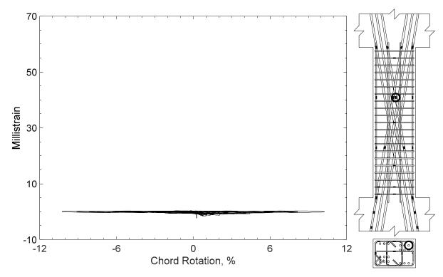
Figure 347 – Measured strain in diagonal bar of D100-3.5, strain gauge D9
