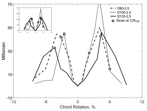
Figure 493 – Envelopes of measured strains in diagonal bars of D-type beams with an aspect ratio of 2.5, D strain gauges
