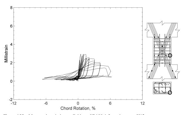
Figure 155 – Measured strain in parallel bar of D100-1.5, strain gauge H12
