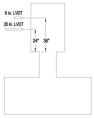
Figure 31 – LVDT locations (1 in. = 25.4 mm)
