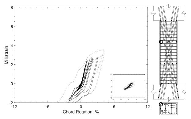
Figure 399 – Measured strain in parallel bar of D120-3.5, strain gauge H5
