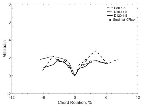
Figure 492 – Envelopes of measured strains in crossties of D-type beams with an aspect ratio of 1.5, T strain gauges
