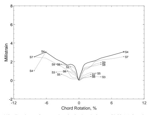
Figure 448 – Envelopes of measured strains in closed stirrups of D80-1.5, S strain gauges
