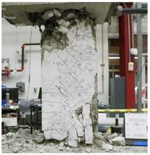
Figure C.39 – D80-2.5 at -10% chord rotation, first cycle
