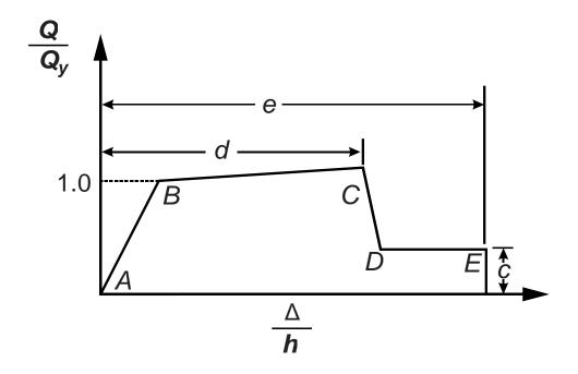
Figure 65 – Generalized force-deformation relationship for diagonally-reinforced concrete coupling beams (taken from ASCE 41-17 Figure  $10-1(b)^{[4]}$ )
