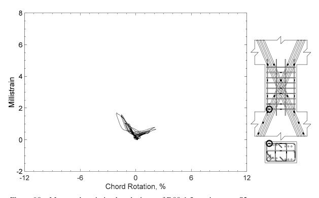
Figure 98 – Measured strain in closed stirrup of D80-1.5, strain gauge S2
