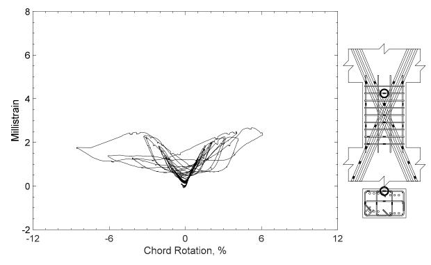
Figure 183 – Measured strain in closed stirrup of D120-1.5, strain gauge S9
