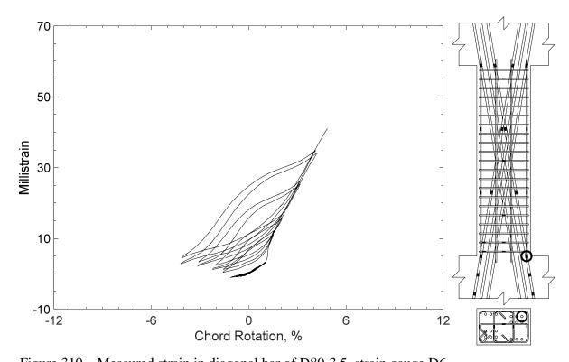
Figure 310 – Measured strain in diagonal bar of D80-3.5, strain gauge D6
