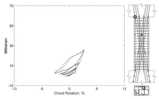
Figure 351 – Measured strain in diagonal bar of D100-3.5, strain gauge D13
