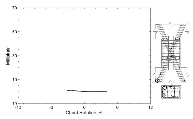
Figure 121 – Measured strain in diagonal bar of D100-1.5, strain gauge D1
