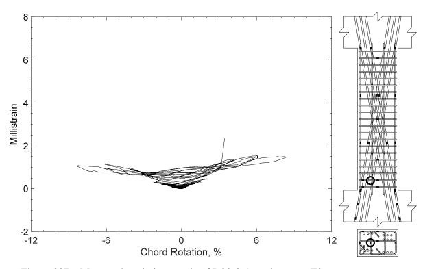
Figure 337 – Measured strain in crosstie of D80-3.5, strain gauge T2
