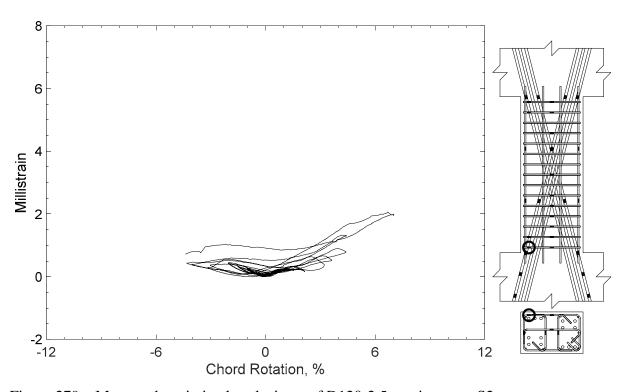
Figure 279 – Measured strain in closed stirrup of D120-2.5, strain gauge S2
