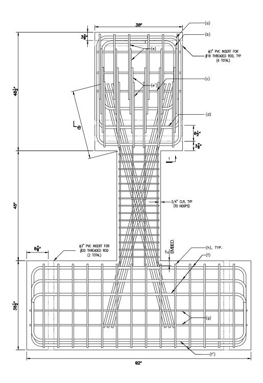
Figure 8 – Elevation view of D80-2.5 (1 in. = 25.4 mm)
