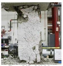
Figure C.37 – D80-2.5 at -8% chord rotation, second cycle
