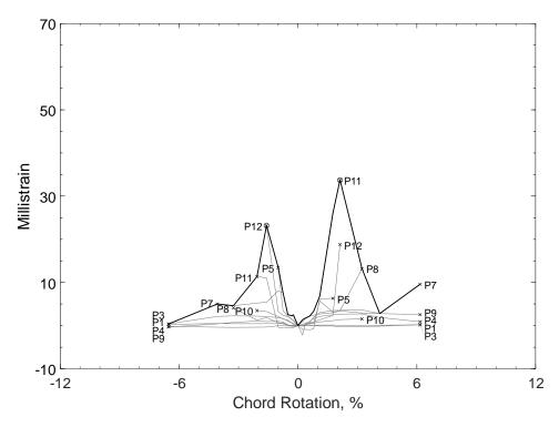
Figure 486 – Envelopes of measured strains in parallel bars of P100-2.5, P strain gauges
