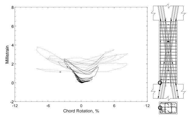
Figure 388 – Measured strain in closed stirrup of D120-3.5, strain gauge S3
