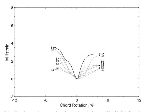
Figure 476 – Envelopes of measured strains in closed stirrups of D100-3.5, S strain gauges
