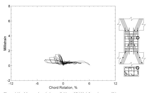
Figure 149 – Measured strain in parallel bar of D100-1.5, strain gauge H6
