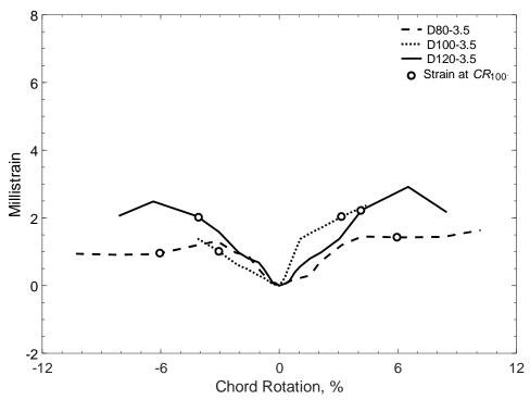
Figure 500 – Envelopes of measured strains in crossties of D-type beams with an aspect ratio of 3.5, T strain gauges
