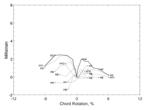
Figure 457 – Envelopes of measured strains in parallel bars of D120-1.5, H strain gauges
