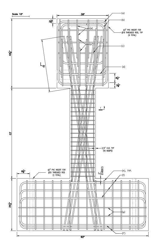
Figure 18 – Elevation view of D120-3.5 (1 in. = 25.4 mm)
