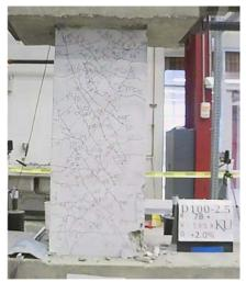
Figure C.42 – D100-2.5 at +2% chord rotation, second cycle
