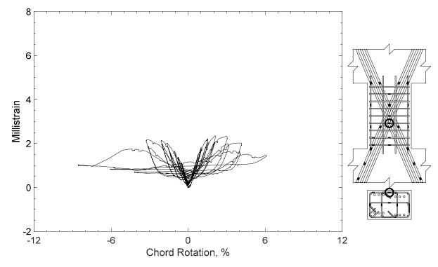
Figure 181 – Measured strain in closed stirrup of D120-1.5, strain gauge S7
