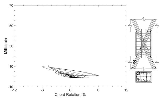
Figure 85 – Measured strain in diagonal bar of D80-1.5, strain gauge D3
