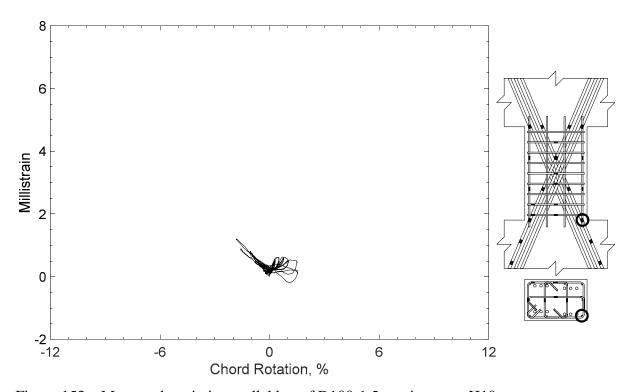
Figure 153 – Measured strain in parallel bar of D100-1.5, strain gauge H10
