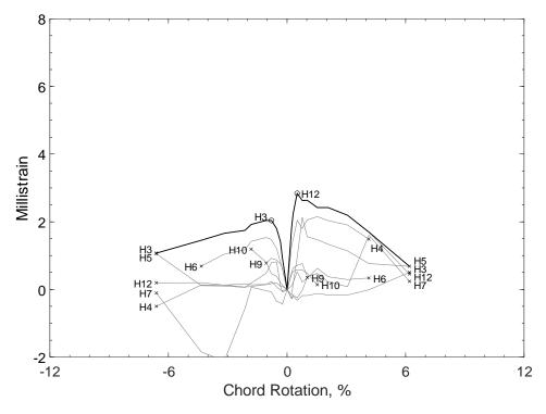
Figure 453 – Envelopes of measured strains in parallel bars of D100-1.5, H strain gauges
