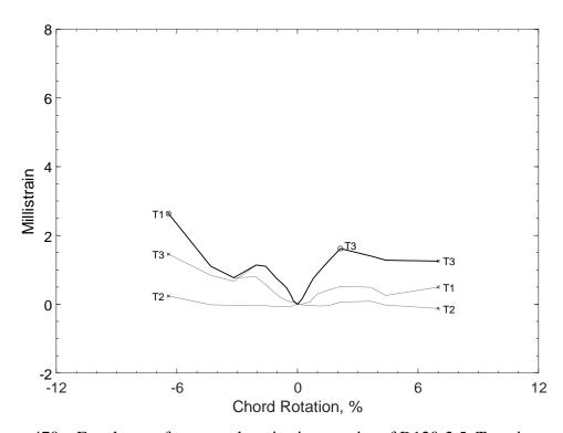
Figure 470 – Envelopes of measured strains in crossties of D120-2.5, T strain gauges
