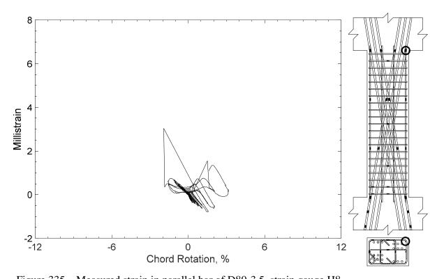
Figure 335 – Measured strain in parallel bar of D80-3.5, strain gauge H8
