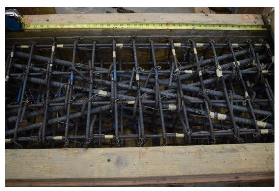
$Figure\ B.2-Coupling\ beam\ reinforcement,\ D120-2.5$
