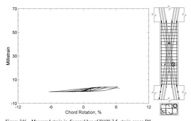
Figure 346 – Measured strain in diagonal bar of D100-3.5, strain gauge D8
