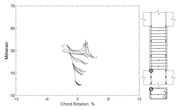
Figure 407 – Measured strain in parallel bar of P80-2.5, strain gauge P5
