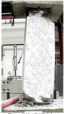
Figure C.82 – D100-3.5 at +10% chord rotation, first cycle
