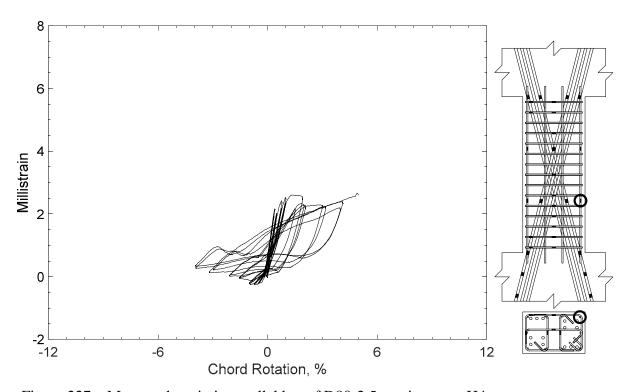
Figure 227 – Measured strain in parallel bar of D80-2.5, strain gauge H4
