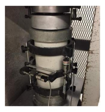
Figure 3.8: Series V Modulus Testing Setup
