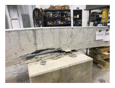
Figure 2.37: Flexural Failure (C4/60-60-5-100)
