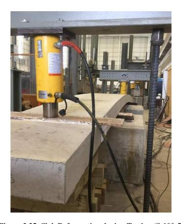
Figure 3.35: Slab Deformation during Testing (S-100-5)
