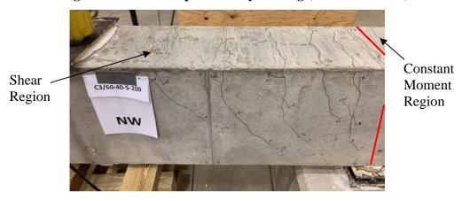
**Figure 4.48: Shear Span – Late Testing (C3/60-40-5-200)**
