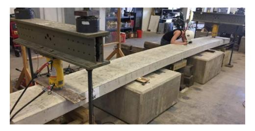
Figure 3.32: General Slab Test – Crack Mapping (S-80-5)
