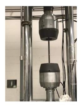
Figure 2.7: Testing of No. 8 Bars
