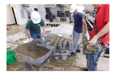
Figure 2.20: Making of Cylinders
