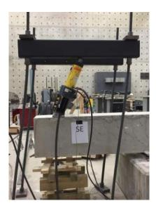
Figure 2.24: DYWIDAG Bars Yielding in Testing of U-80-5
