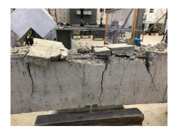
Figure 2.36: Typical Confined Specimen Failure (C3/60-40-5-100)
