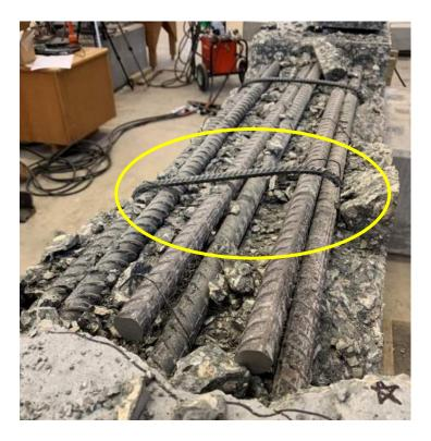
Figure 4.58: Ruptured Stirrup on Specimen C3/60/2-40-10-50
