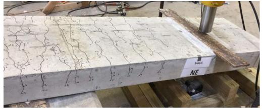
Figure 3.42: Post-Failure Shear Span Cracking (S-60-5)
