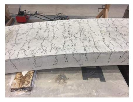
Figure 3.36: Typical Flexural Cracking – West Side and Tension Face (S-80-5)
