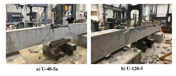
Figure 2.35: Typical Unconfined Specimen Failure
