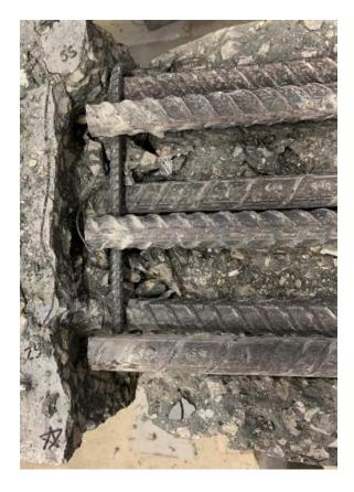
Figure 4.56: Bar Slip on Specimen C3/60/2-40-10-25
