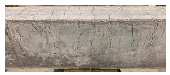
Figure 4.39: Typical Flexural Cracking within Unconfined Splice Region (U-60-10)
