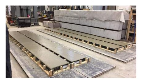
**Figure 3.18: Series V Casting Complete**
