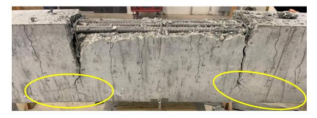
a) Full Splice at Failure
