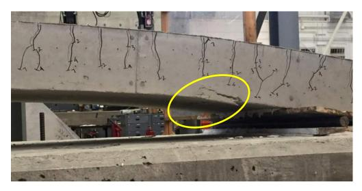
Figure 3.50: Initiation of S-80-5 Failure – East Elevation
