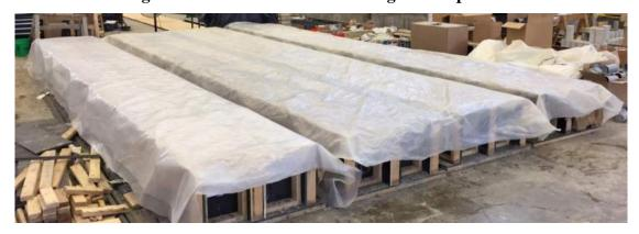
Figure 4.29: Series VI Moist Curing – Plastic Cover
