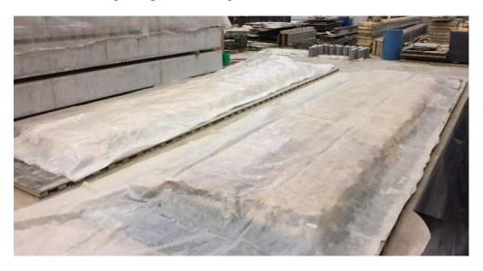
Figure 3.19: Series V Moist Curing
