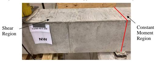
**Figure 4.47: Shear Span – Early Testing (C3/60-40-5-200)**
