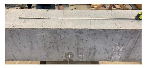
Figure 4.45: Transverse Flexural Cracking within Splice Region (C3/60/2-40-10-50)
