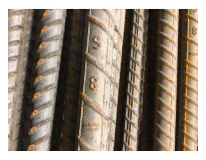
Figure 2.6: Bar Mark for Longitudinal Bars
