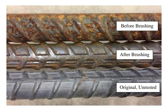
Figure 4.12: Comparison of Grade 100 Bar Surfaces
