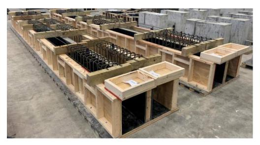
Figure 4.16: Series VII Cage Support Blocks
