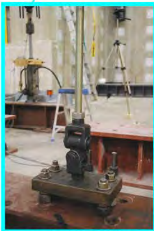
Universal joint at the support
