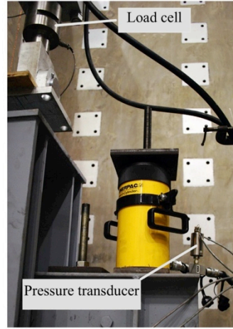
Measurement of concentric and eccentric loads
