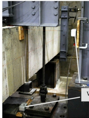
Measurement of vertical & horizontal displacements due to torque
