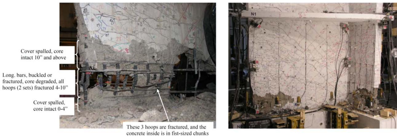
Figure 5: Flexural-compression failure of a T-shaped wall specimen subjected to bi-directional lateral loading and constant axial loading (Brueggen 2009). At the end of the test: (a) buckled longitudinal steel with crushed confined concrete removed and (b) wall damage.
