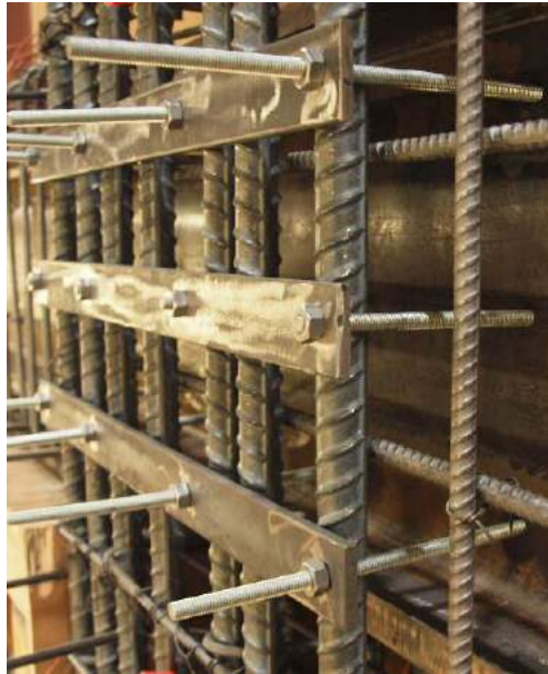
Figure 4.4: Close-Up of Embedment Detail
