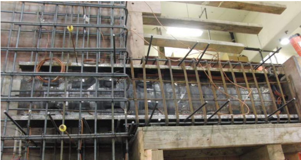
Figure 4.8: SRC4 Embedded Steel Section and Reinforcement
