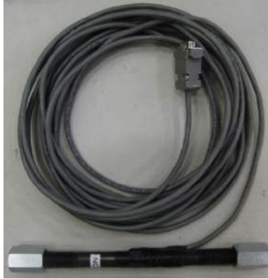
Figure 4.21: Load Cell Used to Determine Coupling Beam Axial Load
