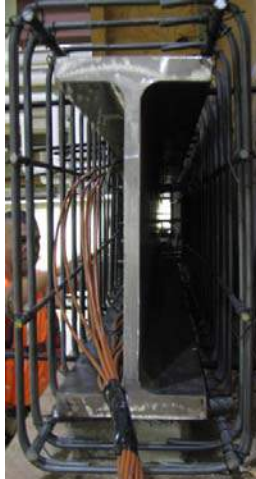
Figure 4.1: Typical Coupling Beam Cross-Section
