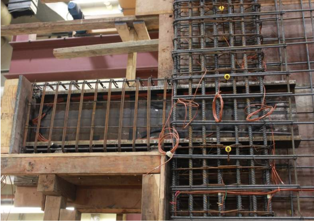
Figure 4.7: SRC3 Embedded Steel Section and Reinforcement
