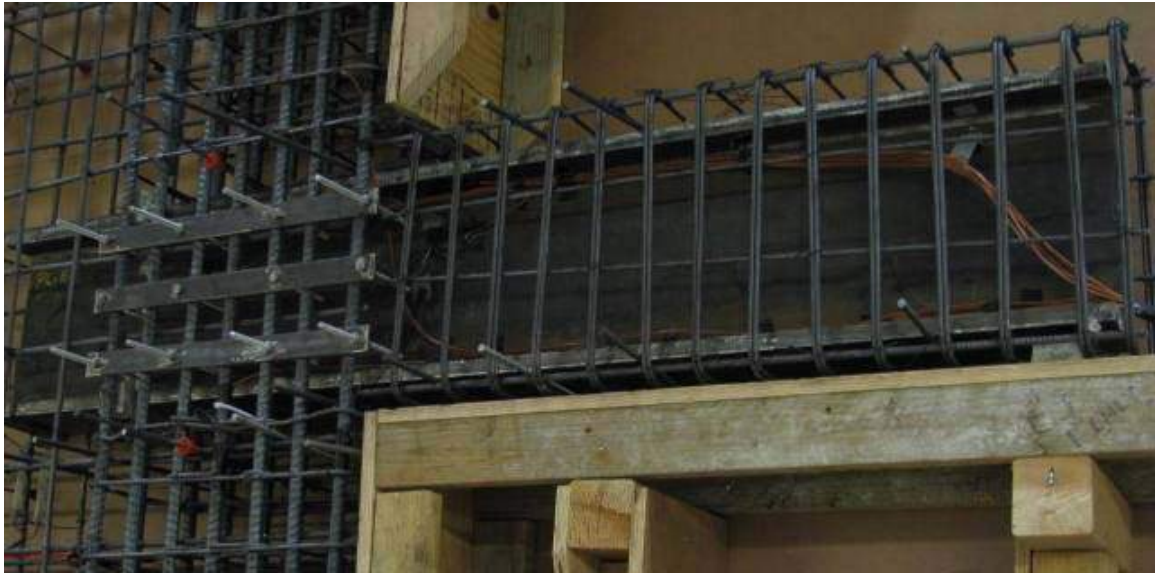
Figure 4.5: SRC1 Embedded Steel Section and Reinforcement
