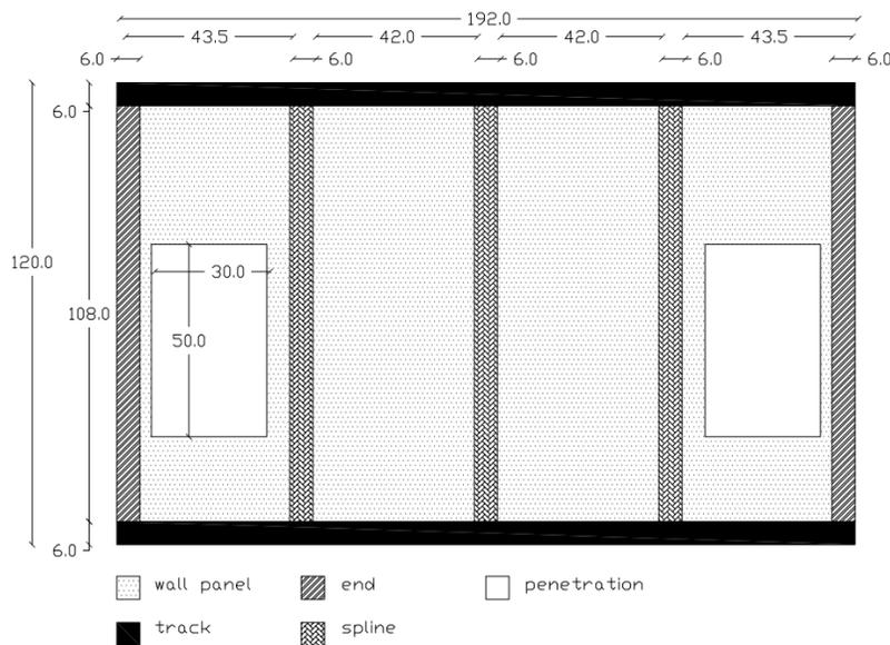
Figure 57 - Diagrammed Wall Assembly
