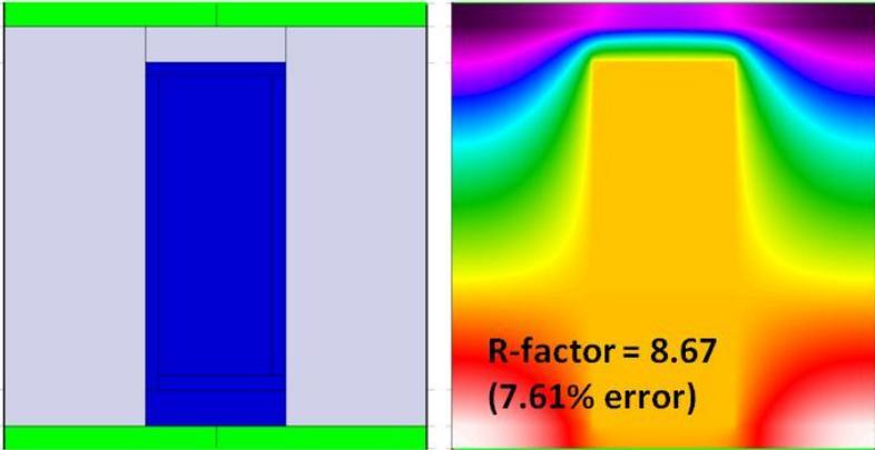
Figure 25 – Infrared Thermal Analysis of SIP with Offset Spline
