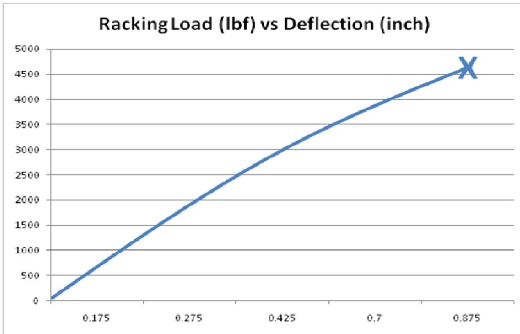
Figure 19 - Approximate Racking Loading of CSIPs
