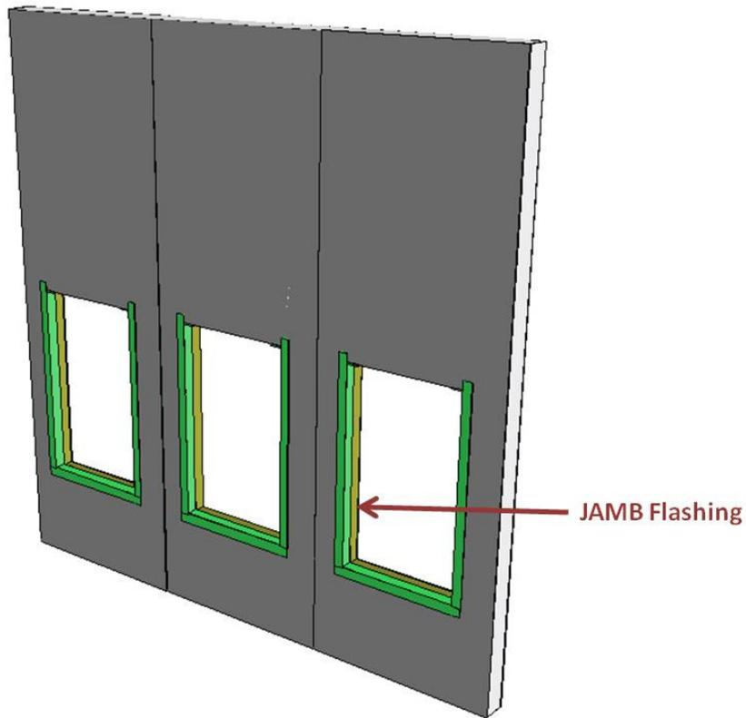
Design Considerations include: Jamb flashing material, Installation Specifications.
