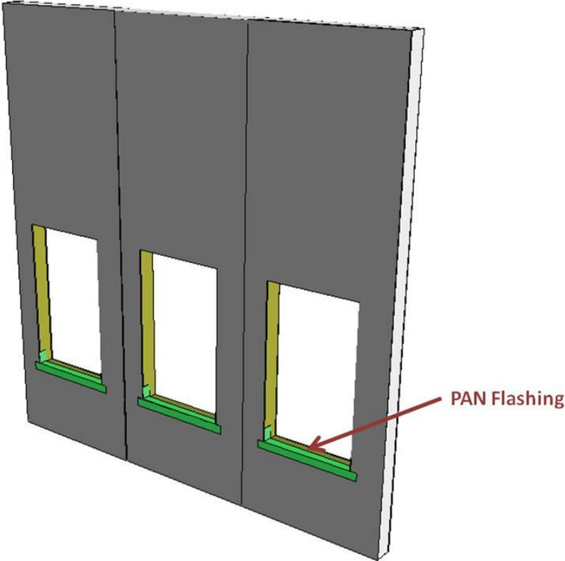
Design Considerations include: Pan flashing material, Installation Specifications.
