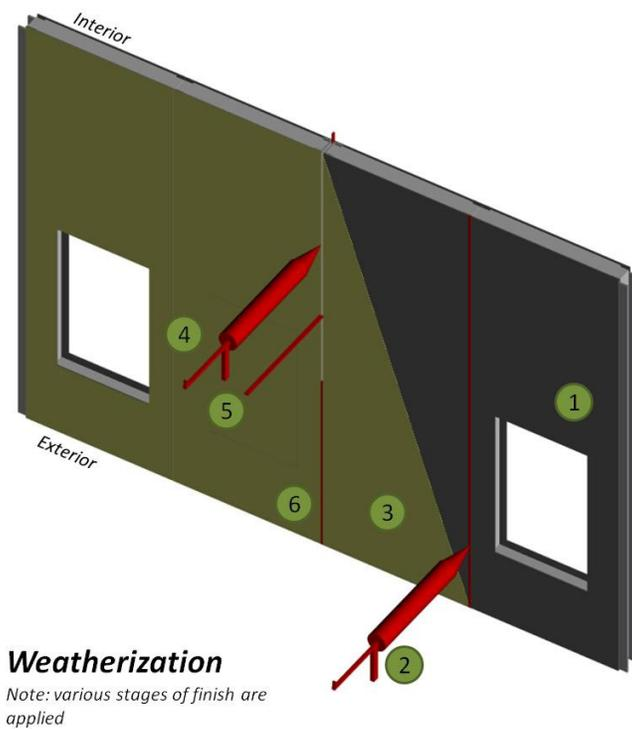
Figure 33 – Required Steps for Weatherizing CSIPs
