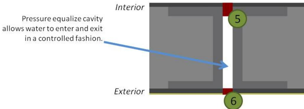
Figure 34 – Pressure Equalized Cavity
