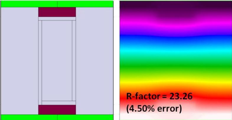
Figure 22 – Infrared Thermal Analysis Diagram of SIP with Surface Spline
