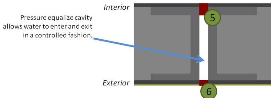
Figure 58 - Pressure Equalized Cavity
