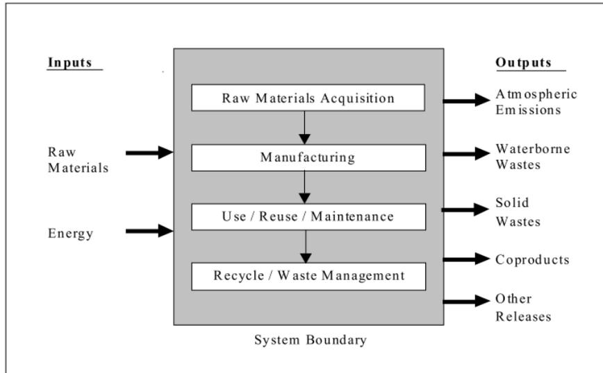
Figure 30 – Diagram of Life Cycle Stages <sup>44</sup>
