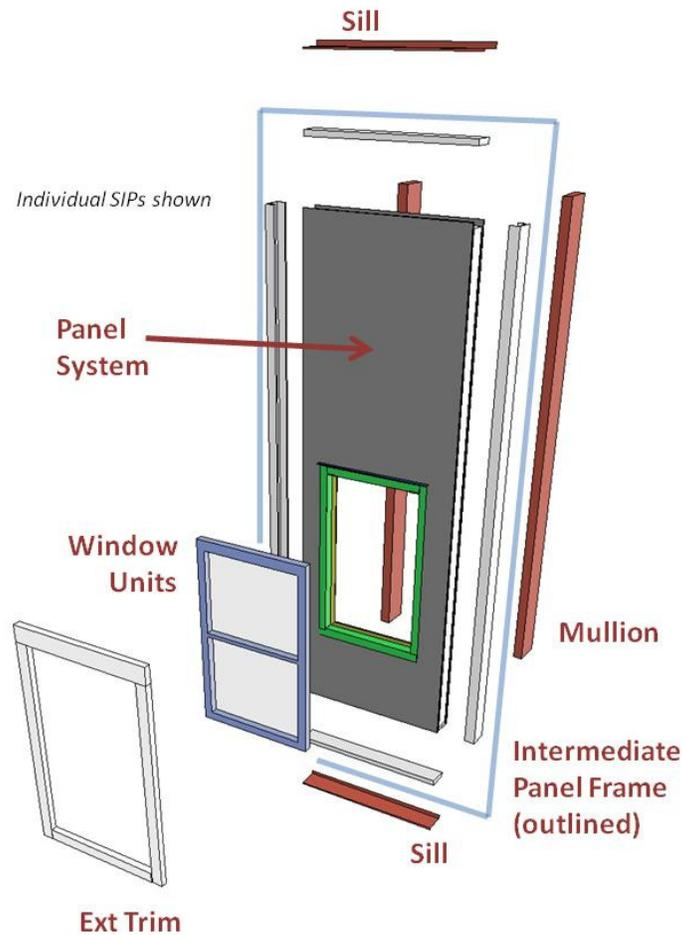
Figure 48 - Parts of the Unit Mullion System
