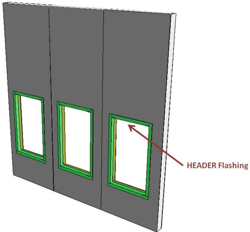
Design Considerations include: Header flashing material, Installation Specifications.
