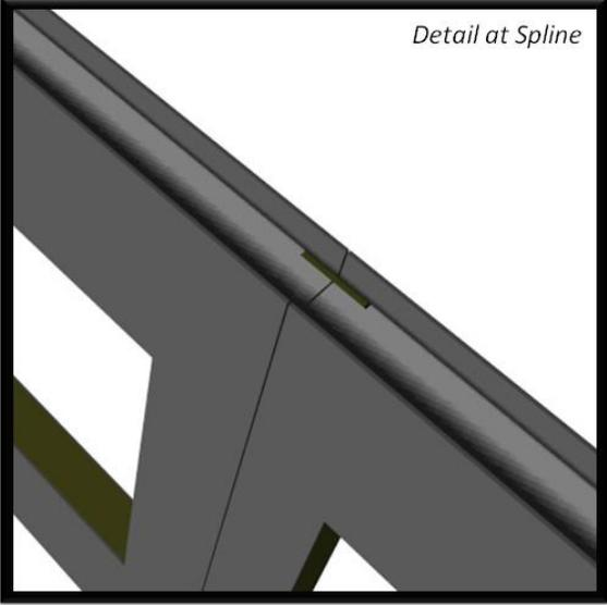
6 & 7. Installation of band plate and top plate: installed with 2x6 #3 or better. Plates must be tied together horizontally with and to the panel and must be tied together vertically.
