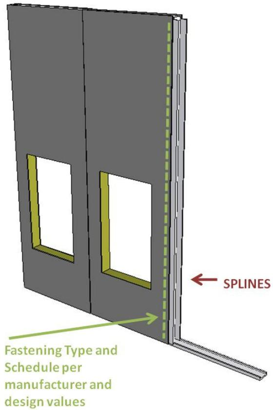
Design Considerations include: Panel Span, Panel Material, Measured Panel Performance, Panel conditions of use, Panel Thickness, Panel Design Values, Tested Spline materials, Tested Spline connections, Tested Spline limitations.
