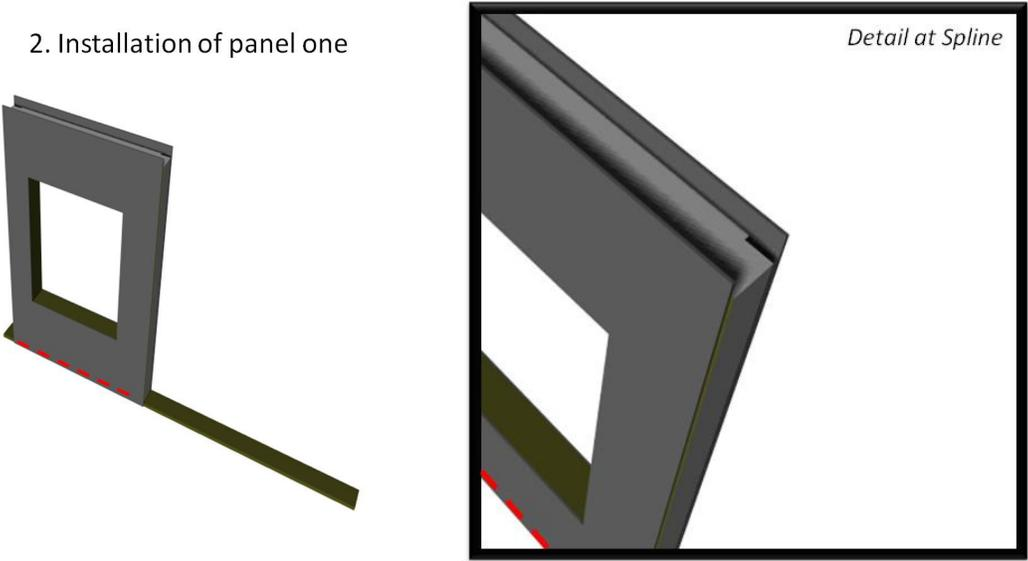
3. Installation of spline: Splines are comprised of 19/32 OSB or better splines, cut 5.5" wide to prevent telegraphing or "saw tothing" of panels. This detail recognizes the industry need to give generous spline widths and meet code minimums for fastening depth through the spline. More spline types are detailed later in this report.
