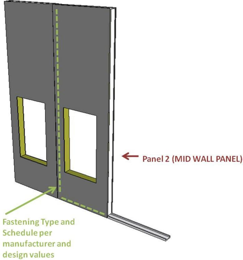
Design Considerations include: Panel Span, Panel Material, Measured Panel Performance, Panel conditions of use, Panel Thickness, Panel Design Values.
