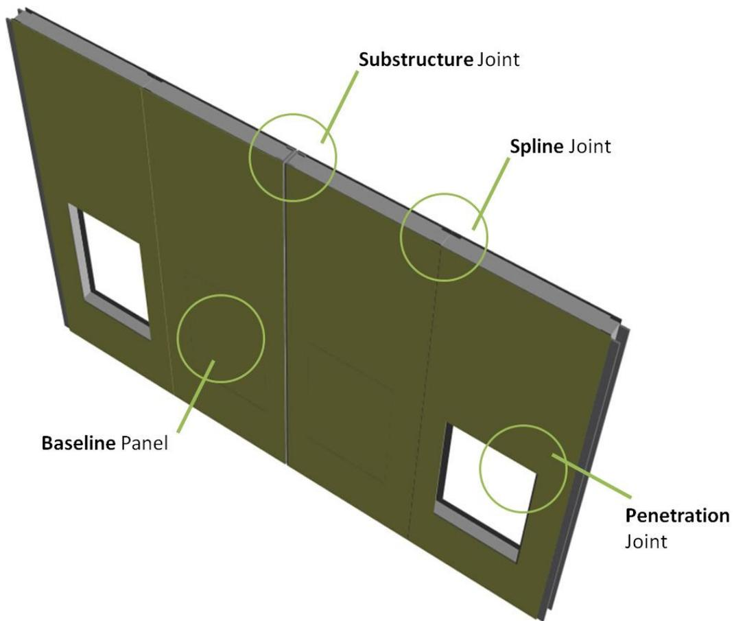
Figure 35 – Typical Joint Locations for Thermal Optimization
