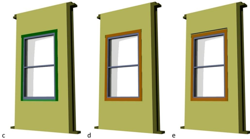
11. Installation of trim (a, b, c): Allow for positive drainage at all abutments and surface caulk all joints and other exposed areas. Follow the manufacturer's specifications.
