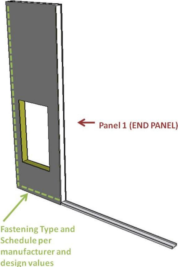
Design Considerations include: Panel Span, Panel Material, Measured Panel Performance, Panel conditions of use, Panel Thickness, Panel Design Values.
