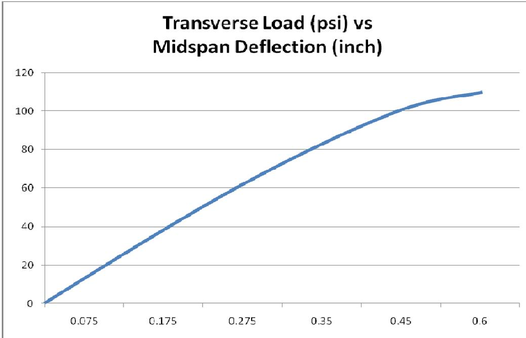
Figure 17 - Approximate Transverse Loading of CSIPs
