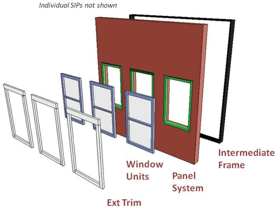
Figure 47 - Components of Unit System
