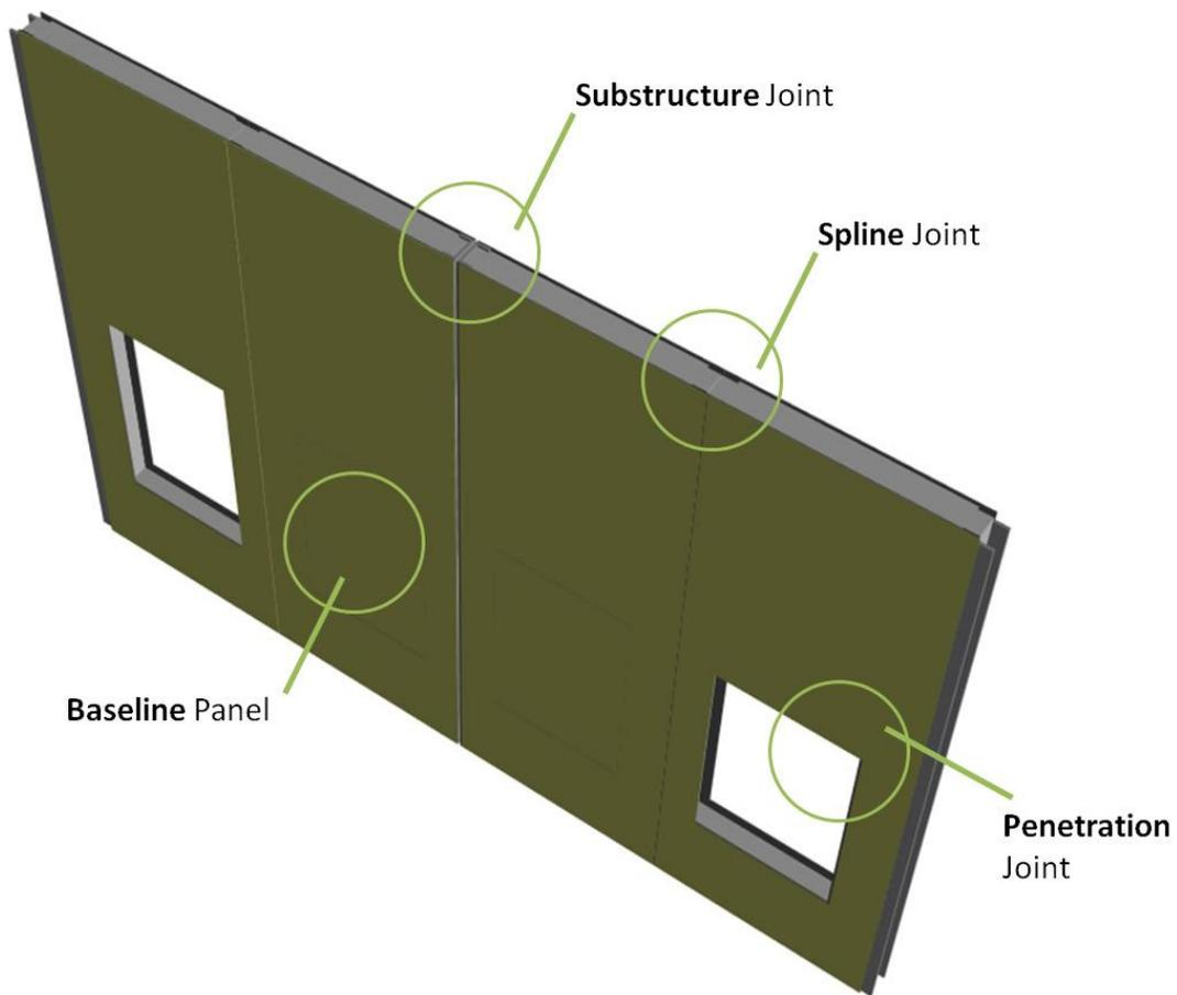
Figure 54 - Typical Joint Locations for Thermal Optimization
