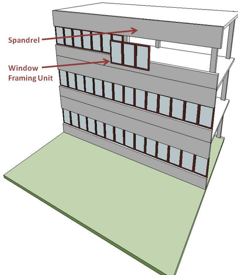
Figure 41 – Typical Building with Continuous Spandrel and Window Framing Units
