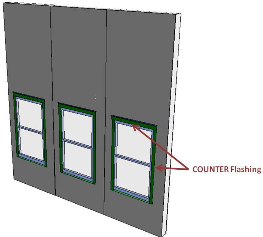
Design Considerations include: Counter-flashing material, Installation Specifications.
