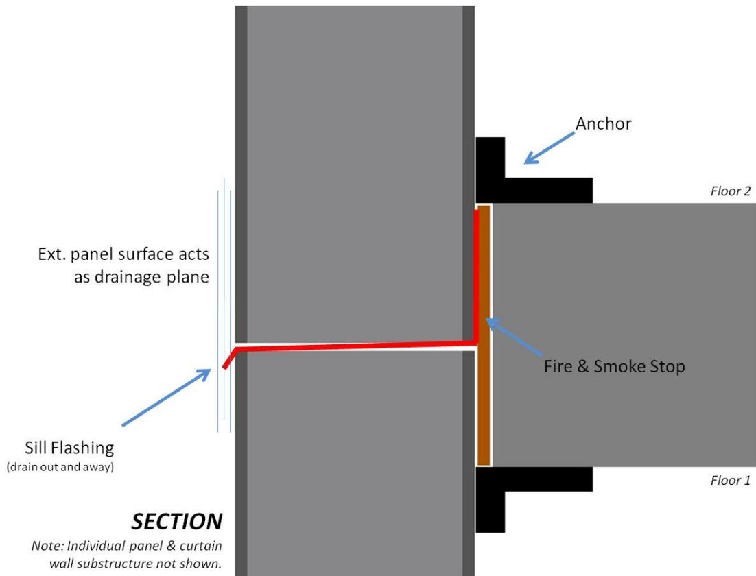
Figure 59 - Common Fire Stop Details
