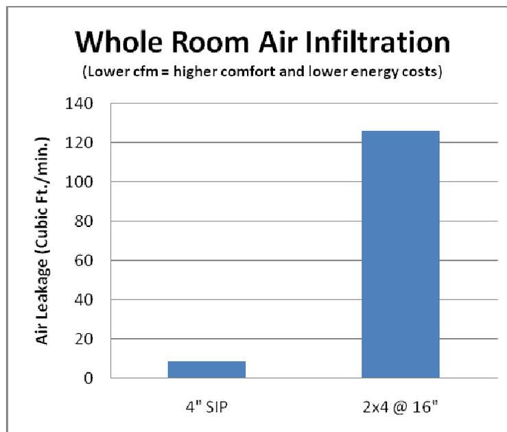
Figure 29 – Air Infiltration of SIPs Versus Wood Frame Construction<sup>39</sup>
