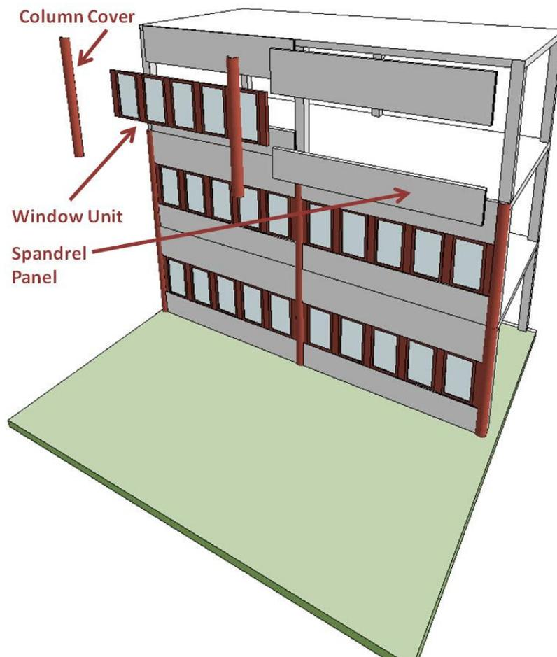
Figure 46 - Column-cover-spandrel System
