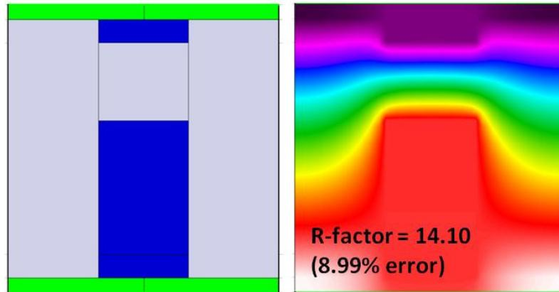
Figure 26 – Infrared Thermal Analysis of SIP with Guarded Offset Spline
