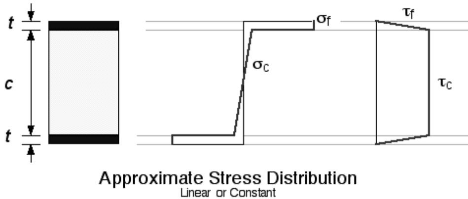
Figure 12 – Stress Distribution in a Composite Panel<sup>16</sup>
