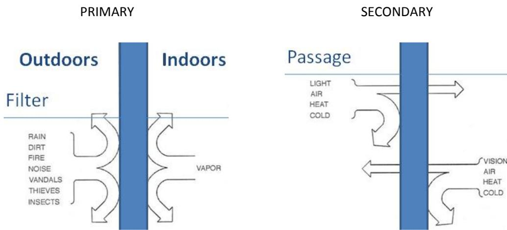
Figure 32 – Primary and Secondary Functions of the Building Envelope
