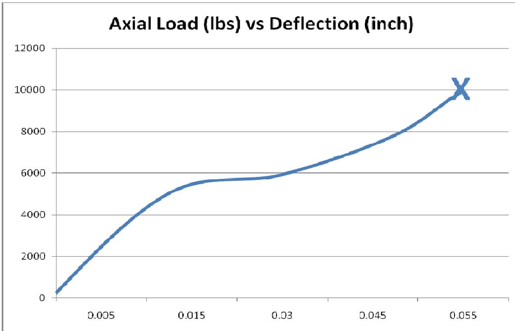
Figure 18 - Approximate Axial Loading of CSIPs
