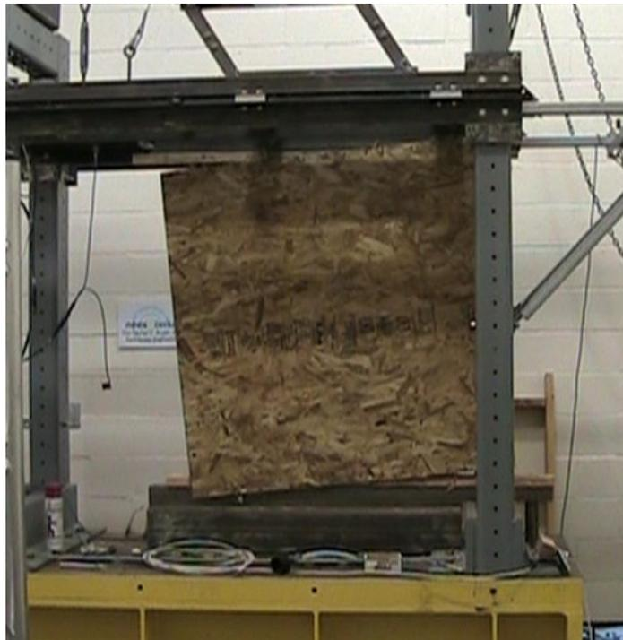
**Figure 20 – Small Scale Seismic Testing (OSB SIP Shown)**
