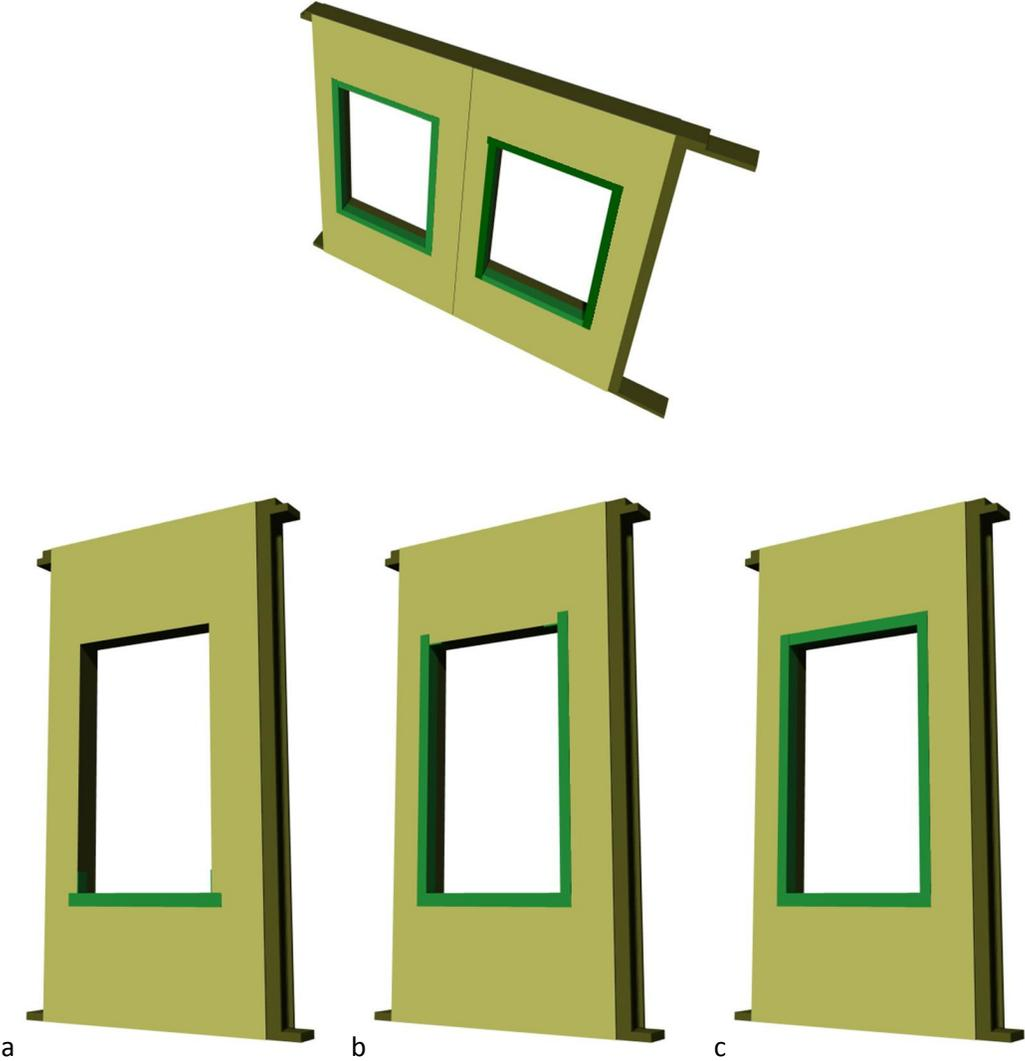
10a. Installation of window set: Only use windows with outer flange (i.e., nailing flange). Be sure to back caulk the window by applying sealant at window jambs and head. Use sealant at sill where required. Then set the window by installing the window level and plumb per the manufacturer's specifications.
