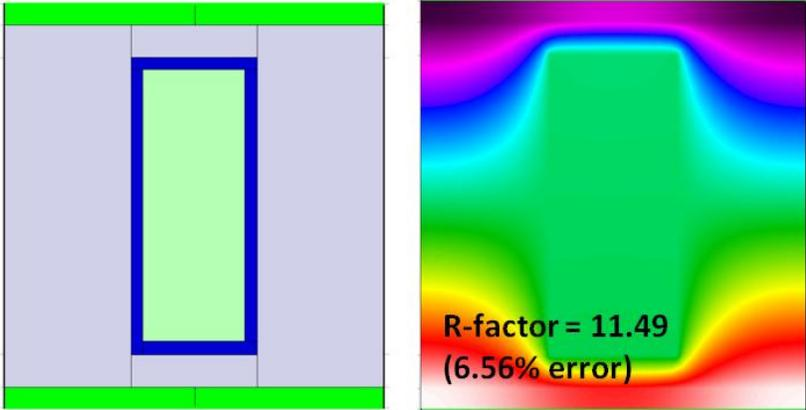
Figure 24 – Infrared Thermal Analysis Diagram of SIP with Guarded Spline
