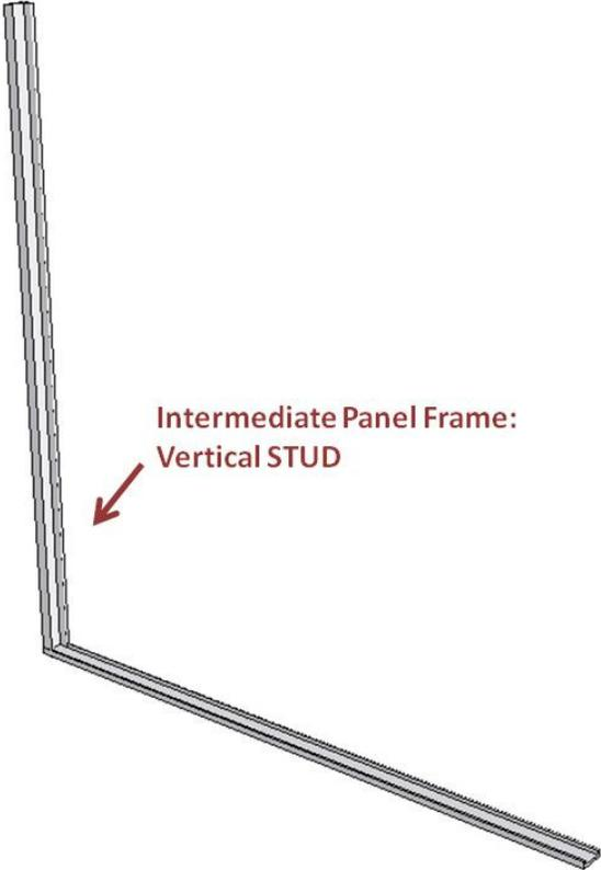
Design Considerations include: Stud Span, Stud Material, and Stud Thickness.
