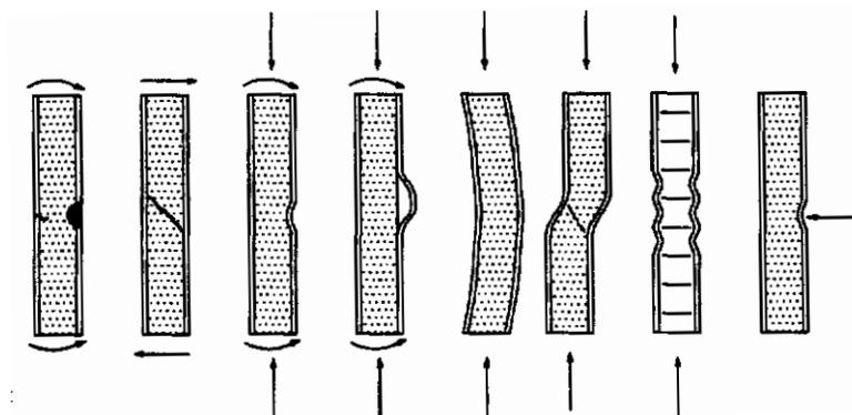
Figure 13 – Modes of Failure of Sandwich Panels
