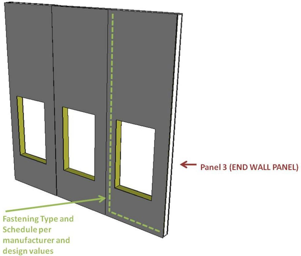
Design Considerations include: Panel Span, Panel Material, Measured Panel Performance, Panel conditions of use, Panel Thickness, Panel Design Values.
