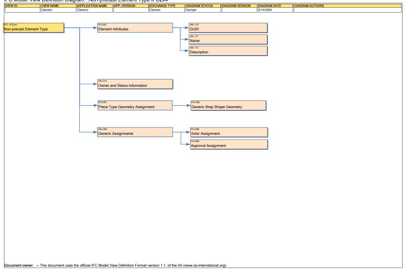
IFC Model View Definition Diagram : Non-precast Element Type IFC2x4
