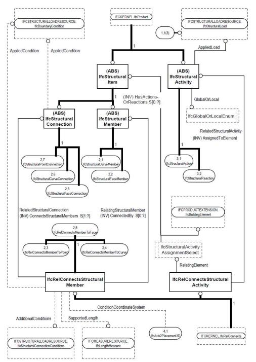
**FIGURE 2** EXPRESS G diagram showing the inheritance structure and main relationships and attributes defined in the structural analysis model.
