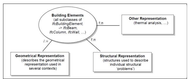
other domains using IFC, with Building Elements being the core concept.
