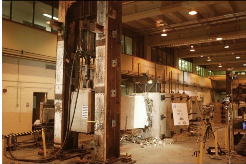
Figure 31 Beam 2: overview at the maximum negative displacement (drift ratio = -6.4%).
