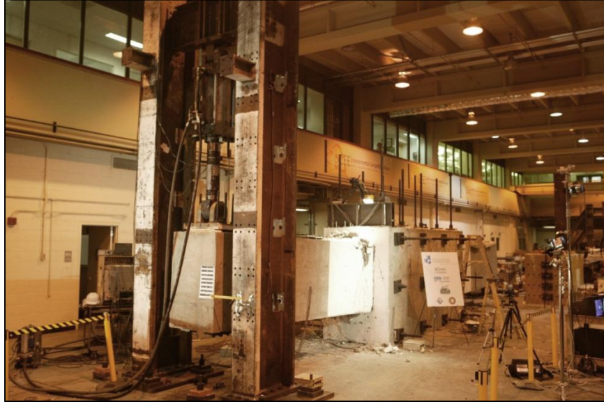
Figure 29 Beam 2: overview at the instant of top reinforcement buckling (first cycle with peak drift ratio = 3.9%, instantaneous drift ratio = -3.9%).
