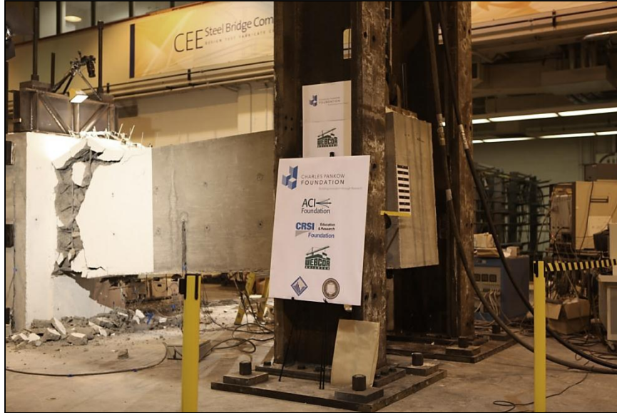
Figure 14 Beam 1: overview at the maximum negative displacement (cycle with peak drift ratio= -5.5%, instantaneous drift ratio= -5.5%).
