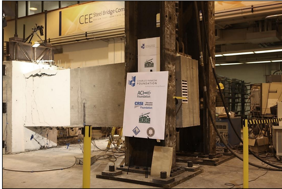
Figure 12 Beam 1: overview after the buckling of the top longitudinal bars (first cycle with peak drift ratio = 2.7%, instantaneous drift ratio = -2.7%).
