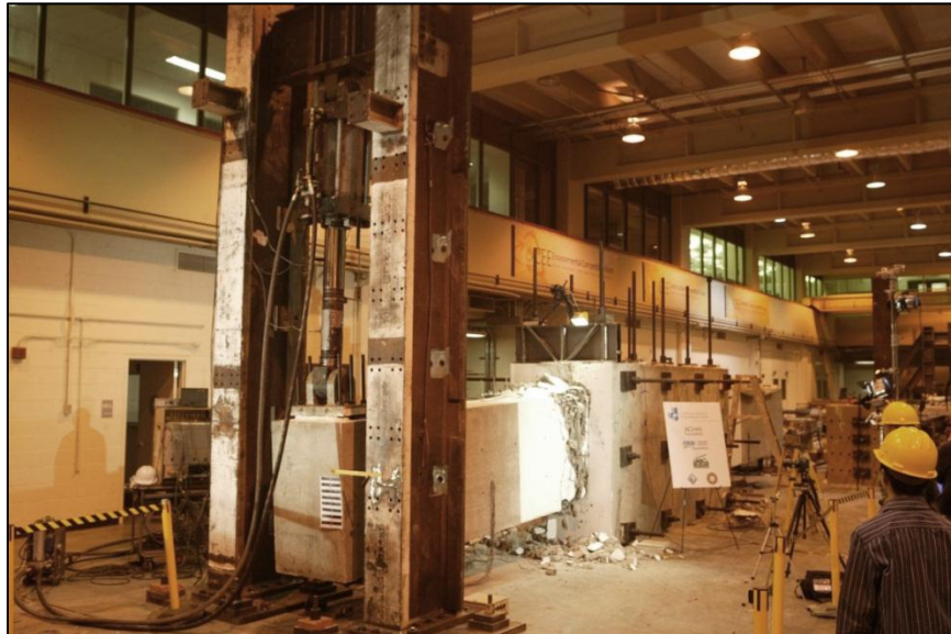
Figure 30 Beam 2: overview at the maximum positive displacement (drift ratio = 5.8%).
