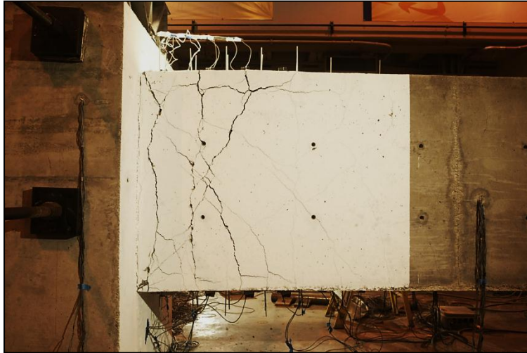
Figure 8 Beam 1: damage state at the beginning of cycle in which buckling occurred (first cycle with peak drift ratio = 2.7%, instantaneous drift ratio = -0.9%).
