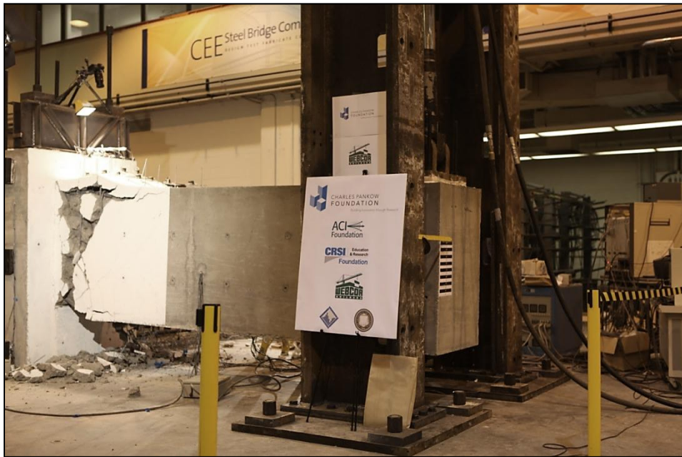
Figure 13 Beam 1: overview at the maximum positive displacement (cycle with peak drift ratio = 5.5%, instantaneous drift ratio = 5.5%).
