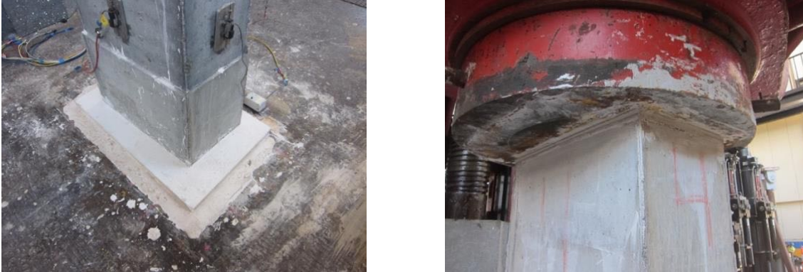
Figure 2.9 Bottom and top hydrostone layers
