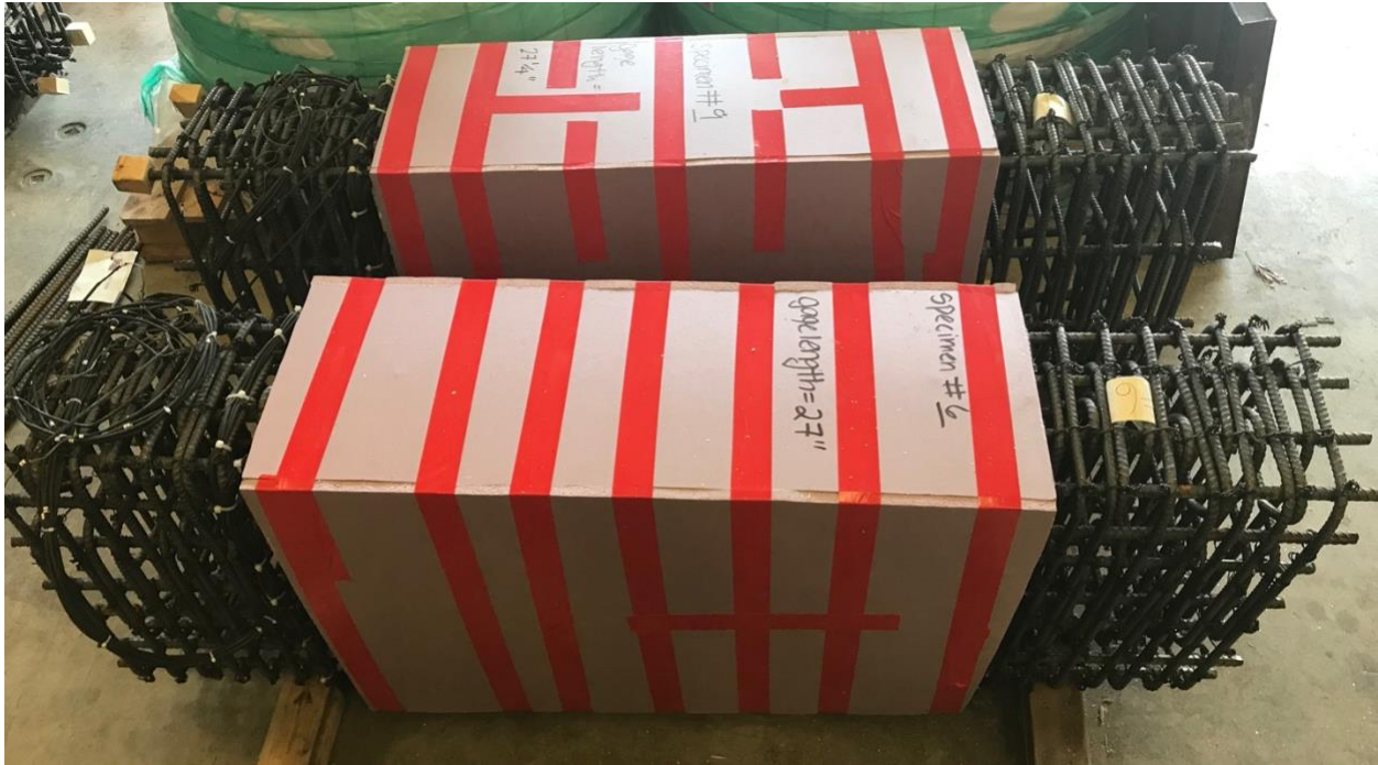
Figure 2.5 Reinforcement cages wrapped in insulation foam boards
