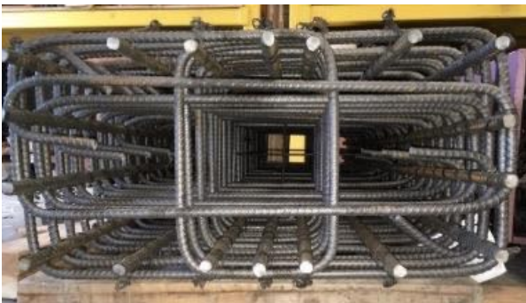
(c) Cross section of rectangular configuration 1 CWT specimen
