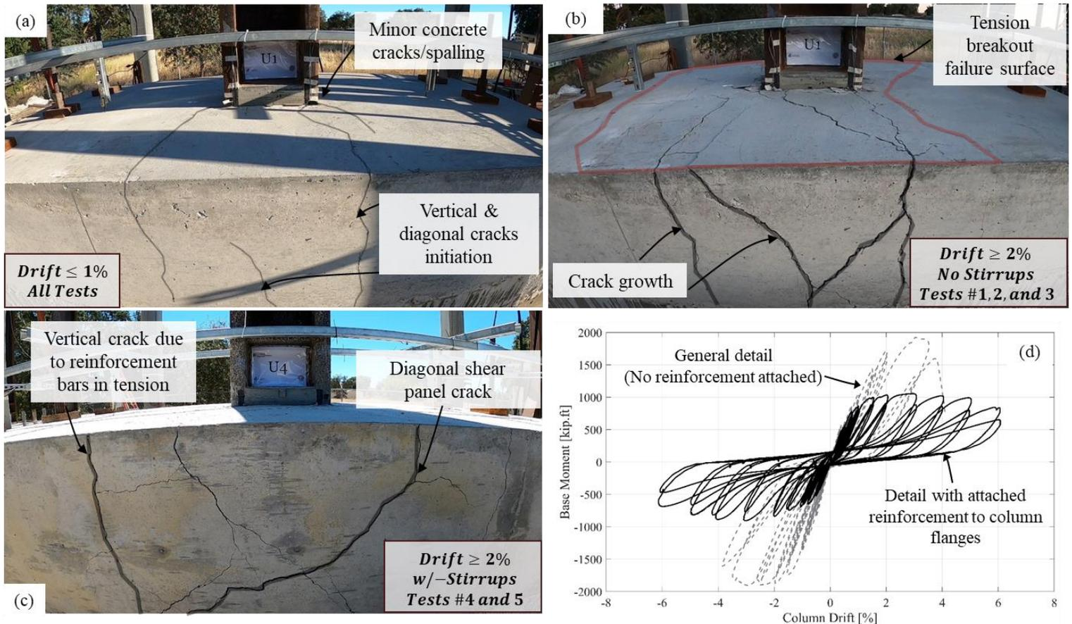
**Figure 4.9** – Typical damage progression and behavioral insights: (a) below 1% drift for all tests; (b) failure mode for specimens with no stirrups (Tests #1, 2, and 3); (c) failure mode for specimens with stirrups (Tests #4 and 5); (d) moment-drift curve showing the effect of additional horizontal reinforcement as compared to a generic detail from Grilli et al. (2017)
