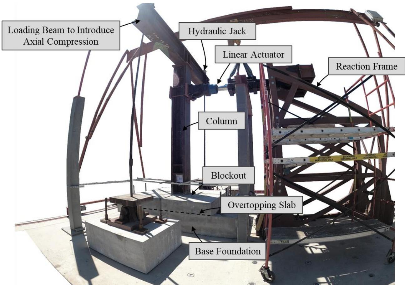
**Figure 3.4** – Wide angle view of test setup
