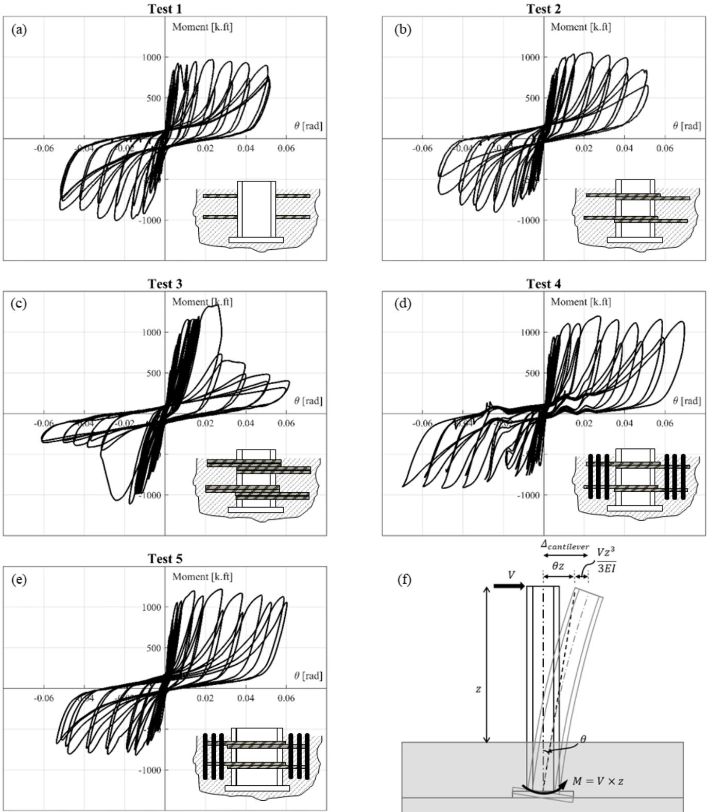
**Figure 4.8** – Moment-rotation plots for all tests, and a schematic illustration of plotted quantities
