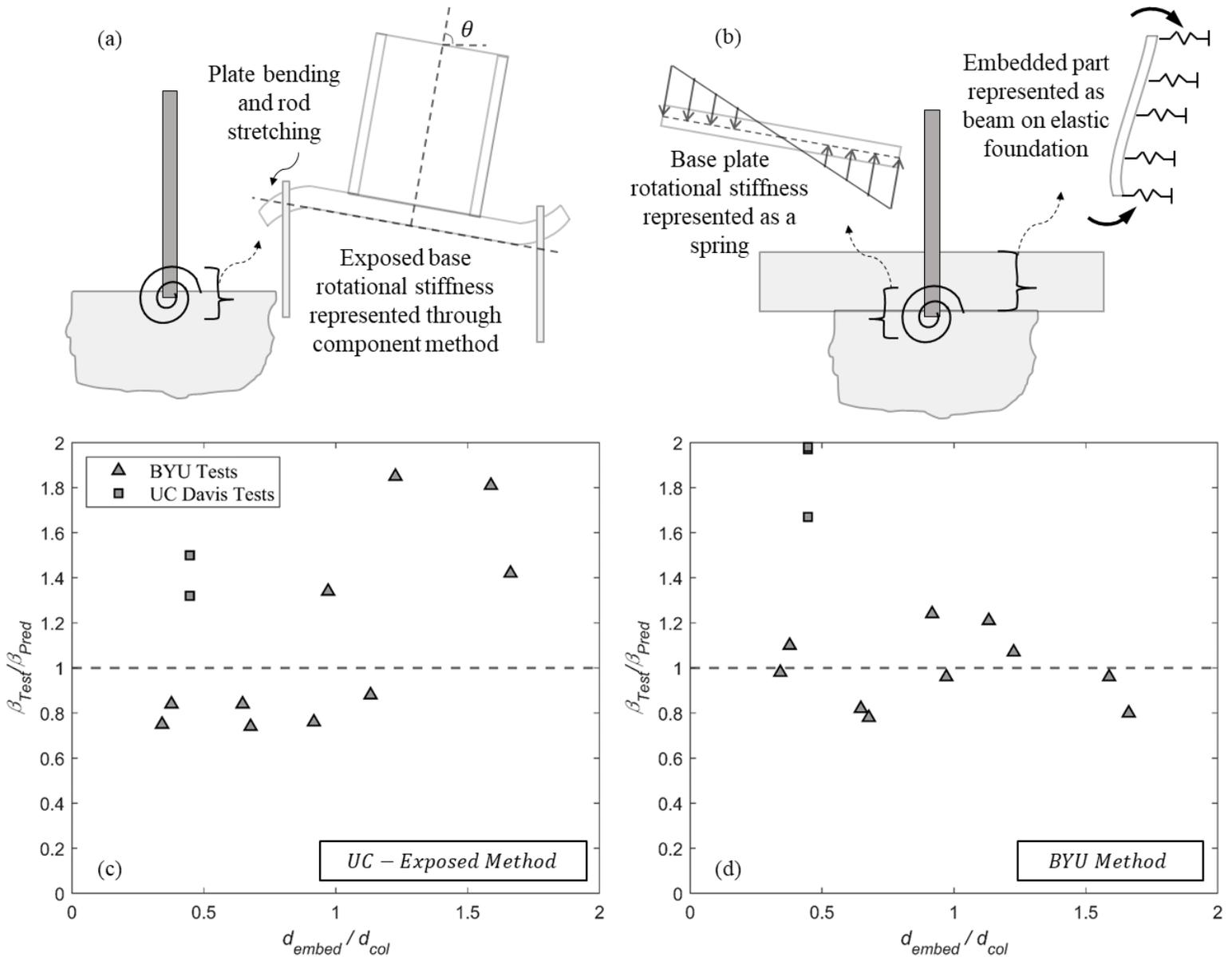
**Figure 3.11** – Key elements of stiffness method proposed by (a) UC Method - Kanvinde et al. (2012) and (b) BYU Method - Richards et al. (2018); (c-d) Test-predicted ratios for rotational stiffness from both methods.
