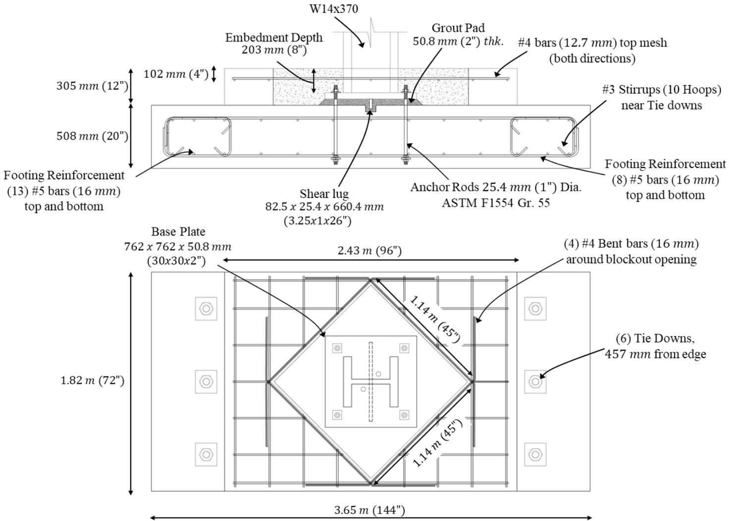
**Figure 3.5** – Schematic illustration of experimental specimens detailing
