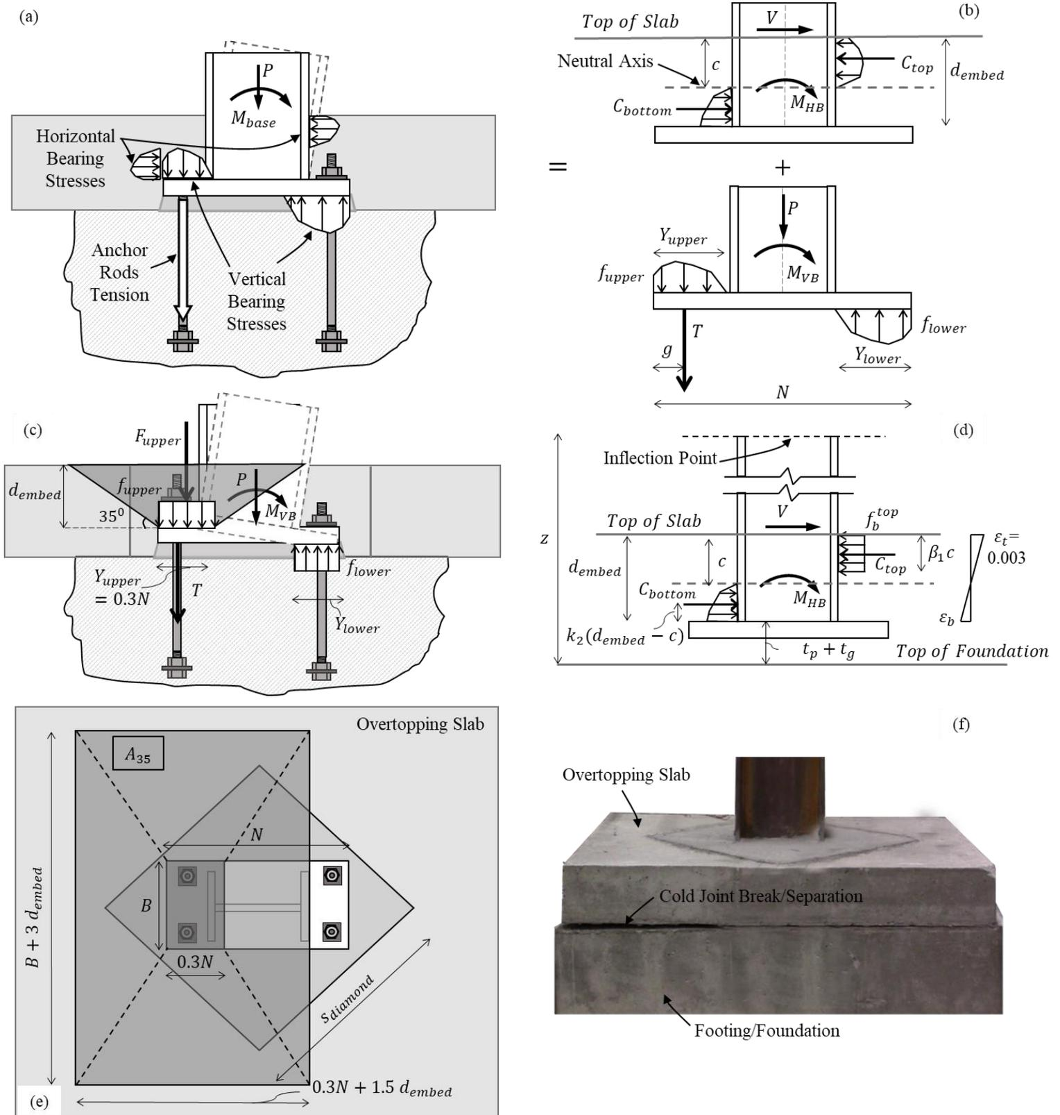
**Figure 3.10** – Mechanisms and model for strength characterization – Method 2 (a) overall mechanism; (b) moment resisted due to horizontal forces and due to vertical forces; (c) elevation view of concrete breakout cone and vertical resistance mechanism model; (d) horizontal resistance mechanism model (modified Mattock and Gaafar 1981); (e) projected area of breakout cone failure  $A_{35}$ ; (f) observed failure mode in some of BYU experiments (slab separation).
