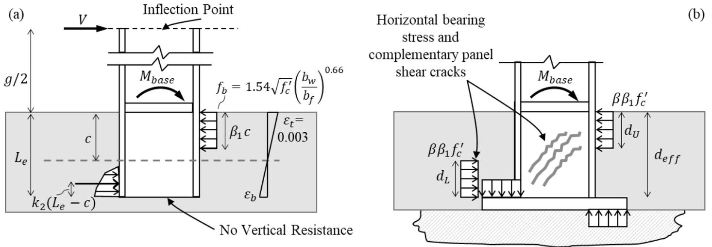
**Figure 4.4** – Strength model assumptions from (a) the AISC Seismic Design Manual approach (AISC 2018), and (b) Grilli and Kanvinde (2017) model
