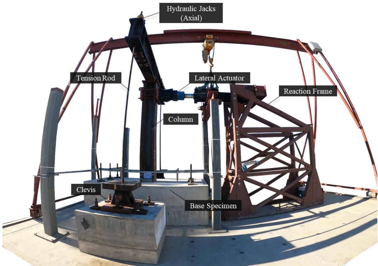
**Figure 4.5** – Wide angle view of test setup
