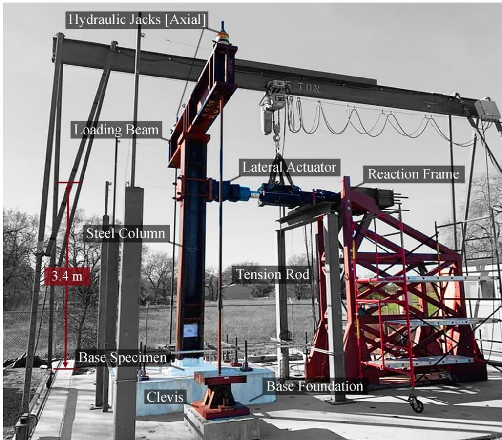
**Figure 2.3** – Experimental test setup.
