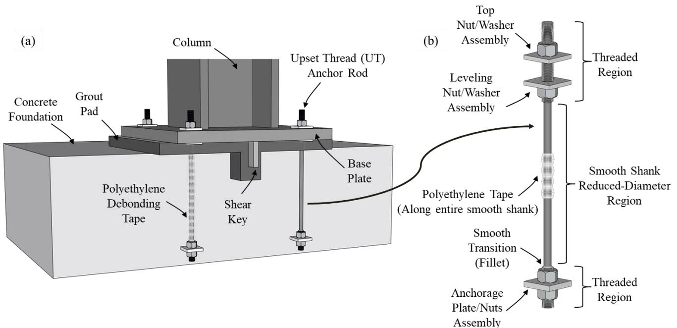
**Figure 2.2** – (a) Exposed Base Plate Connection with Upset Thread (UT) anchor rods (Isometric section view); (b) Upset Thread (UT) anchor rod detail.
