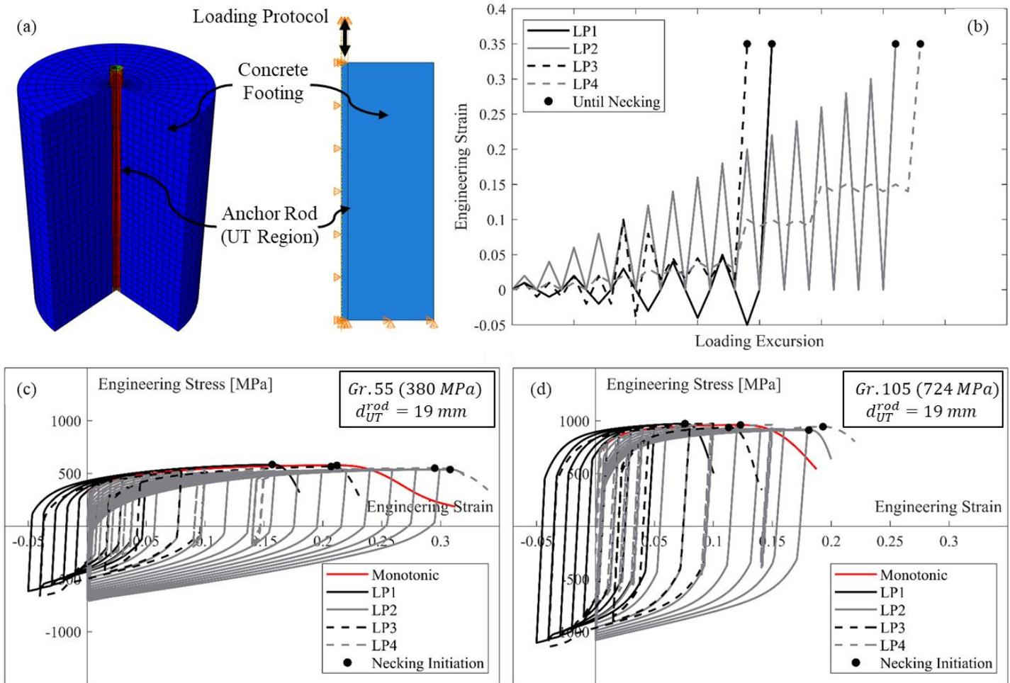
**Figure 2.16** – CFE simulations for necking damage measure validation: (a) CFE model for anchor rod with surrounding concrete; (b) Loading protocols under investigation; (c) stress-strain curves for rods of same diameter size (19 mm), subjected to monotonic and cyclic loading protocols, for Grade 55; and (d) Grade 105
