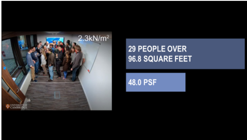
327 Figure 4. Live Load with People Pushed into About 100 square feet.
