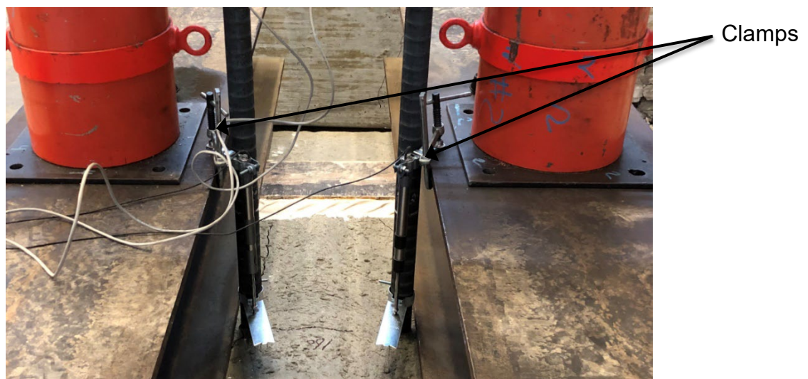
Figure 2.15 LVDTs clamped to the top flange of the spreader beams
