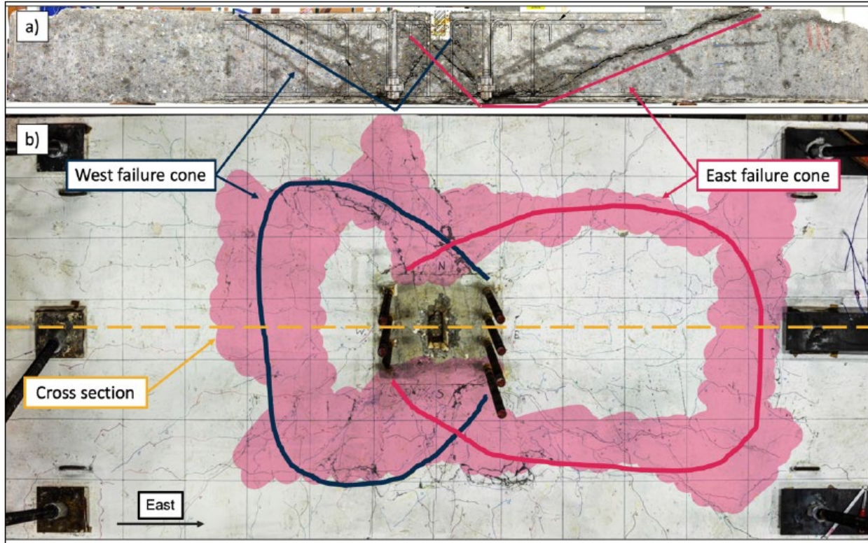
Figure 1.31 Cross section and plan view highlighting crack patterns and breakout cone geometry for Specimen M02 (Worsfold et al. 2022)
