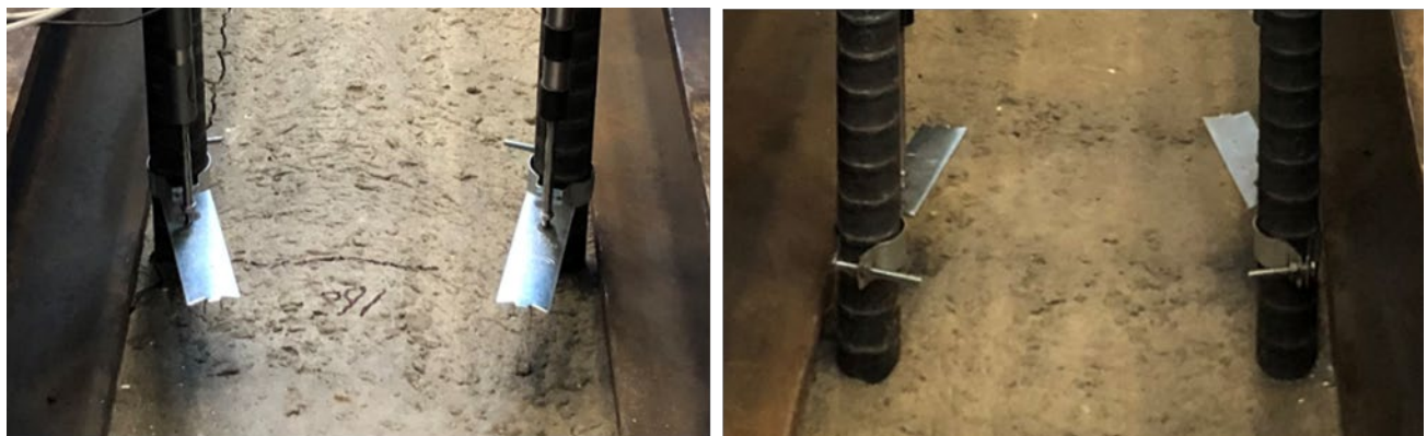
Figure 2.16 LVDT plates attached to test bars
