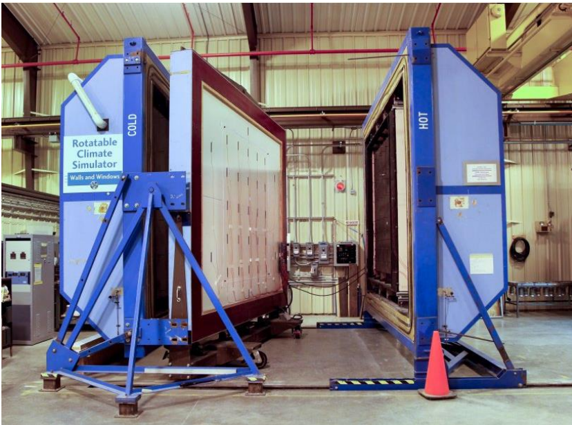
Physical thermal “hot box” testing Oak Ridge National Laboratory
