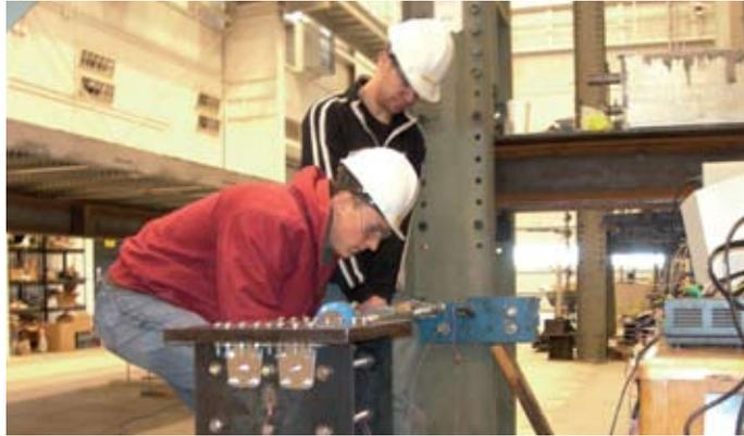
Construction of loading frame assembly in preparation to test the hybrid precast wall system design for seismic zones at the University of Notre Dame
