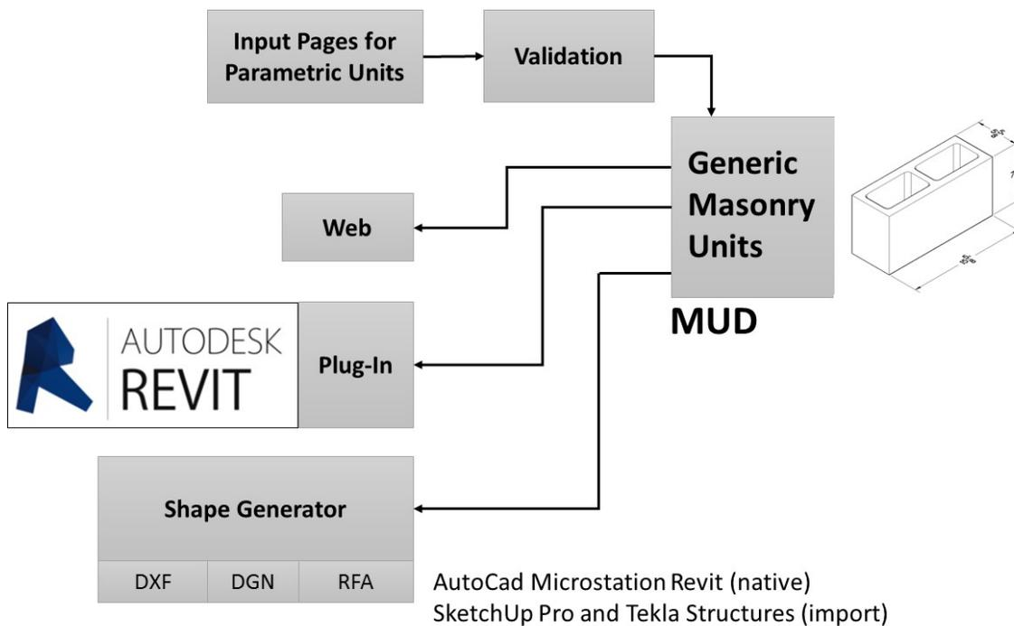
**Figure 1 - Elements and Organization of the Masonry Unit Database.**
