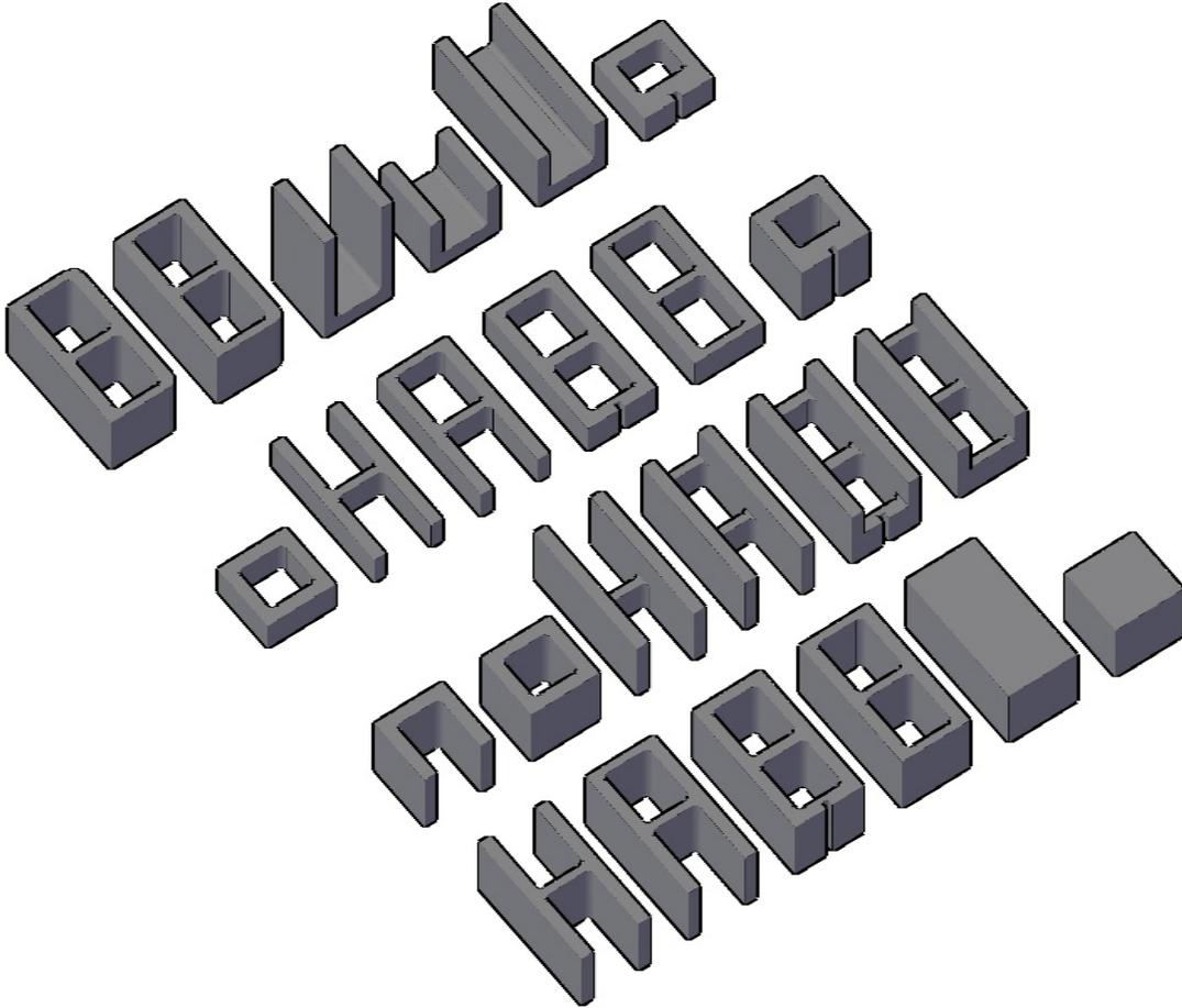
**Figure 2** - 8 inch concrete masonry units identified by NCMA for inclusion in the MUD.
