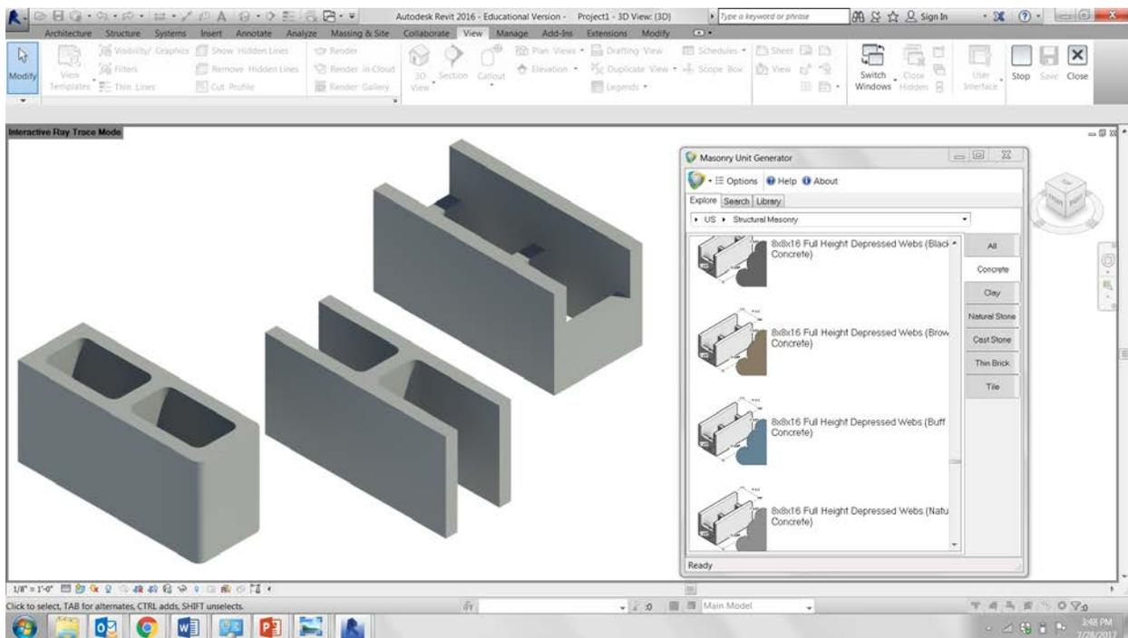
**Figure 5** - Access to the MUD using the Revit Plug-In.
