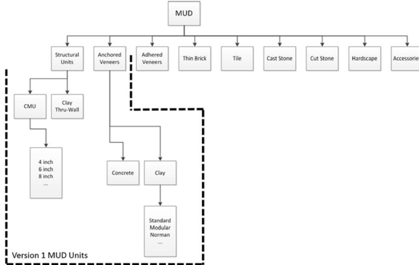
Figure 4 - Organization of Masonry Units in the MUD.
