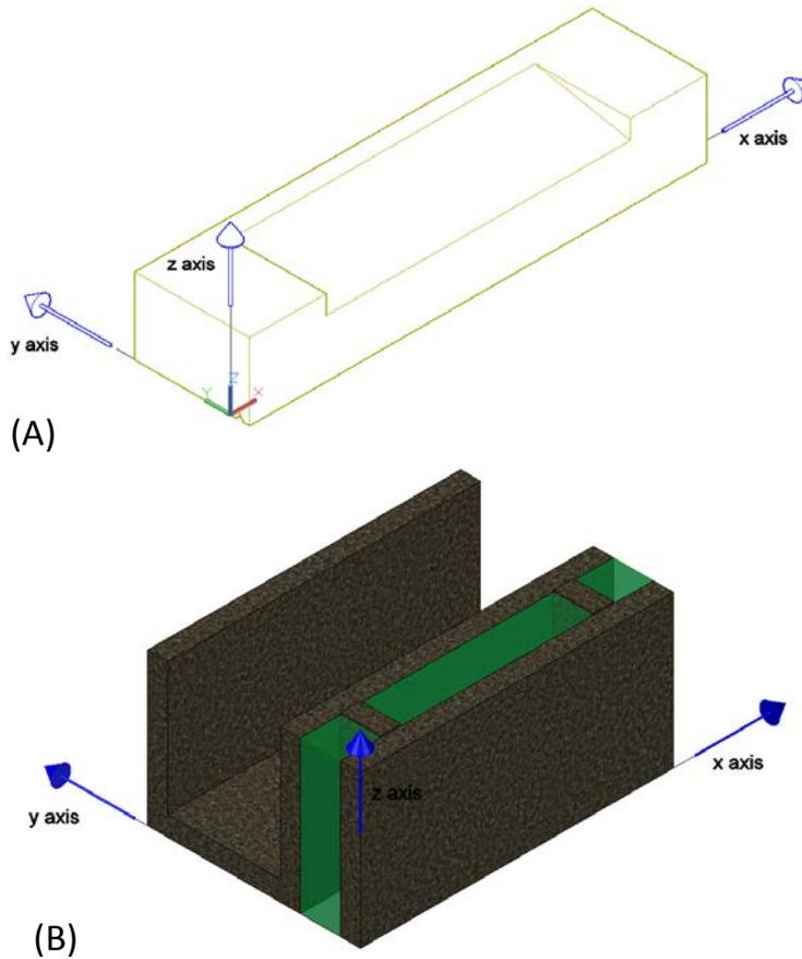
**Figure 6** - Examples of Custom Masonry Units: (A) Cast stone lug sill and (B) CMU with integral insulation.
